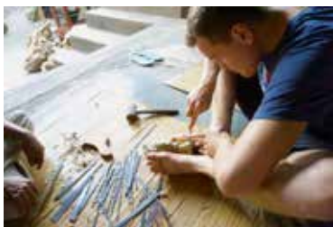
Carving Balinese style - notice the chisels have no handles
