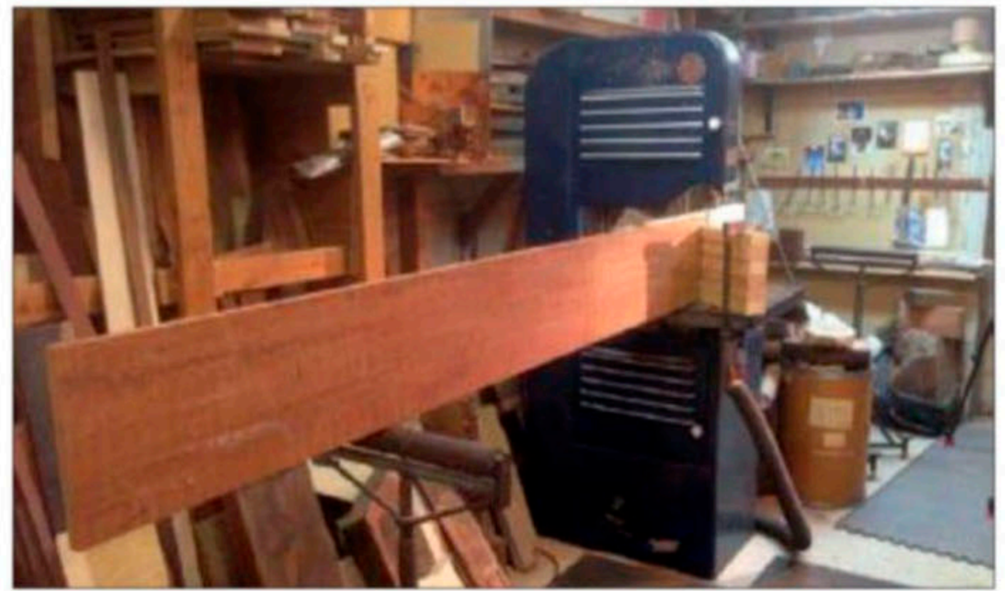
A board of rare Quilted Mahogany is positioned on David's 20" bandsaw. The board is 7' 8" long by 11 \frac{1}{2} " wide by \frac{15}{16} " thick and will be resawn into thick veneers of \frac{3}{32} ". Roller stands support the board on the infeed and outfeed.
