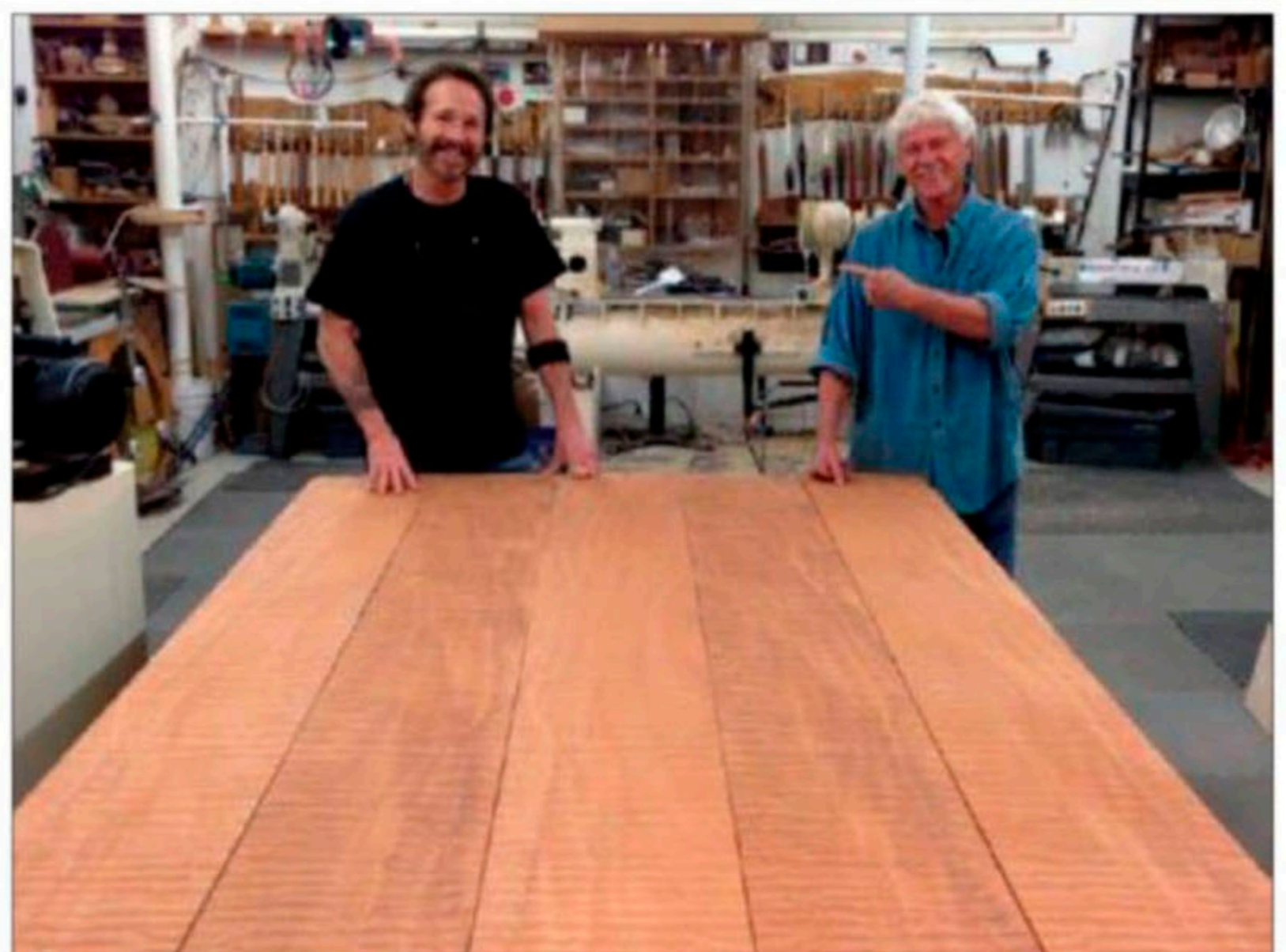
David got five \frac{3}{32} " thick slices from that board—the final slice is on the right. The remainder of the board (left) was \frac{1}{4} " thick, which was later resawn into two \frac{1}{32} " veneers.
