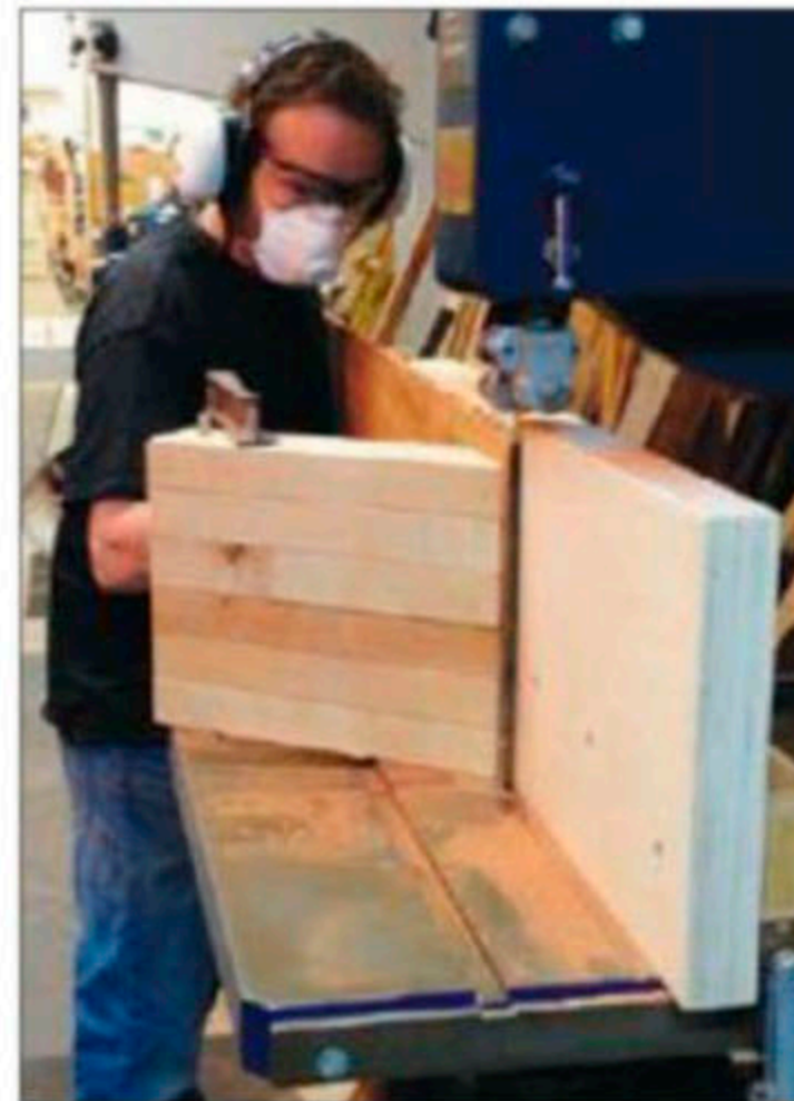
David got five \frac{3}{32} " thick slices from that board—the final slice is on the right. The remainder of the board (left) was \frac{1}{4} " thick, which was later resawn into two \frac{1}{32} " veneers.
