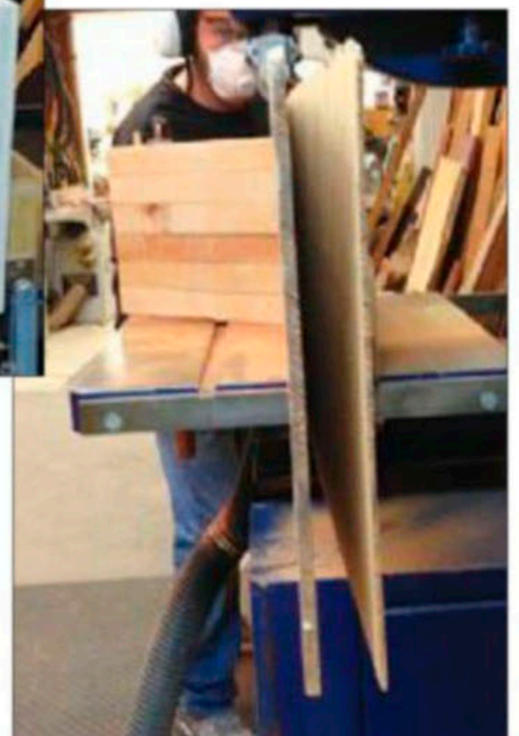
David got five \frac{3}{32} " thick slices from that board—the final slice is on the right. The remainder of the board (left) was \frac{1}{4} " thick, which was later resawn into two \frac{1}{32} " veneers.
