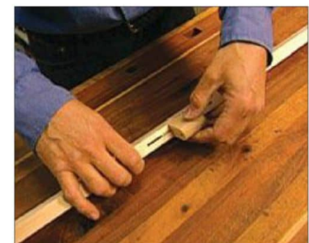
FIGURE 4 A slot is cut on each side of the notch with an hand-held router with a slot/kerf cutter bit.
