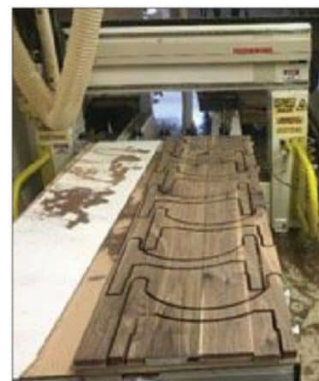
The laminates of the slide were cut on a CNC machine.
