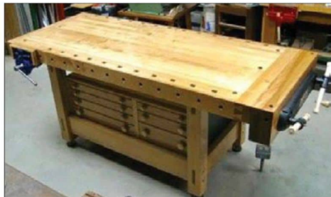
Workbench using a Bally Block countertop in the center
