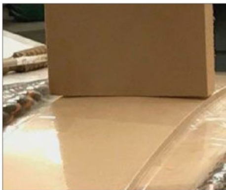
The good news is that by persevering, I eventually experienced success, which I tested by placing a straight edge on top of the bag with test pieces under pressure.
