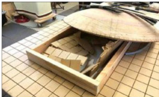
What remains of the imploded platen from the force of the vacuum press.
