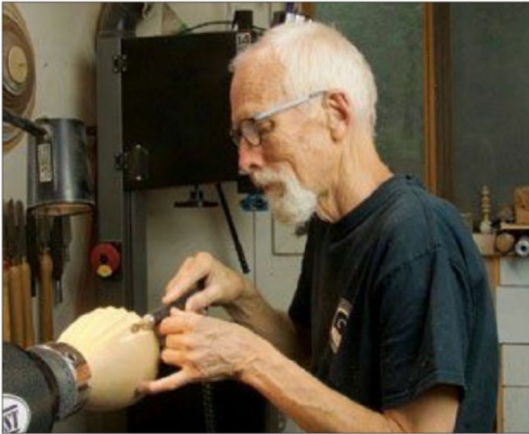
Jim Piper carves flutes in a piece using a rotary chisel.
