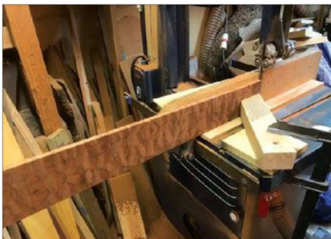
My bandsaw set up, with a featherboard to hold the stock firmly against the fence.
