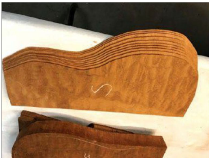
The guitar back blanks were then very carefully sliced into 10 pieces, approximately \frac{1}{8} " thick. This was a great yield, considering the boards were approximately 1\frac{7}{8} " thick originally. Keep in mind that I used a thin kerf blade that only removes a \frac{1}{32} " and then drum sanding removes another \frac{1}{32} ". My light passes on the jointer removed about \frac{1}{64} " at a time.
