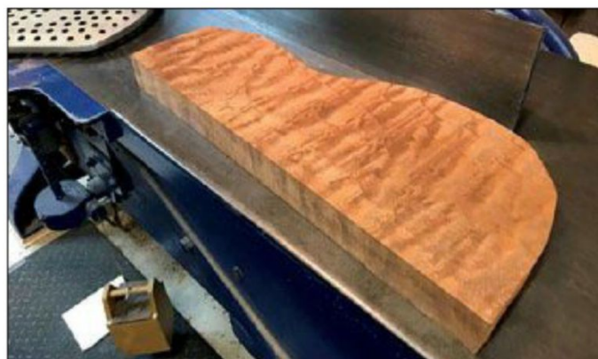
Each guitar back blank was jointed flat on the face, which is 8\frac{1}{2} " at its widest.
