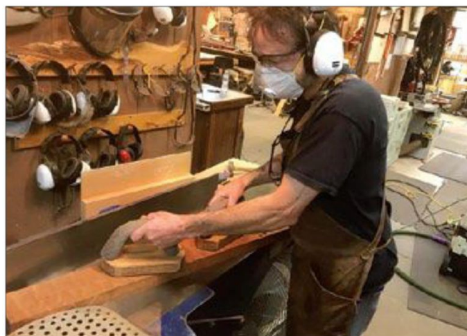
I flattened the boards by taking very light passes ( \frac{1}{64} " at a time) on my 16" jointer, outfitted with a custom made Byrd Shelix carbide cutterhead.
