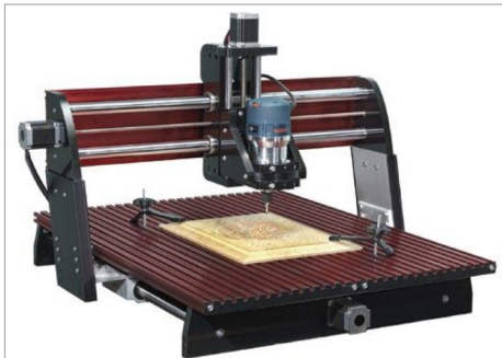
Fig 1. Three axis CNC machines move in three directions. The X and Y axes control the left to right and front to back movement. The Z axis controls the vertical movement. This machine is shown utilizing a woodworking router.
