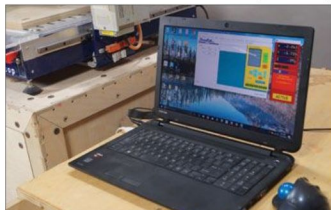
Figs 3 & 4. CNC machines connect to either a control computer (below) or a control pendant (right). These allow the operator to control the movements of the CNC machine automatically and manually.
