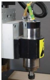
Fig 2. Using an industrial spindle, instead of a woodworking router, provides quieter operations and longer life, though more expensive.
