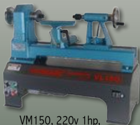
VL300, 220v, 2hp, Variable Speed 24" swing
