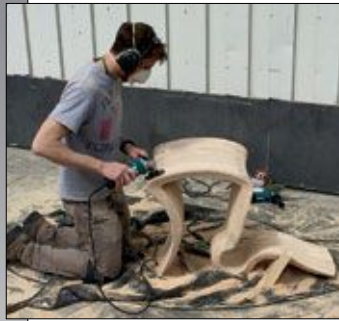
Chance Coalter (San Diego, CA) shaping his Sculptural Chair , which uses wood strips laminated in a brick pattern to give it strength.
