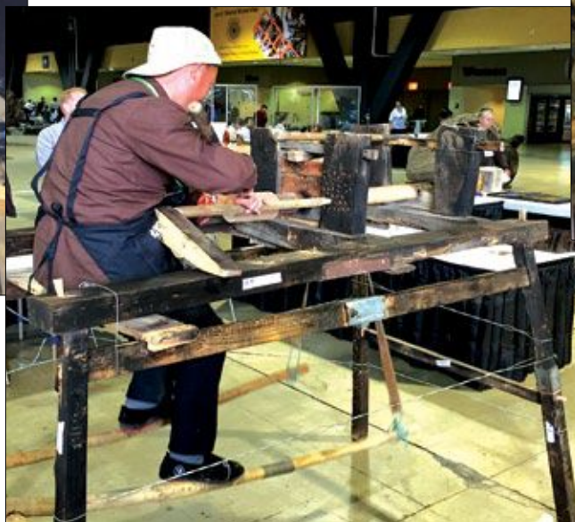
Xuemin Li (China) stays in shape while turning on a foot-powered lathe, a 2,000-year old design. In fact, there are components of the lathe, which are 300 years old. Conference visitors were encouraged to try it out.
