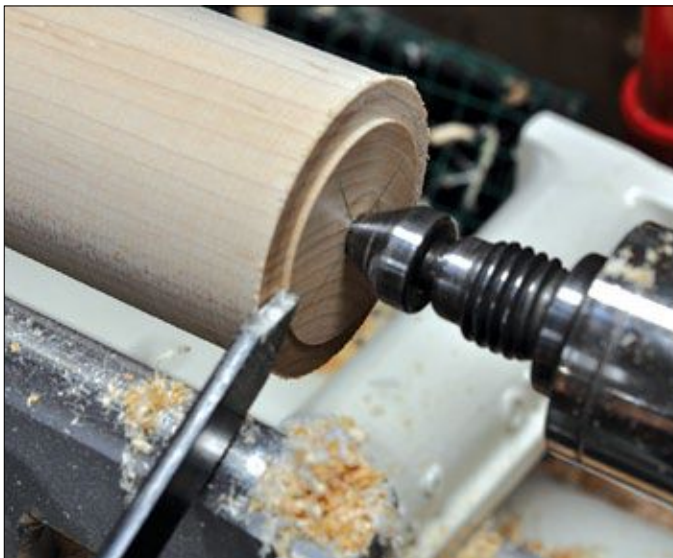
The parting tool allows you to cut the end of a cylinder or to make a tenon
