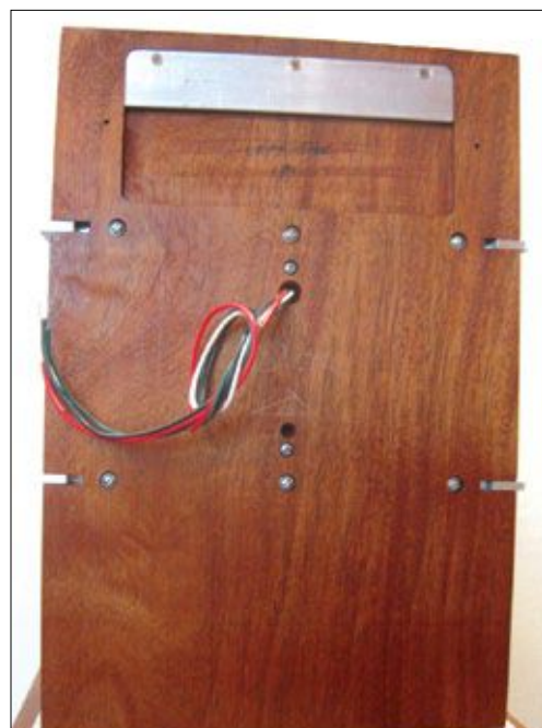
The back side of the Mahogany back board. Note the through dados on each side, where the shelves are inserted, and the screws to attach the Central Core.
