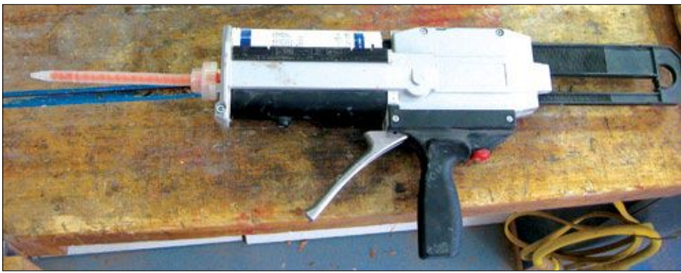
A catalyzed resin glue gun is necessary for laminating solid surface materials. The tip mixes the resin and must be replaced with each glue-up operation.
