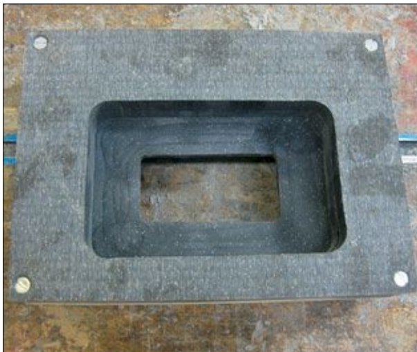
The laminated solid surface block is routed to provide an opening and space for the electrical outlet and switch combination.
