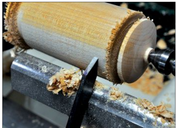
The Parting Tool allows you to make space or clearance on your work to allow access for a gouge.
