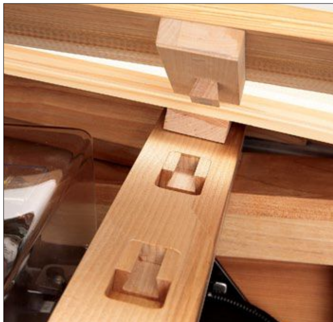
Kusabi joints are wedged tenons that hold the frame securely.
