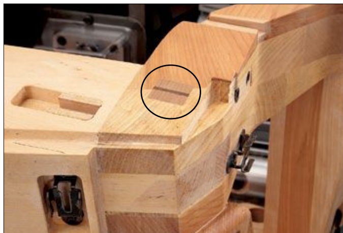
Kusabi joints are wedged tenons that hold the frame securely.
