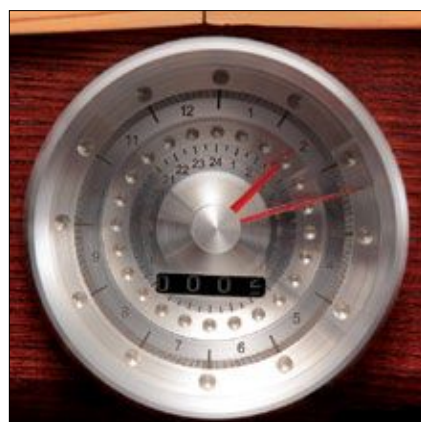
The dashboard meter measures time, rather than miles (up to 100 years).
