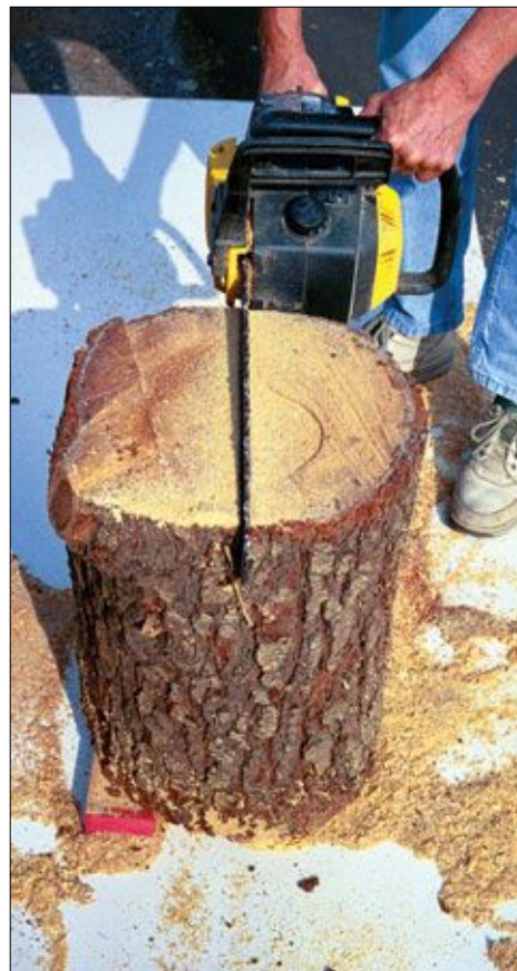
FIGURE 2. When cutting a log down the middle from its end, this end grain cut can be difficult. Resist the temptation.
