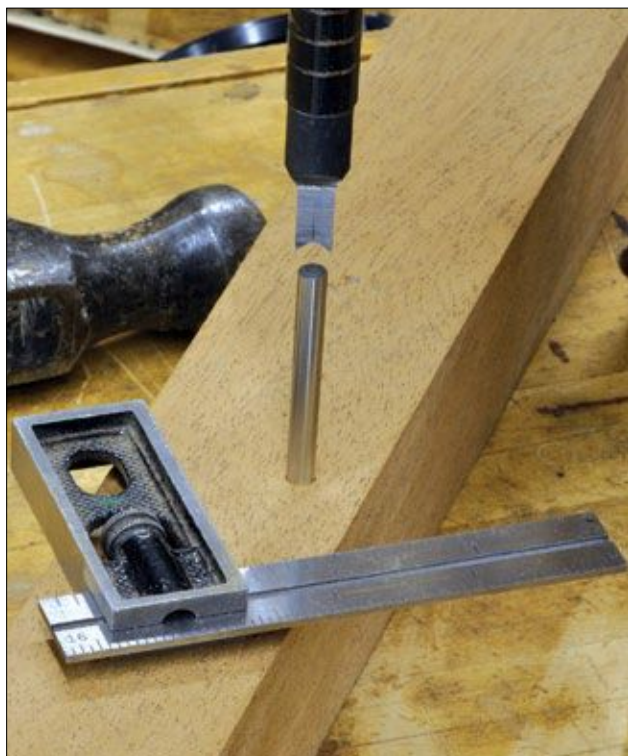
FIGURE 9. Use a short bit shank as a guide for repeated placement of square holes.
