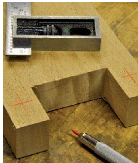
FIGURE 2. Center lines for square holes.
