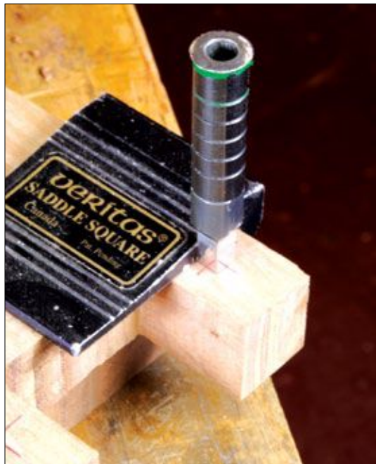
FIGURE 4. Tap with a steel hammer to register the points of the tool.
