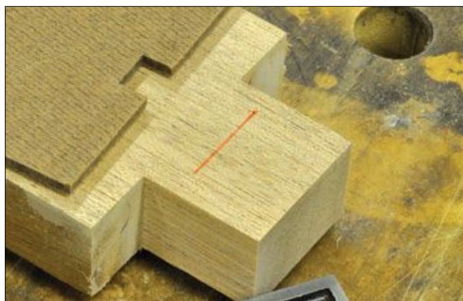
FIGURE 7. Hardboard template, with bottom guideline drawn.
