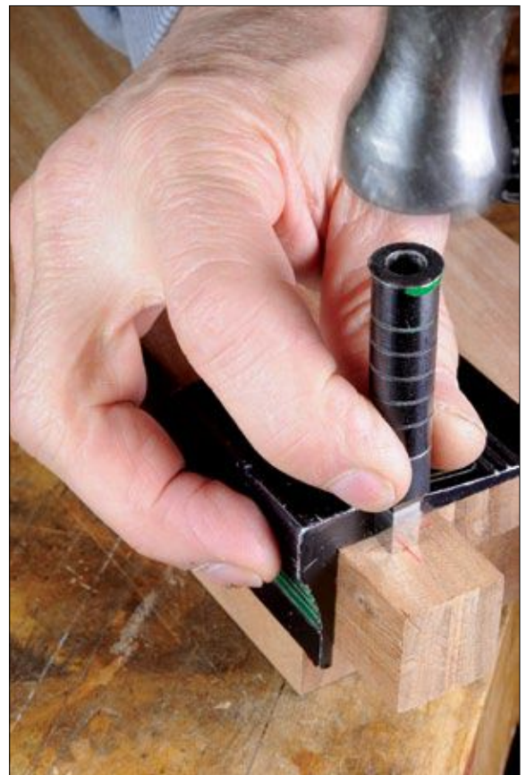
FIGURE 5. With a twist bit installed in the drill press, align the punch over center lines.
