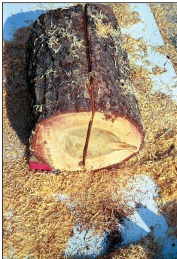
FIGURE 4. Don't cut all the way through; turn the log over. When you break through, avoid hitting dirt, rocks, or concrete with the chain.
