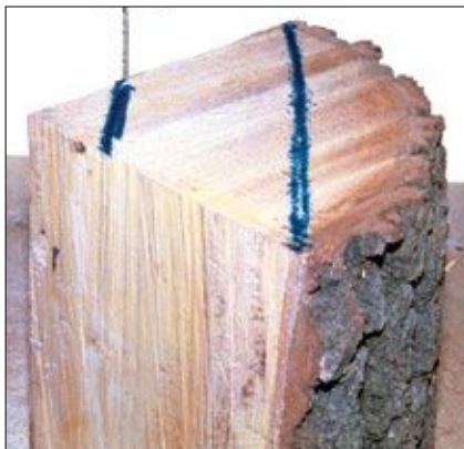
FIGURE 6. Cut lines on a quarter log for turning a natural edge bowl.
