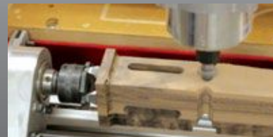
Using the turning system to mill the legs and mortise/tenon joints.
