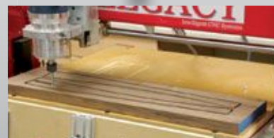
Milling the chair back stiles on the horizontal worktable.
