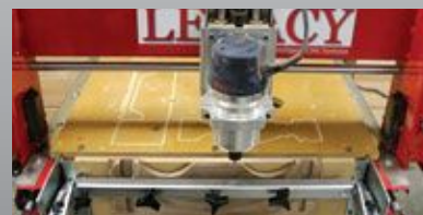
Cutting the back splat mortise with the panel clamp.
