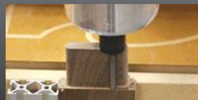
Cutting the straight tenon on the vertical work table.
