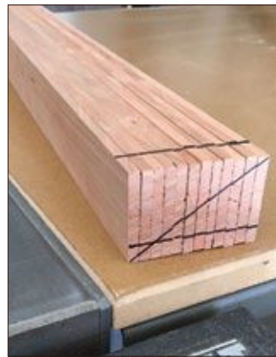
FIGURES 12 & 13. Flipping every other laminate during the tapering process will compensate for any inaccuracy in the jig's squareness.
