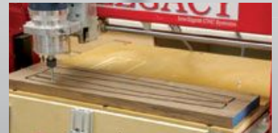
Milling the chair back stiles on the horizontal worktable.
