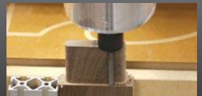
Cutting the straight tenon on the vertical work table.
