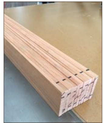
FIGURES 12 & 13. Flipping every other laminate during the tapering process will compensate for any inaccuracy in the jig's squareness.
