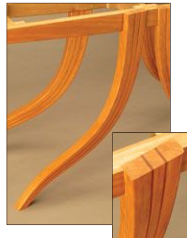
FIGURES 6 & 7. 13 tapered laminates in Cherry and two untapered laminates in Mahogany were used to create this table leg. At the top the leg is 3" wide, \frac{1}{8} " at the bottom.
