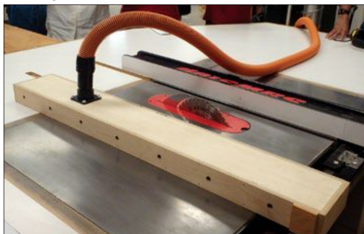
FIGURE 1. Ouwehand's jig for cutting tapered laminations on the table saw includes a vacuum hose adapter—allowing it to be connected to a shop vacuum—and holes to create the suction needed to hold the laminate in place during the tapering process.
