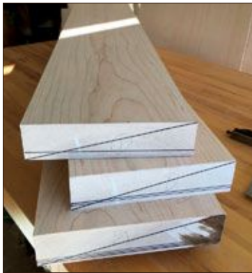
FIGURE 11. Mark your wood clearly, so that you can return the laminates to the correct order after each process.
