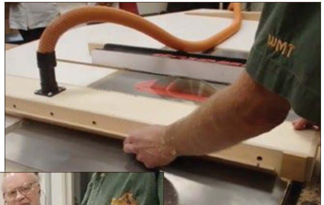
FIGURE 14. With the vacuum running, adhere the strip to the tapering jig. Be sure it is flush to the table and against the back stop.
