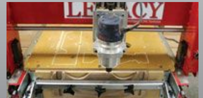
Cutting the back splat mortise with the panel clamp.
