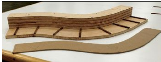
FIGURE 5. The pattern is created from the full-size drawing. This is used to make the bending form. It had to be sturdy enough to support the more than 20 clamps it took for this glue up.
