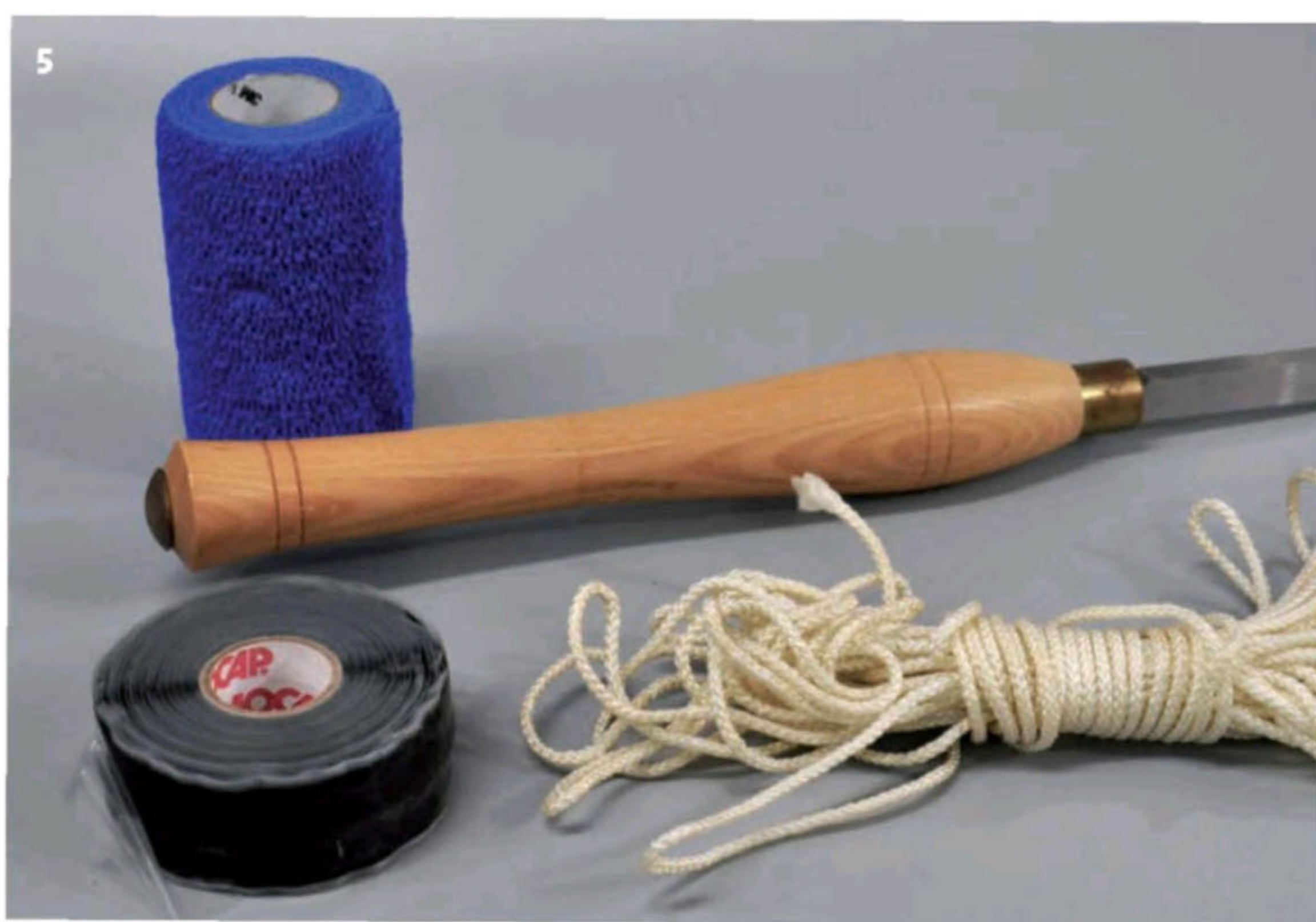
5 Many turners use some form of tape to wrap tool handles. Others use some rope, or a combination of both products. The blue tape in the photo is a tape originally developed for veterinarians and often sold as a wound-care product. The black tape is a silicone product that sticks to itself. Neither leaves a residue on a handle and both work well
