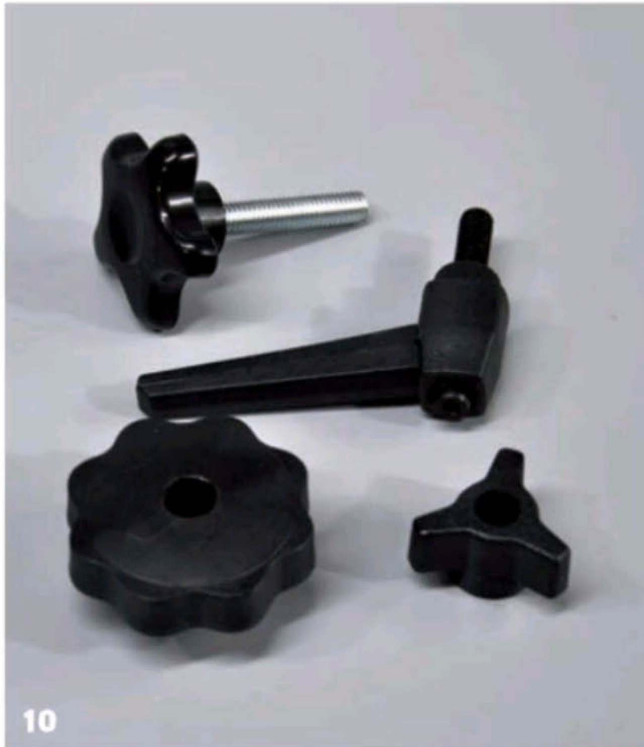
10 Here are a few styles of replacement knobs you would find in use in my shop. If a tool or jig has a knob that is hard for you to turn, look at options. The larger-diameter round knobs with finger grooves and lever-style knobs are easier on the hands
