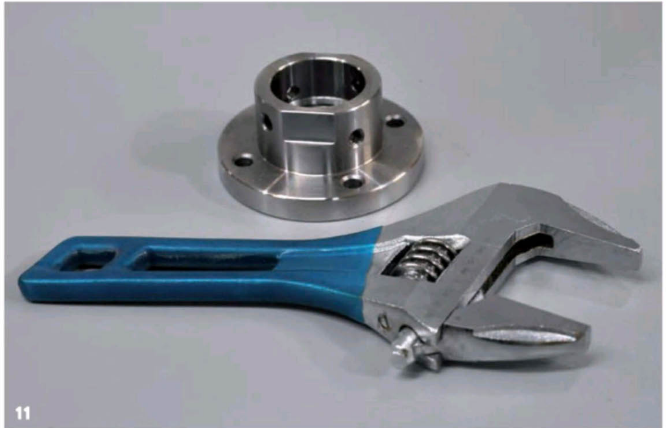
11 This Japanese-style adjustable wrench can replace all those stamped spanners that come with lathe accessories. They are far easier on the hand and work well in my shop
