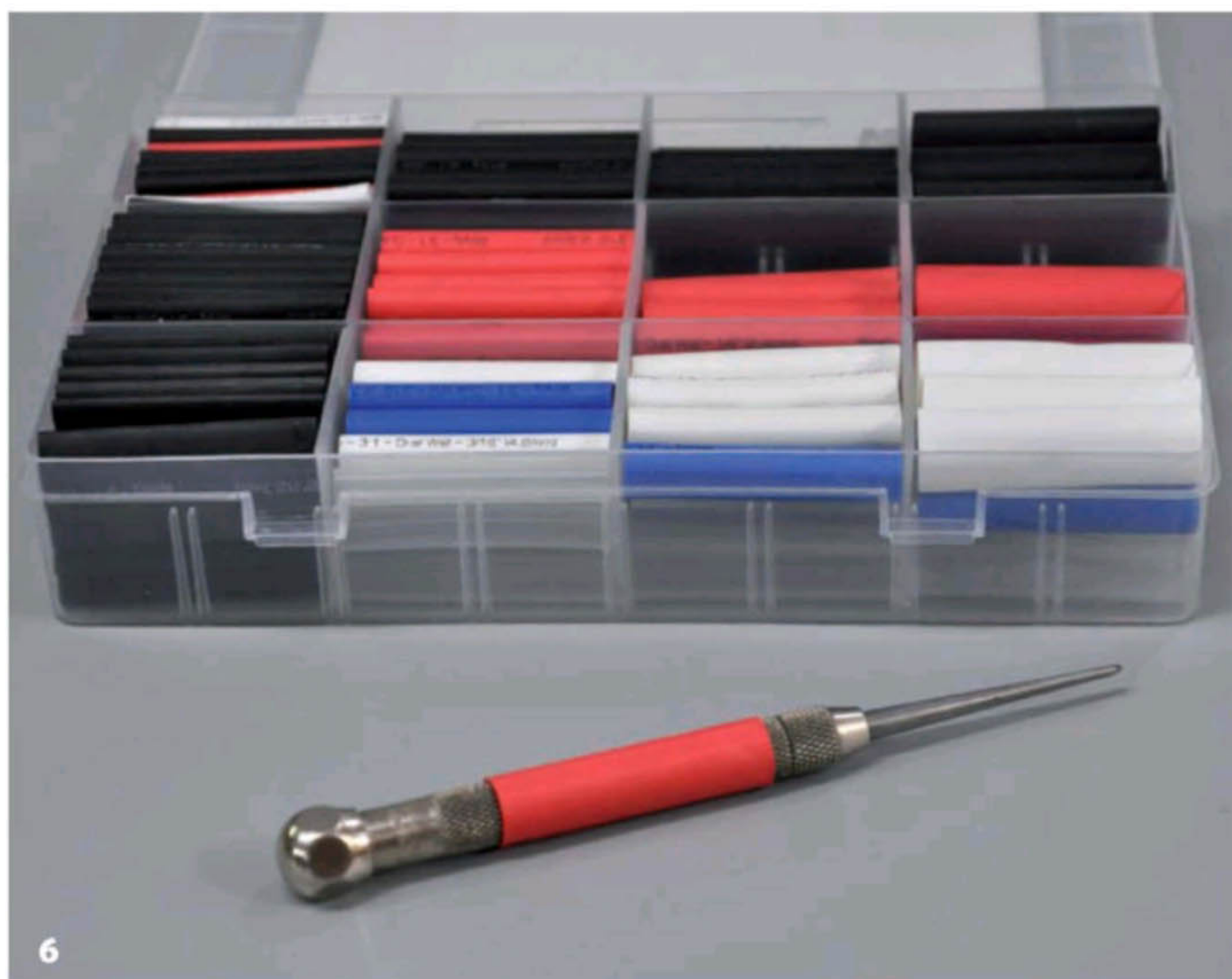
6 Heat-shrink tubing, sold for electrical applications, works well for small-diameter auxiliary grips. You can see here how it makes this centre punch easier to identify and grab
