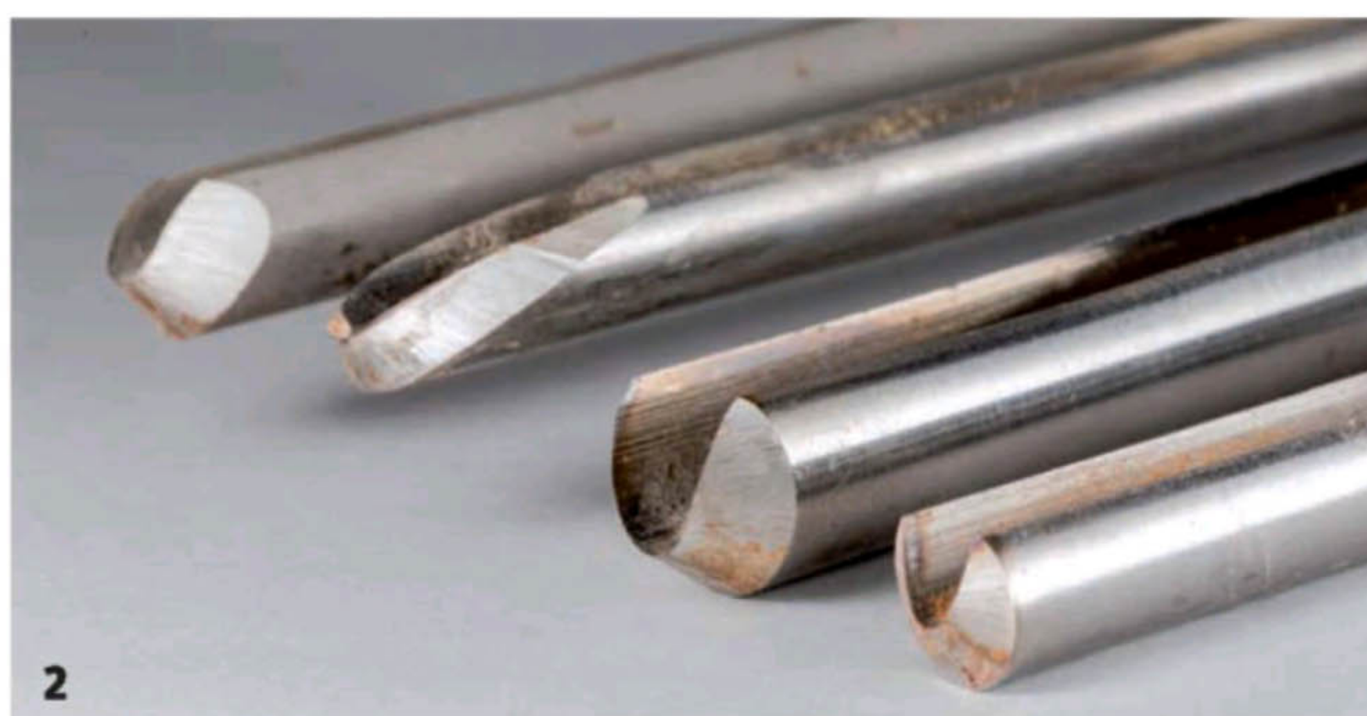
1 Different gullet shapes and your chosen grind will perform different tasks. Ultimately, you'll have several (many?) bowl gouges 2 Here are a few of my many bowl gouges. The different sizes, shapes, and grinds do the different tasks well
