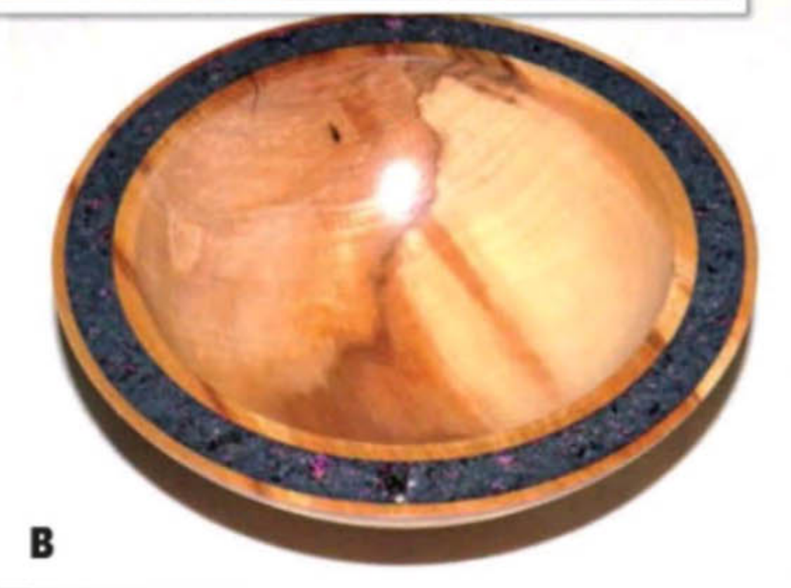
A-B The cellulose finish on the inlay C Here's more detail of the opalescent finish before the cellulose spray D After a coat of high gloss lacquer
