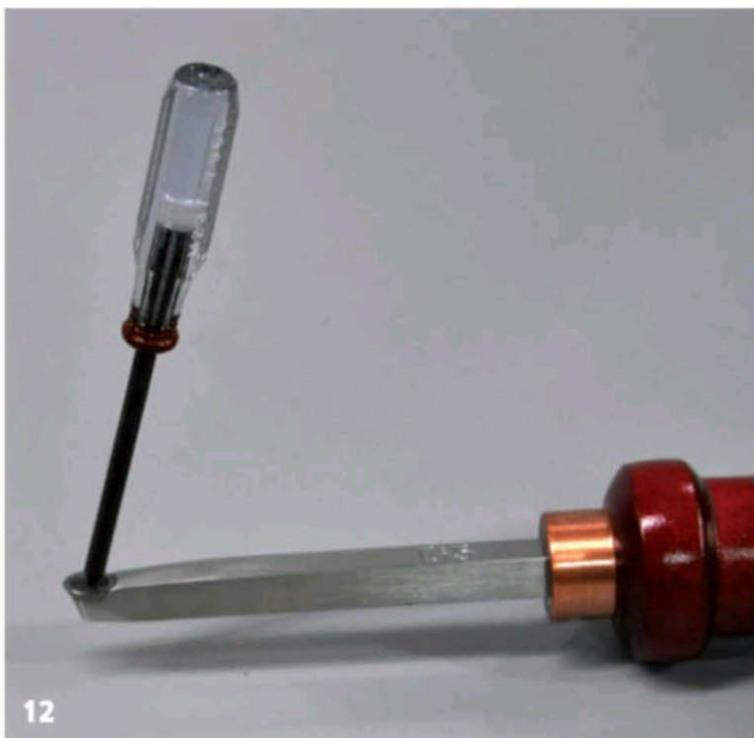
12 The little Allen screws on carbide insert tools are far easier to change with a screwdriver-style wrench. This one has a ball end to find the tiny screw hole even at an angle
