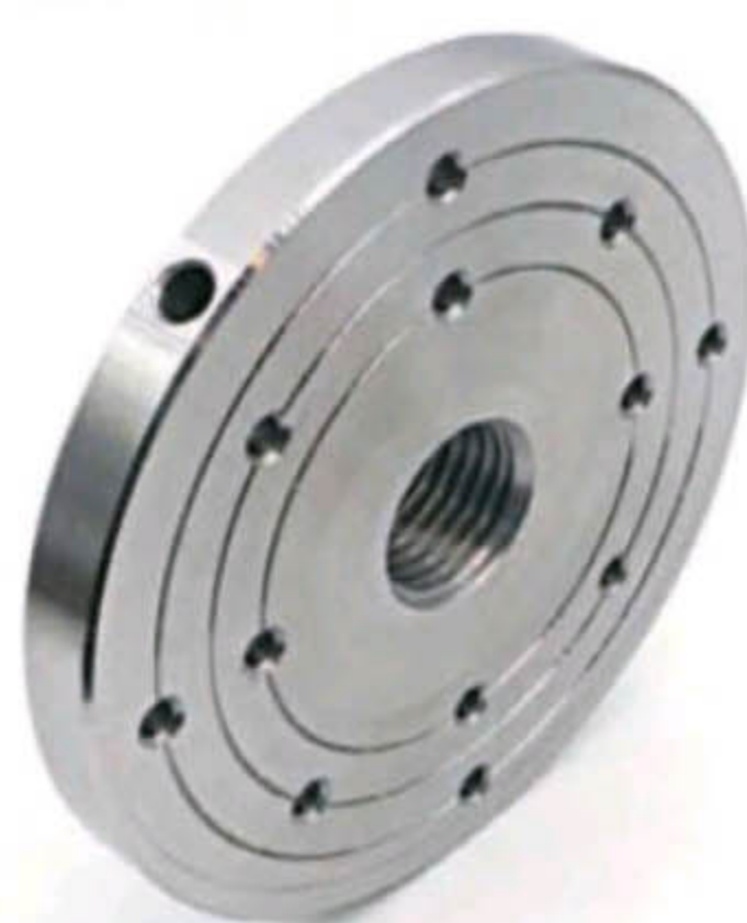
Lathe faceplates: Available in 80mm, 105mm & 150mm diameters. M33x3.5, 1x8tpi, 3/4x16tpi or 1 1/2x6tpi
