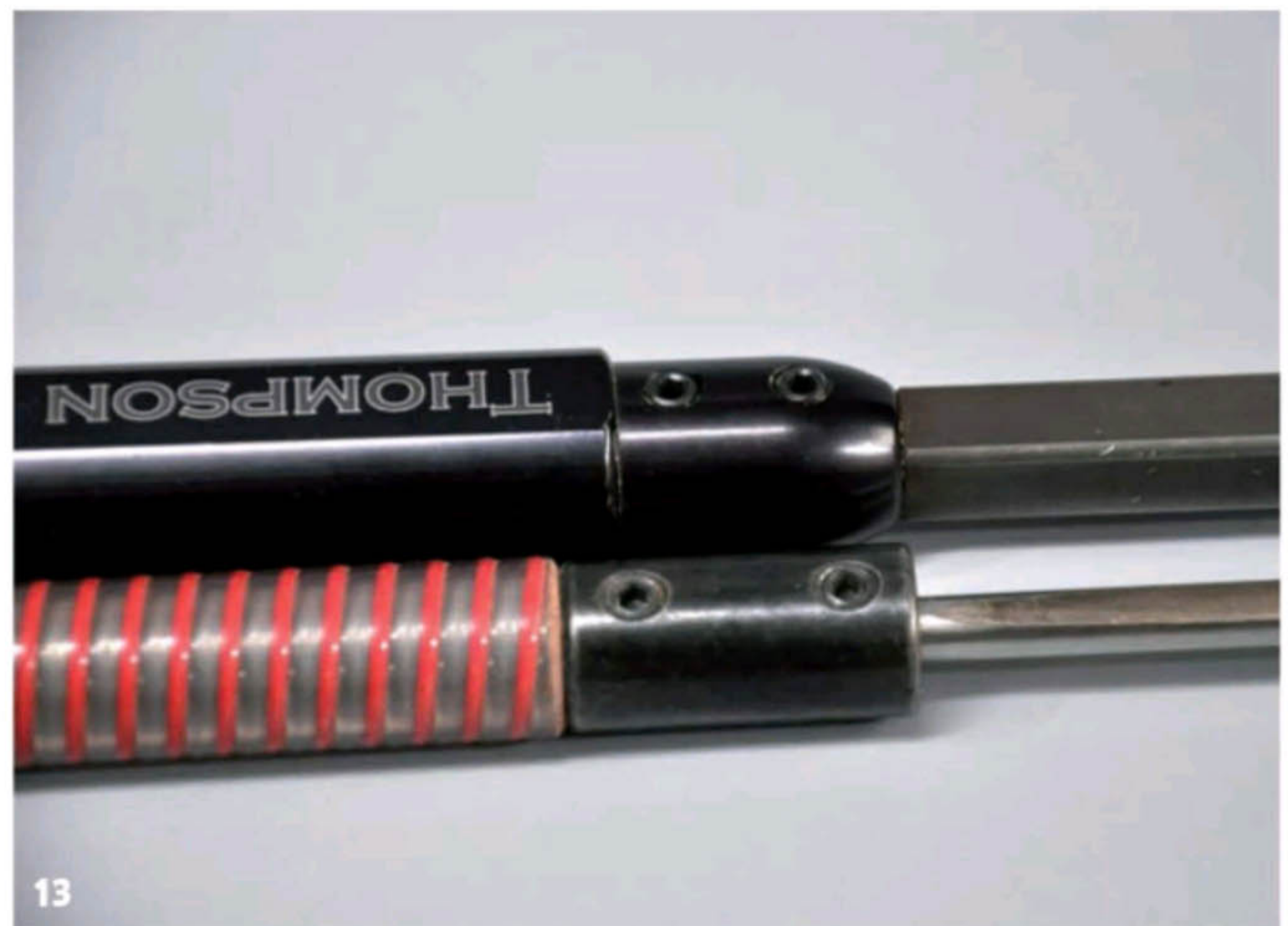
13 On any replacement handle that uses set screws, you want full engagement of the threads in the handle, yet the screws should be slightly flush or below the surface of the handle to prevent injury. This may require you to replace the factory set screws with longer or shorter ones depending on the situation
