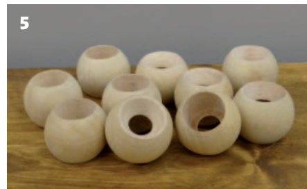
4 Turning the inside of the balls
