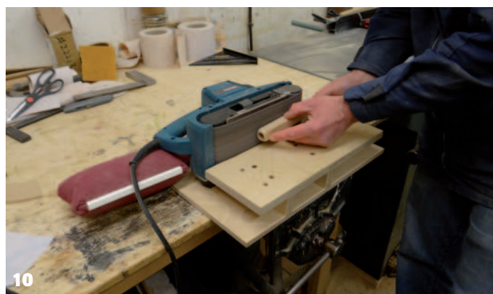
7 The pan with the original damaged handle 8 Using the planer to shape the sides of the handle 9 Turning the handle 10 Refining the handle on the sander 11 The pan with its new handle
