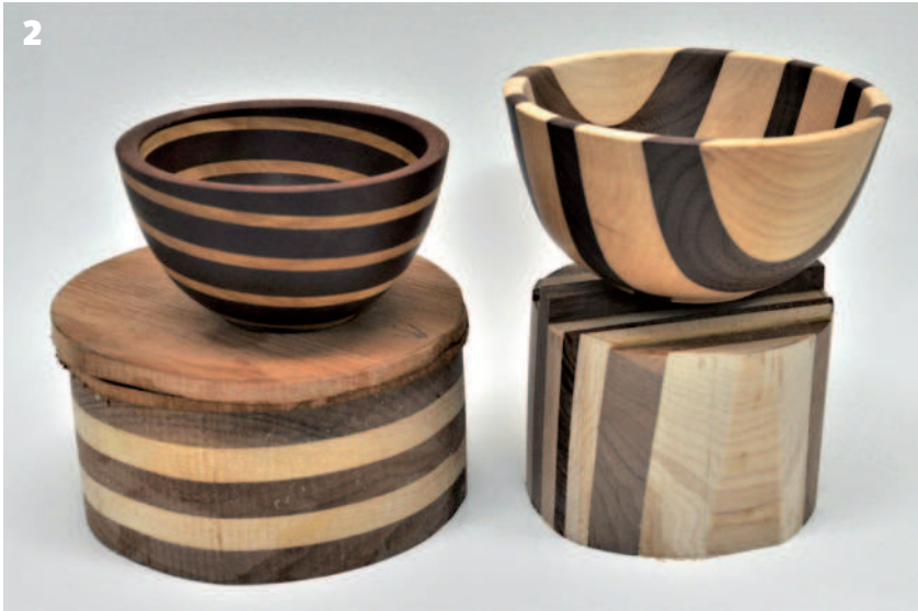
2 Examples of horizontal and vertical orientation for a bowl 3 Develop a pleasing design and dry-fit the pieces before gluing 4 Glue up the blanks using good gluing techniques 5 Clamp the glue-up and let it sit for 24 hours
