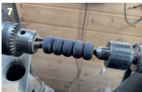
7 Oak beaded pull ready to sand in the lathe with a dowel and revolving centre for support 8 Scrubbing the grain clean with liming brush 9 Filled with gold gilt cream
