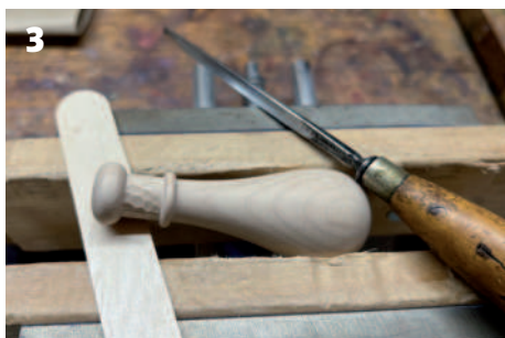
3 Sycamore beaded teardrop being carved 4a Sycamore carved teardrop – gesso being applied 4b Sycamore beaded teardrop size coat application copy 5 Sycamore beaded teardrop – flakes applied with soft, fluffy brush 6a Oak beaded teardrop – carved 6b Oak beaded teardrop – flakes
