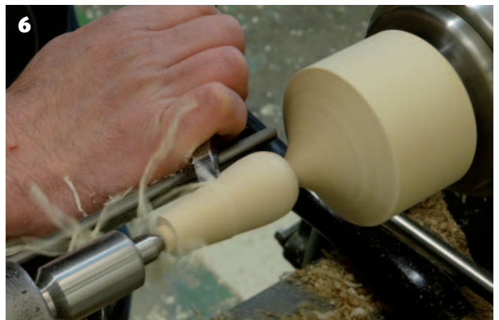
3 Turning to a cylinder with my spindle roughing gouge 4 Rolling the bottom curve 5 Sizing the top of the teardrop 6 Planing the gentle curve down to the narrowest part of the teardrop 7 The difference in shavings between oak and sycamore using the same cut was interesting 8 Slicing the end grain 9 The finished teardrop pulls
