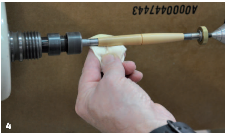
2 Surface preparation 3 Building a finish in layers 4 Turn up speed and generate heat to cure the finish completely 5 Wide assortment of friction polishes
