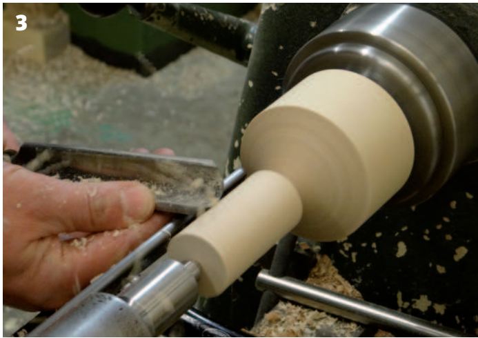
3 Turning to a cylinder with my spindle roughing gouge 4 Rolling the bottom curve 5 Sizing the top of the teardrop 6 Planing the gentle curve down to the narrowest part of the teardrop 7 The difference in shavings between oak and sycamore using the same cut was interesting 8 Slicing the end grain 9 The finished teardrop pulls
