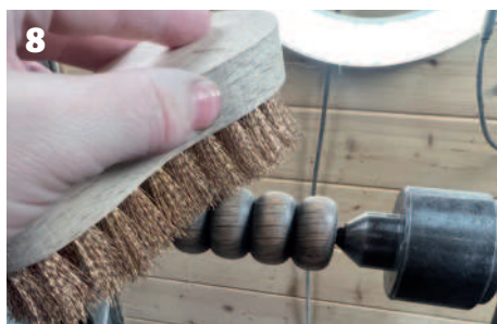
7 Oak beaded pull ready to sand in the lathe with a dowel and revolving centre for support 8 Scrubbing the grain clean with liming brush 9 Filled with gold gilt cream
