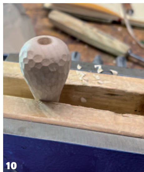
10 Sycamore teardrop being carved all over 11a Sycamore teardrop being dry brushed 11b Sycamore teardrop – dry brushing complete
