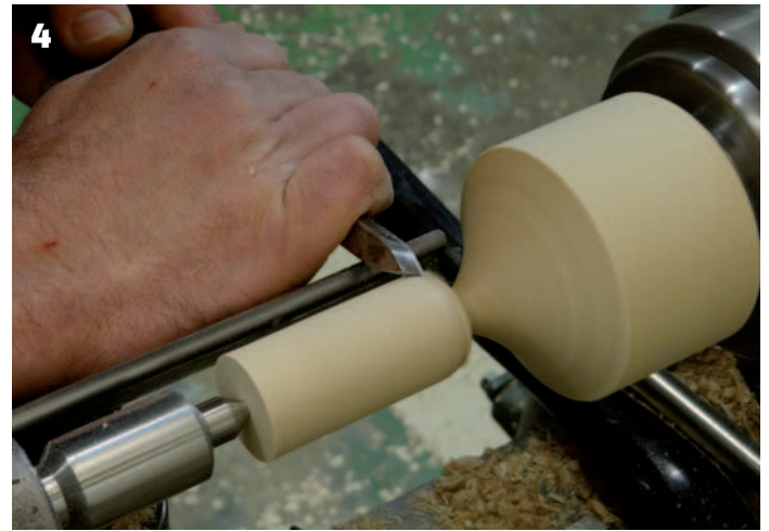
3 Turning to a cylinder with my spindle roughing gouge 4 Rolling the bottom curve 5 Sizing the top of the teardrop 6 Planing the gentle curve down to the narrowest part of the teardrop 7 The difference in shavings between oak and sycamore using the same cut was interesting 8 Slicing the end grain 9 The finished teardrop pulls
