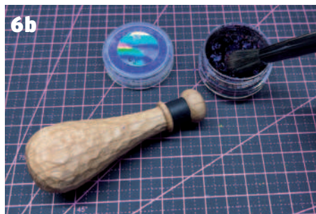
3 Sycamore beaded teardrop being carved 4a Sycamore carved teardrop – gesso being applied 4b Sycamore beaded teardrop size coat application copy 5 Sycamore beaded teardrop – flakes applied with soft, fluffy brush 6a Oak beaded teardrop – carved 6b Oak beaded teardrop – flakes
