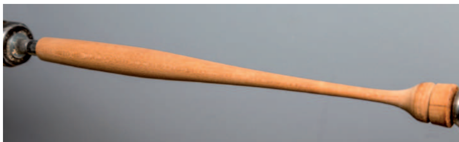
The uphill vs downhill surface finish changes I have run into on rare occasions have been with cherry or oak. They usually occur on long, gentle radius curves
