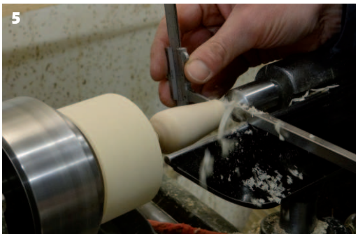
3 Turning to a cylinder with my spindle roughing gouge 4 Rolling the bottom curve 5 Sizing the top of the teardrop 6 Planing the gentle curve down to the narrowest part of the teardrop 7 The difference in shavings between oak and sycamore using the same cut was interesting 8 Slicing the end grain 9 The finished teardrop pulls
