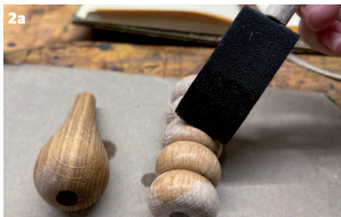
2a Applying the tannin solution 2b Ebonising process
