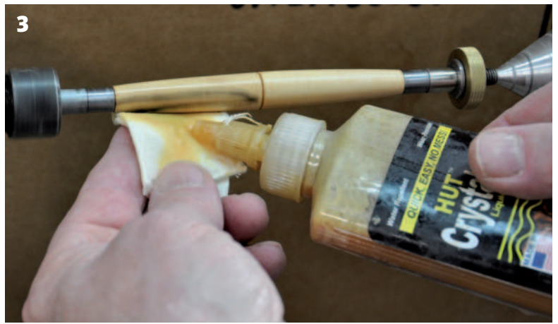
2 Surface preparation 3 Building a finish in layers 4 Turn up speed and generate heat to cure the finish completely 5 Wide assortment of friction polishes
