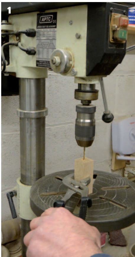
1 Drilling the blanks 2 Mounting on the wooden cone
