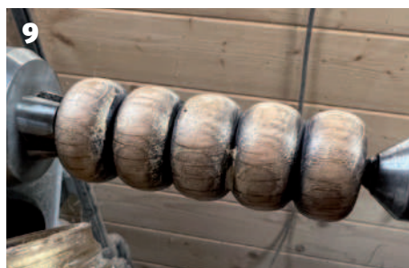
7 Oak beaded pull ready to sand in the lathe with a dowel and revolving centre for support 8 Scrubbing the grain clean with liming brush 9 Filled with gold gilt cream
