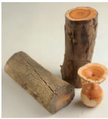
Left: Boxwood and yew sold as sections of branch or small trunks. The left-hand boxwood section has split
