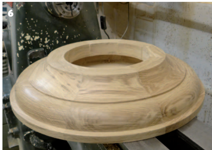
4 The table pedestal base on the lathe with the gap-bed removed and the cranked banjo in place 5 Shavings fly from my negative rake scraper as I turn the table base 6 The finished table base
