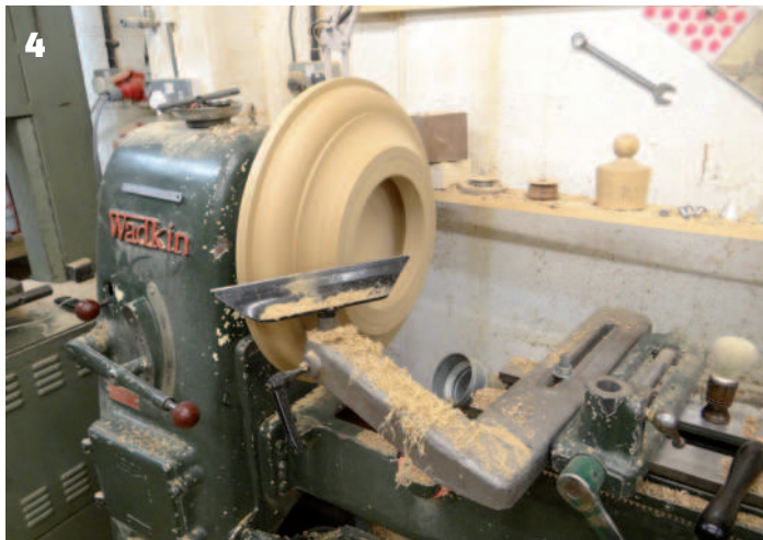
4 The table pedestal base on the lathe with the gap-bed removed and the cranked banjo in place 5 Shavings fly from my negative rake scraper as I turn the table base 6 The finished table base
