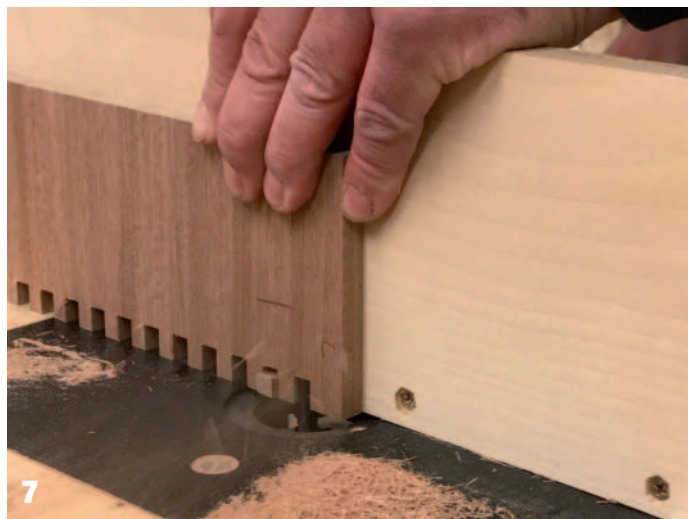
7 Cutting the finger joints (for the boxes)
