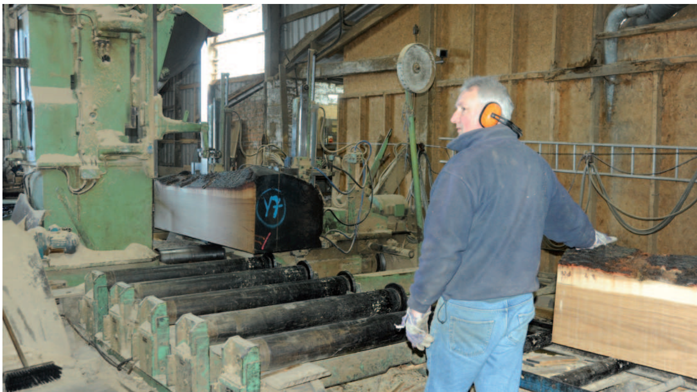
Above: A log being sawn into boards
