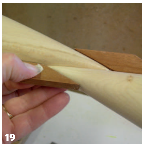
A Using the shape finder. B Transferring the fins' shape to the timber
