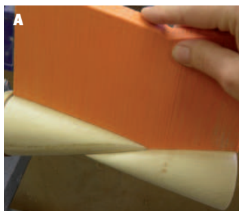
A Using the shape finder. B Transferring the fins' shape to the timber
