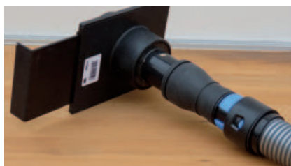
All the adapted pipes fit into the 65mm blast gates of the Axminster extraction system
