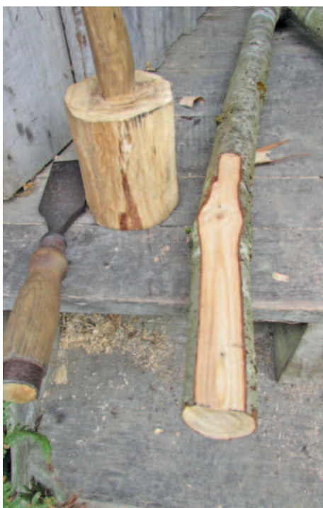
19 Chiselling the flats on the treadle for the 'T'-hinges.
