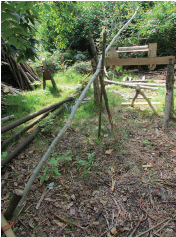
22 Setting up the pole: the support can be moved backwards or forwards to find the right amount of spring in the pole
