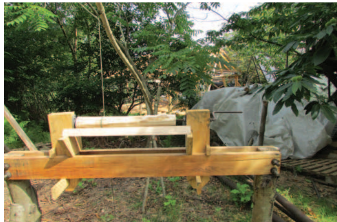
23 Ready to go: notice the tool rest across the poppets
