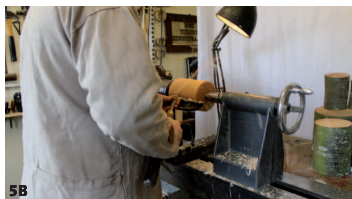
5A End-grain green wood log mounted between centres 5B Roughing down a green wood log blank
