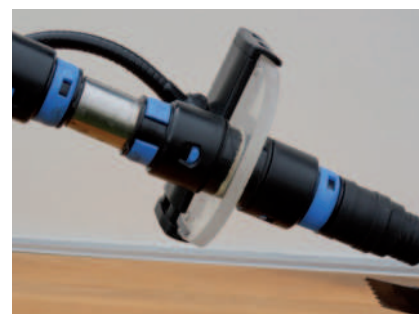
Two CT collars sandwiched between a sheet of acrylic
