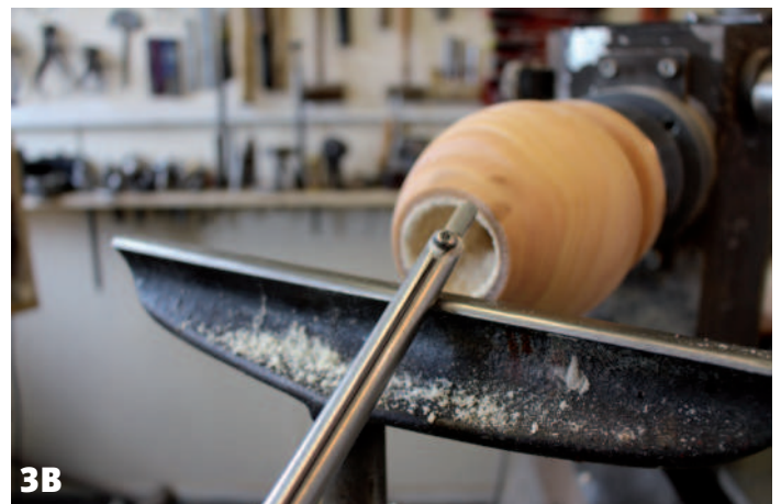
3 Above images show a shop-made toothpick DHT and the tool in use
