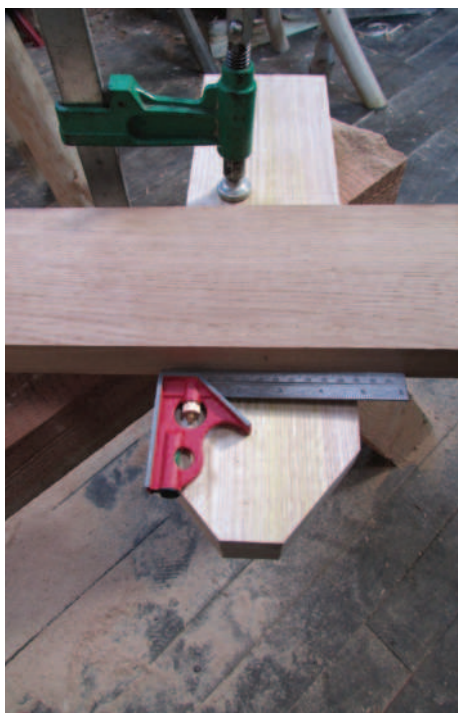
7 Laying the bed plank over the poppet to mark the top and bottom lines
