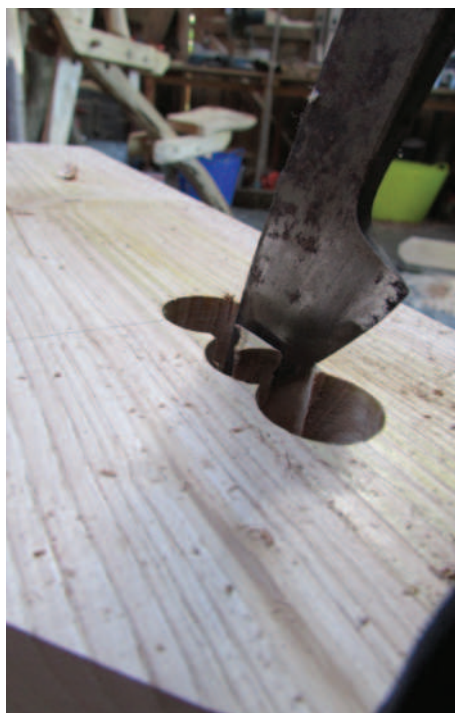
8 Using the try-bill to cut the mortice edges
