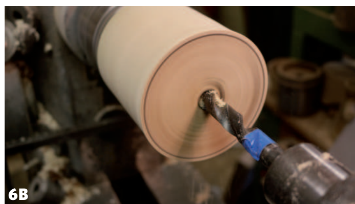
6A End grain marked to show faster and slower running wood 6B Using a twist drill to bore out the slower-running centre wood
