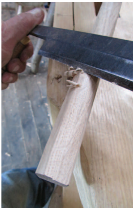
10 Creating a curve on the tapered edge of the key with a draw knife
