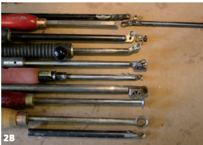
2A Evolution of the toothpick-type tool, 2B Evolution of the hook tool to the shielded cutter
