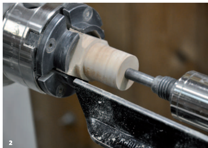
This flat-ended pin supports the work without penetrating it
