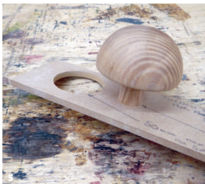
4 The holes I received with the doughnuts 5 Testing and end cap for fit in the hole
