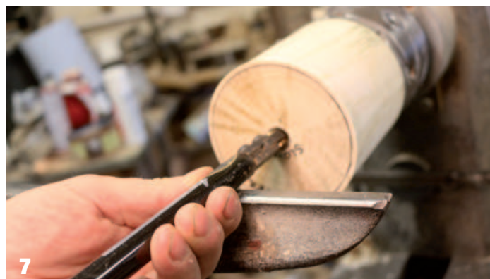
7 White marking made on top of shaft to show when cutter is at 45° to the wall of the vessel
