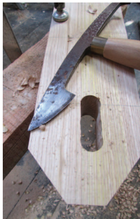
9 The completed mortice
