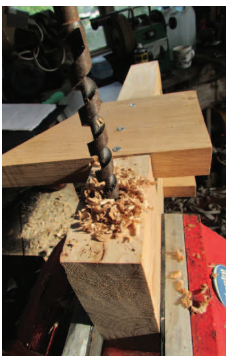
15 Drilling through the poppet for the cranked handle threaded bar
