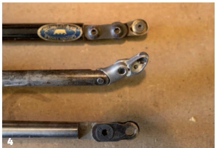
4 Three types of shielded cutter DHTs
