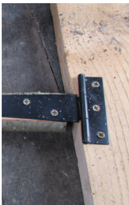
20 A 'T'-hinge joining the treadle branch to the footplate
