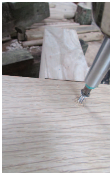
12 Fixing the poppet rests to the poppets using stainless steel screws. Always pilot the hole prior to screwing through the wood with a drill bit slightly smaller than the diameter of the screw to avoid splitting the wood
