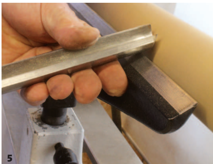
3 Typical examples of fabricated toolrests commercially available 4 An example of a commercially made, forged steel toolrest 5 A well-designed, forged steel toolrest allows a good grip on the tool 6 An underhand grip, with the thumb on top, acts as an aid to maintaining a constant depth of cut
