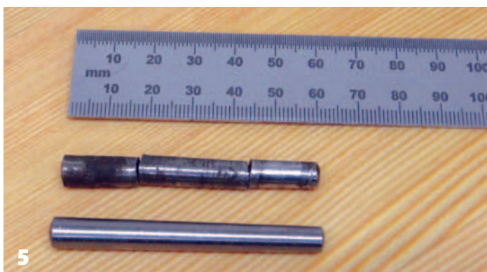
3 The speed-change lever and part of the internal mechanism, removed from the lathe 4 The lathe with the arm removed 5 The offending tapered pin with the replacement 6 Reassembled, the lathe is running better than it has in years
