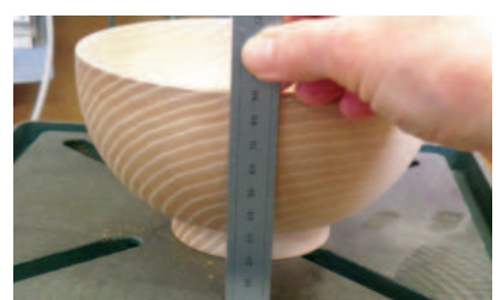
Measuring the overall height
