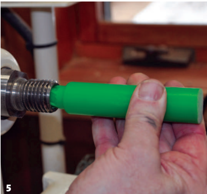
1 Four-prong drive centre 2 The drive centre and diamond sharpening paddle 3 Polish the drive shaft with a non-abrasive pad 4 A little oil or wax protects the tool 5 Clean out spindle taper 6 Check alignment of headstock and tailstock
