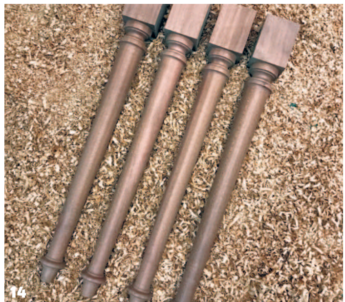
11 The laminated sapele columns, ready for turning 12 Turning one of the columns 13 The finished columns, showing the entasis 14 The sapele table legs
