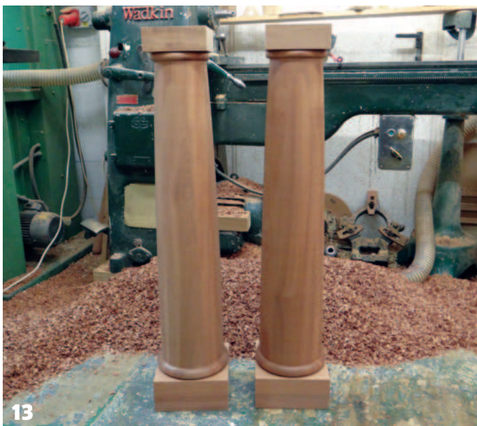
11 The laminated sapele columns, ready for turning 12 Turning one of the columns 13 The finished columns, showing the entasis 14 The sapele table legs
