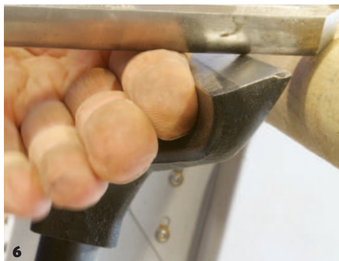
3 Typical examples of fabricated toolrests commercially available 4 An example of a commercially made, forged steel toolrest 5 A well-designed, forged steel toolrest allows a good grip on the tool 6 An underhand grip, with the thumb on top, acts as an aid to maintaining a constant depth of cut
