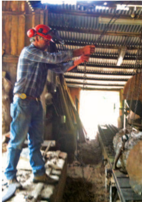
Nigel setting a portion of the tree on the mill bed
