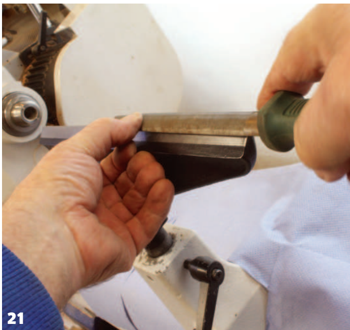
18 Bowl gouge held with bevel rubbing and good support from the toolrest 19 The point at which the radiused toolrest can sometimes obstruct the gouge 20 Note the toolrest-friendly edges of the Sorby skew chisel 21 Gently filing along the top edge, keeping the file at a constant angle 22 Iron filings should fall on to an appropriate barrier/paper
