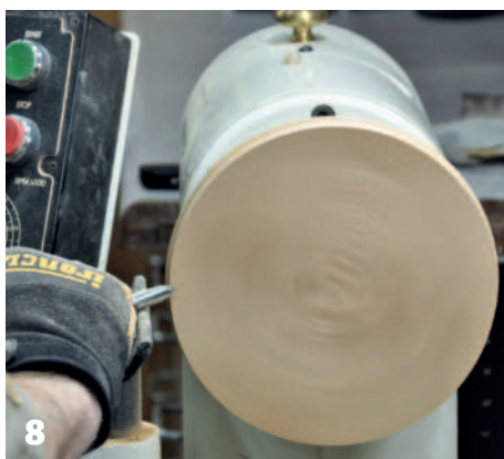
7 We have work ahead of us – the scrap pile yielded a lot of pieces 8 True up the edge to bring work to round and establish approximate diameter 9 Remove excess wood with step cuts and true up the bottom 10 Mark out the tenon with a compass
