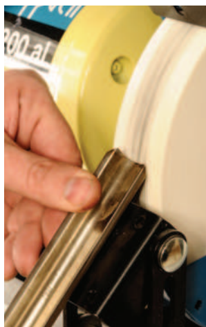
Present your gouge to the wheel with the flute pointing to 2 o'clock...
