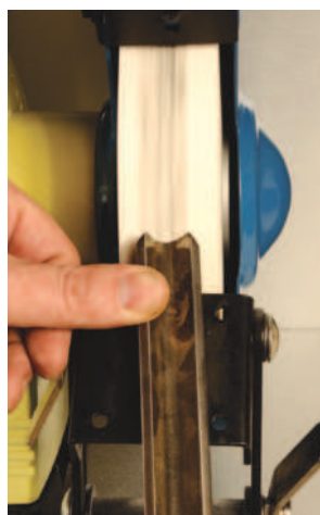
... then rotate the gouge along its axis, keeping firm pressure...
