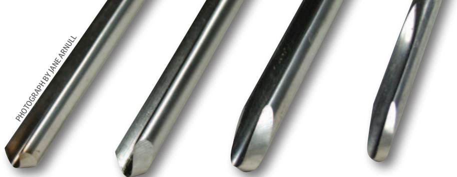
Here are four bowl gouge profiles. The normal profile on the left is followed by successively more swept-back grinds
