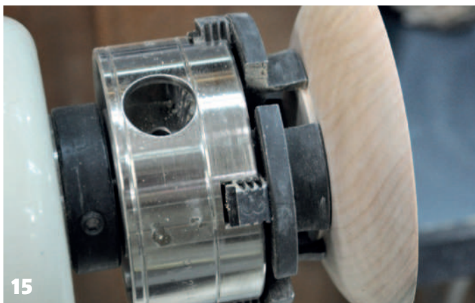
11 Remove excess wood and shape outside of your work 12 Rotate bowl gouge to lightly use wing to carefully shear scrape the piece to final shape 13 Power and hand sand outside. Note some scratches remain that need to be removed in this picture 14 Finished outside of a plate 15 A small, well-cut tenon will hold the work and become the finished bottom 16 Face off the work and establish your rim
