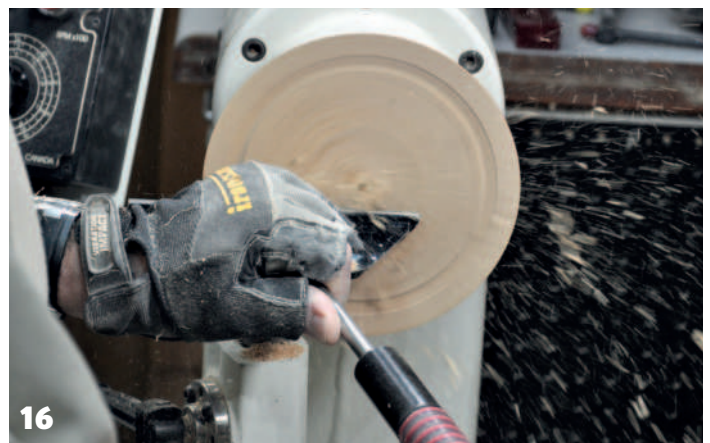
11 Remove excess wood and shape outside of your work 12 Rotate bowl gouge to lightly use wing to carefully shear scrape the piece to final shape 13 Power and hand sand outside. Note some scratches remain that need to be removed in this picture 14 Finished outside of a plate 15 A small, well-cut tenon will hold the work and become the finished bottom 16 Face off the work and establish your rim
