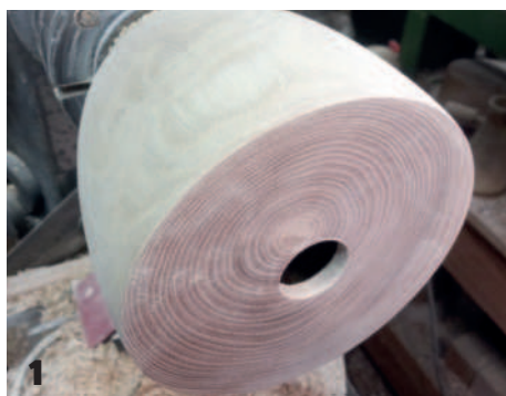
1 Sweet chestnut pot on the lathe 2 Pot stained with iron sulphate solution, and lime waxed – end-grain view 3 Side-grain view
