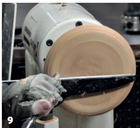
7 We have work ahead of us – the scrap pile yielded a lot of pieces 8 True up the edge to bring work to round and establish approximate diameter 9 Remove excess wood with step cuts and true up the bottom 10 Mark out the tenon with a compass
