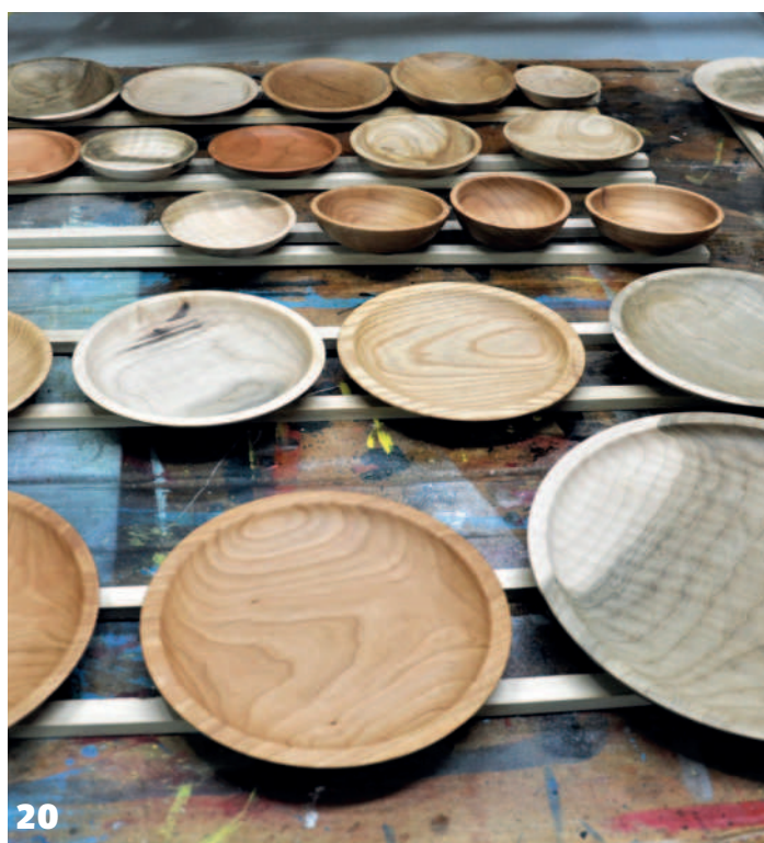
17 Refine the outer section of a plate with a scraper – note the wood towards the centre of the plate remains in place to dampen vibration 18 Power sand with your first grit to remove any tear-out or small bumps 19 A finished piece right off the lathe – note shavings off sharp tools 20 Apply a food-safe oil finish and allow to dry – note this is an additive project 21 The final yield from our pile of scraps
