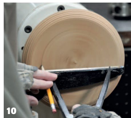
7 We have work ahead of us – the scrap pile yielded a lot of pieces 8 True up the edge to bring work to round and establish approximate diameter 9 Remove excess wood with step cuts and true up the bottom 10 Mark out the tenon with a compass
