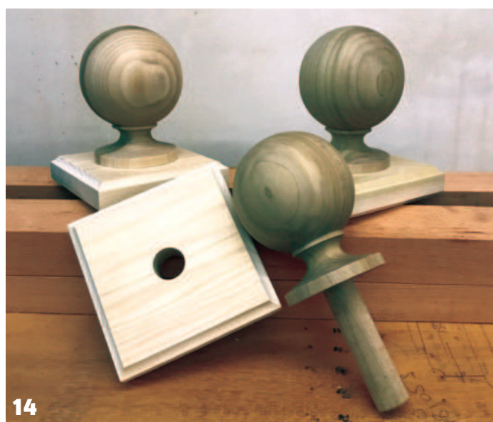
11 The restored newel, complete with finial 12 Turning the ball finial 13 Sanding the end with the finial held in the chuck 14 The finished finials and caps
