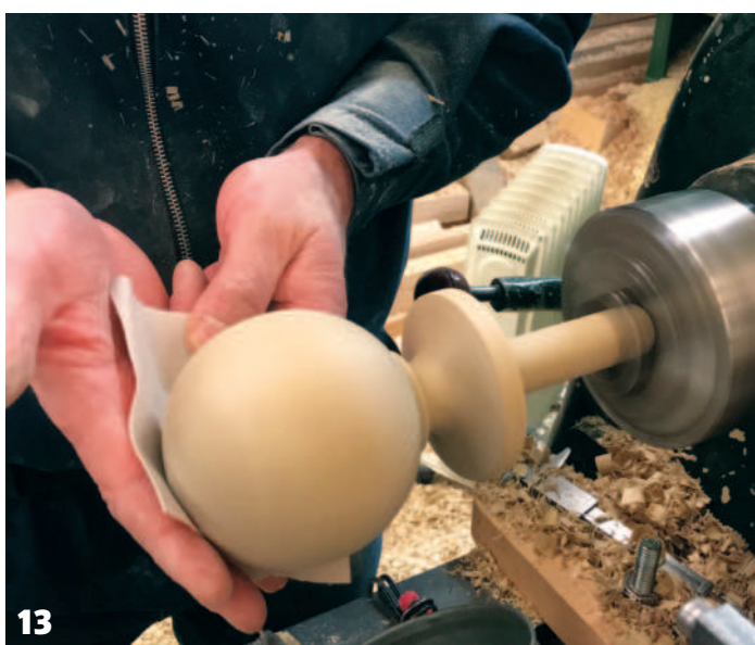
11 The restored newel, complete with finial 12 Turning the ball finial 13 Sanding the end with the finial held in the chuck 14 The finished finials and caps
