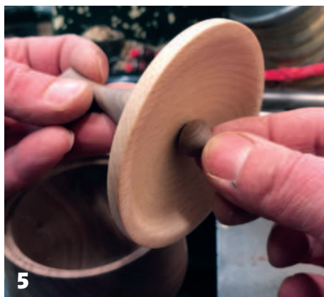
2 Books are a valuable source of inspiration 3 Turning the bowl/base of the box 4 The three finials I made for the project 5 Fitting the drop finial 6 The finished box/lidded bowl
