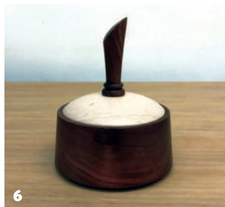
2 Books are a valuable source of inspiration 3 Turning the bowl/base of the box 4 The three finials I made for the project 5 Fitting the drop finial 6 The finished box/lidded bowl
