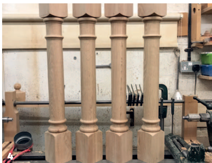
1 The finished stacks of turned rings 2 A ring with the original section of moulding, the sketch shows the style of moulding 3 The set of three table legs 4 The oak pilaster columns 5 Classic Forms is an essential reference
