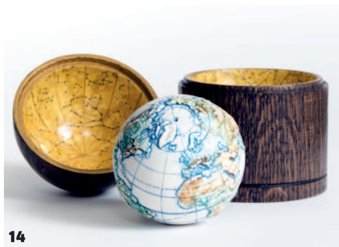
11 Using the sphere jig to turn the outside of the hemispheres 12 Hollowing the inside with a negative rake scraper, the work held in my special custom chuck 13 Some of this batch of globe boxes 14 A finished desk box and globe, ebonised and lined with parchment
