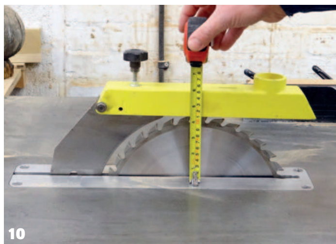
6 My three spindle gouges, showing how much more I use the 10mm 7 The new gouge compared to the old 8 Sharpening the new gouge 9 My new signature beading and parting tool 10 The crown guard on my saw, newly adjusted to take full advantage of the blade diameter
