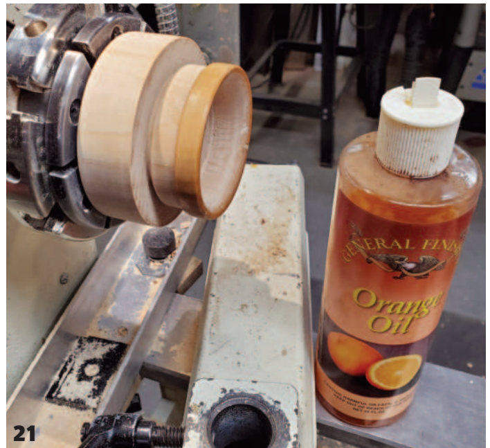
18 Aligning on centreline 19 Positioning the base 20 Thread cutting complete 21 Oiling the thread area
