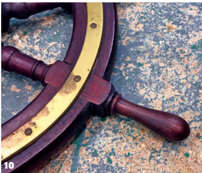
8 Finished shell 9 Damaged handle on the ship's wheel 10 New handle finished and fitted 11 Finished ship's wheel
