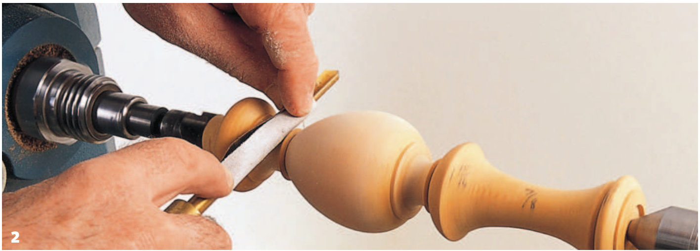
2 Making use of a spindle gouge to sand a cove
