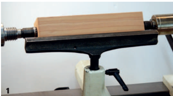
1 Locate centres and mark both ends. Mount between centres on the lathe.
