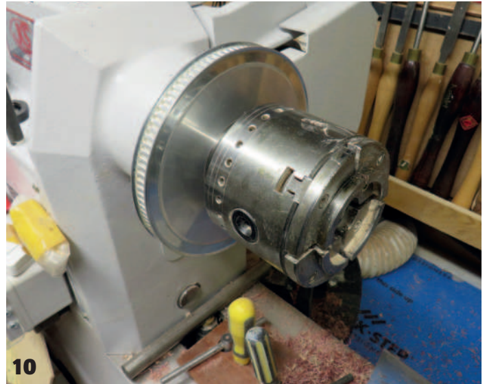
9 Timing wheel bolted on to existing threaded holes in the handwheel 10 Timing wheel sandwiched between the base of the headstock spindle thread and the chuck
