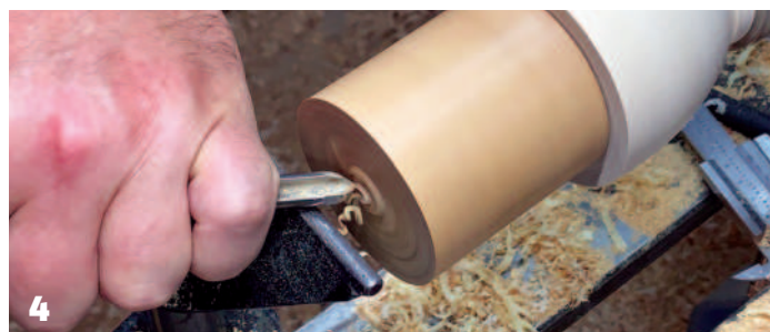
1 About to part the lid from the box, the tenon is roughly cut 2 Transferring the size of the tenon with Vernier callipers, ensuring only the left leg touches the wood 3 With the lid jammed onto the base it can be shaped 4 Using a jam chuck to finish the base
