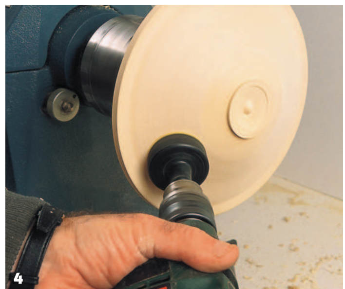
3 Sanding in the safe area – faceplate work 4 Power-sanding the outside of the bowl
