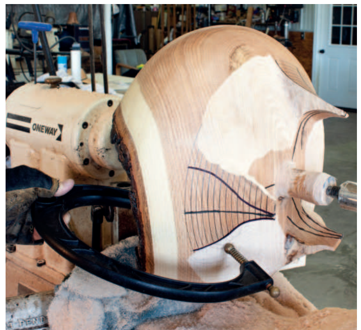
15. Angle grinder position shown with lathe stationary. NB: When in use both hands must be used to control the grinder
