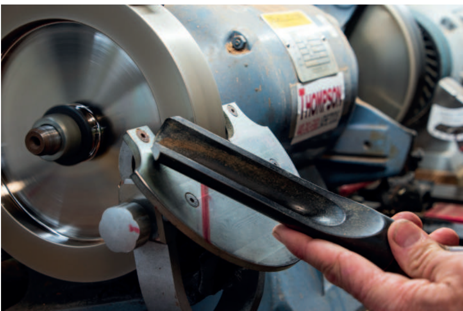
Spindle roughing gouge at the grinder
