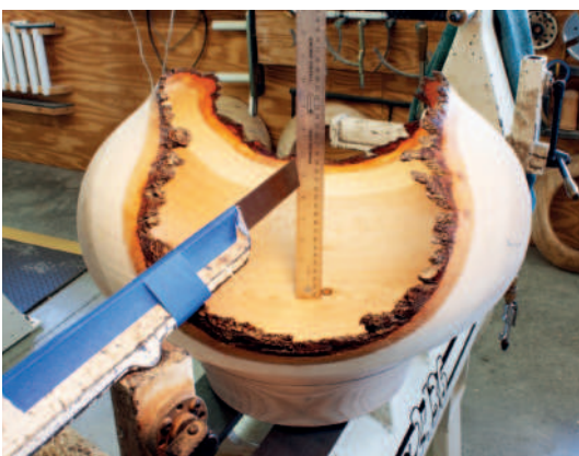
7. Measuring the depth of the bowl
