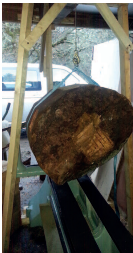
I had to build a winch to mount the piece of wood on to the lathe
