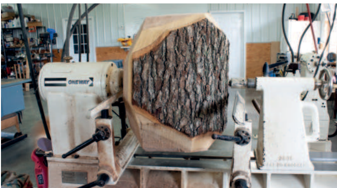
3. Blank mounted on lathe
