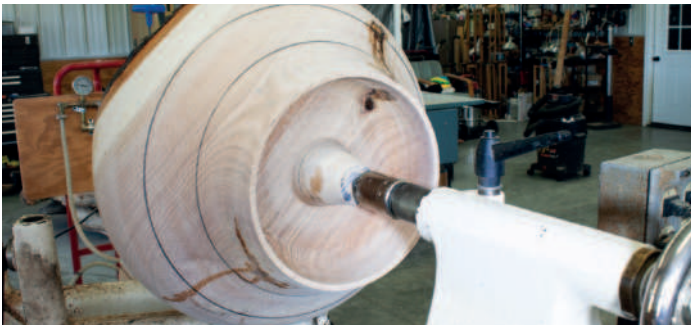
10. Underside hollowing completed
