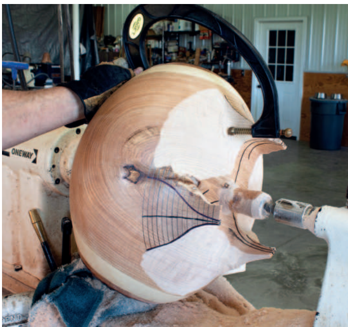
16 & 17. Using a gauge to ascertain thickness
