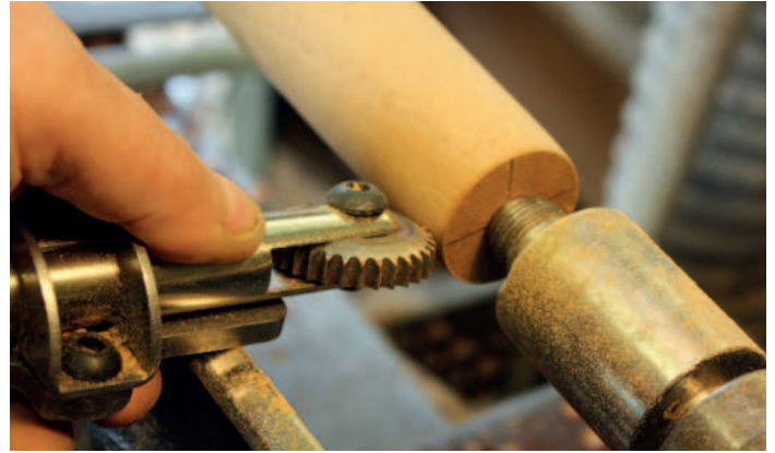
Setting the cutter position
