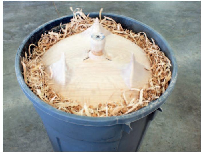
19. Bowl placed in bin of shavings to provide support for nub removal
