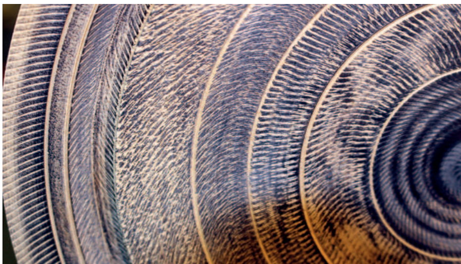
A range of different textures made with the same cutter
