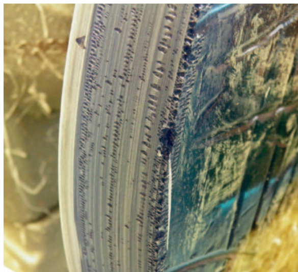
Badly chipped resin caused by cutting too heavily
