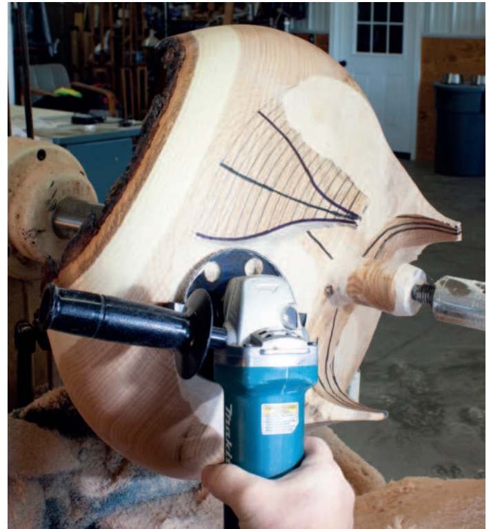
15. Angle grinder position shown with lathe stationary. NB: When in use both hands must be used to control the grinder
