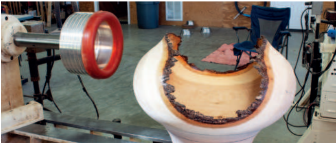
9. Vacuum chuck system installed and ready to mount bowl
