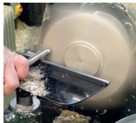
Using a shearing cut with my bowl gouge to produce the outer shape
