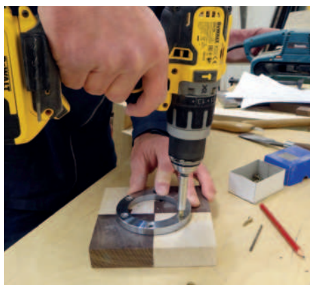
Fixing the faceplate ring for initial mounting
