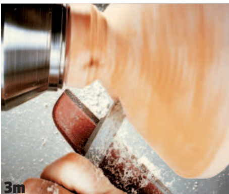
3m If cut E has not produced a good finish, shear-scraping from base to rim will rectify the problem
