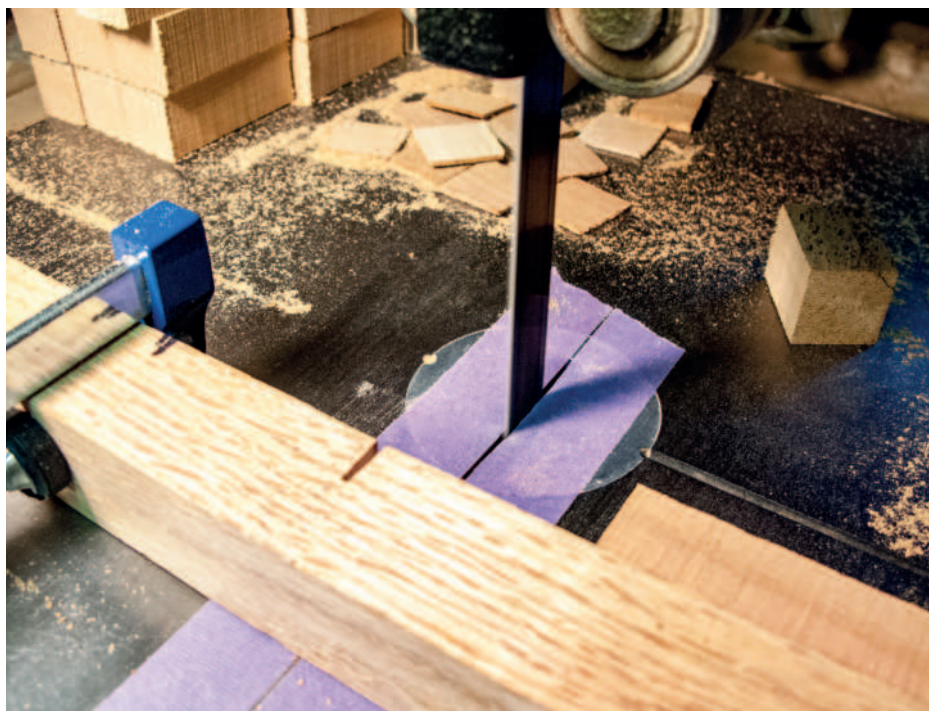
Jigs and fixtures can be as simple as setting a proper length cut off clamp on the bandsaw. Set it for minimal excess needed for barrel trimming, and yet a non-turner can process blanks
