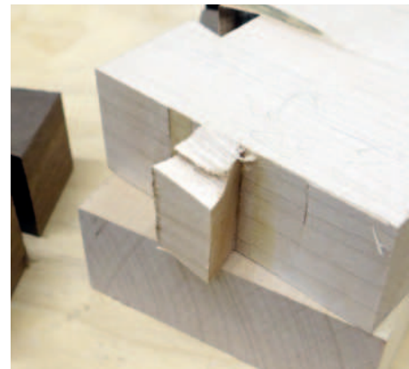
One of the sycamore tails has a chip, but it shouldn't be a problem
