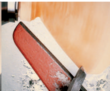
3m If cut E has not produced a good finish, shear-scraping from base to rim will rectify the problem
