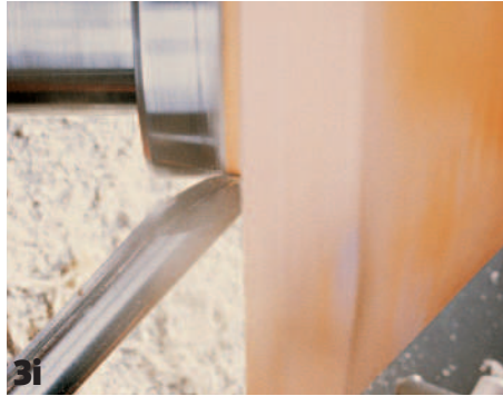
3i Cut D, facing off the upper surface of the bowl, completes the first chucking
