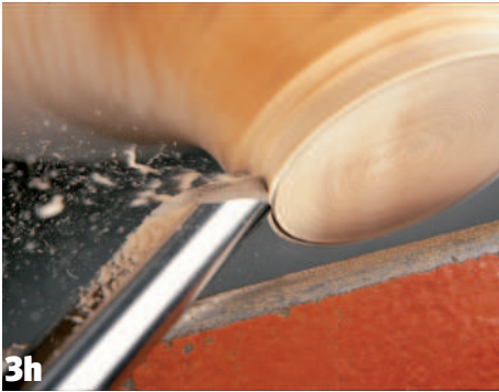
3h Forming the dovetail spigot (cut C)
