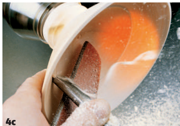
4c A late stage of the hollowing sequence, showing use of fingers to support the bowl (you may prefer to use a glove) and light shining through the bowl wall as a guide to
