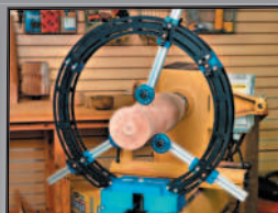
MULTIREST® Vessel Support System
