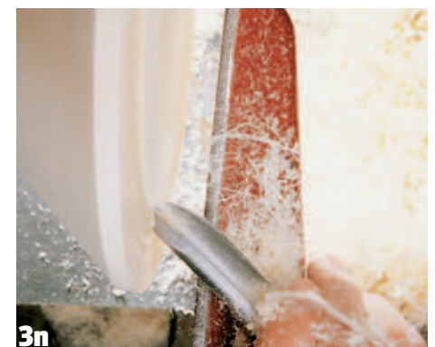
3n Truing the top surface (cut F)
