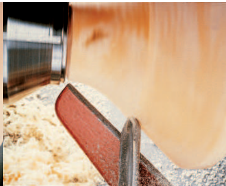
3l A careful cut from rim to base (cut E) should be enough to true the outside
