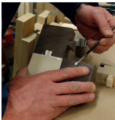
Gluing up the joints
