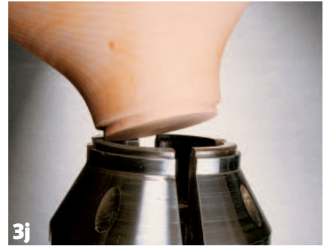
3j Reverse-chucking: mounting the dovetail spigot in the O'Donnell jaws
