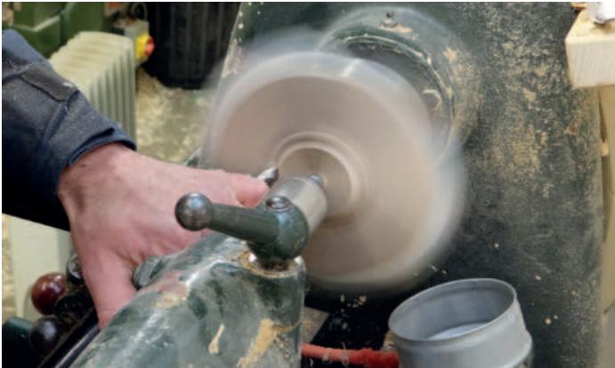
Turning the chucking tenon into a small foot
