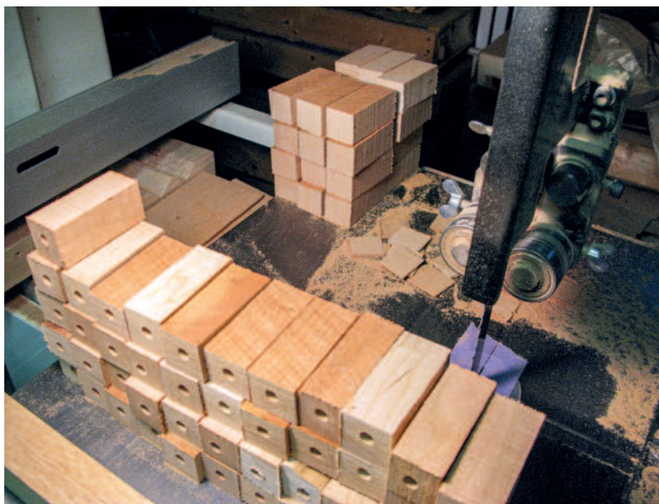
Set up your process to work in efficient sized batches. You don't need all 250 blanks sitting in a pile waiting for turning. Only enough to keep ahead of the turner. (My prep for upcoming classes)
