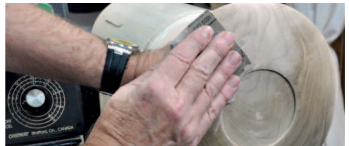
Hand sand to remove radial scratches
