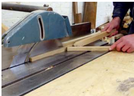
Ripping the 1mm strips
