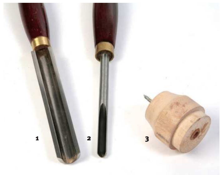
1 ¾in (19mm) spindle roughing gouge 2 ⅜in (10mm) spindle gouge 3 homemade screw chuck
