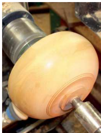
Abrading the first coat
