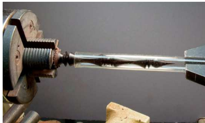
If you aren't comfortable 'catching' your finial as you part it off, use this trick to safely enclose and catch your prize as you separate it
