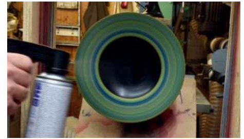
Spraying lacquer: applying lacquer while work is on the lathe
