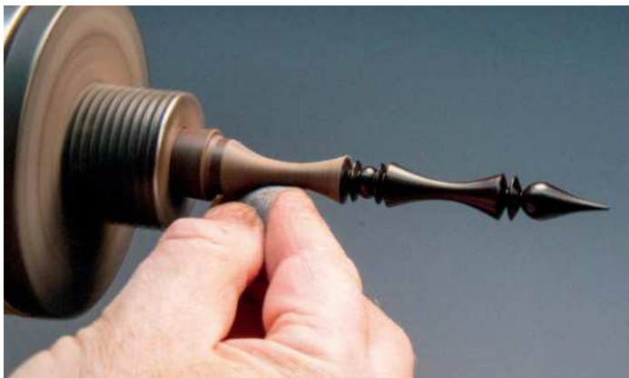
Like the very thin, long stem goblet shaft, you work in sections completely finishing each short section and then moving on to the left
