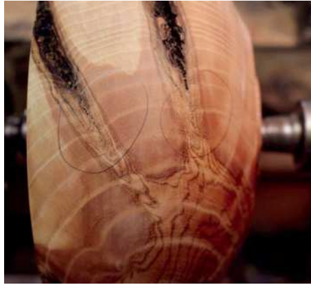
Cracks caused by the burr and inclusions
