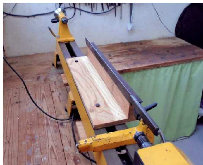
The homemade toolrest can be bolted through your lathe bed with long bolts
