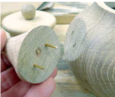
Brass rods used to fit the spout to the pot
