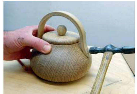
Tapping the fixing rod in place
