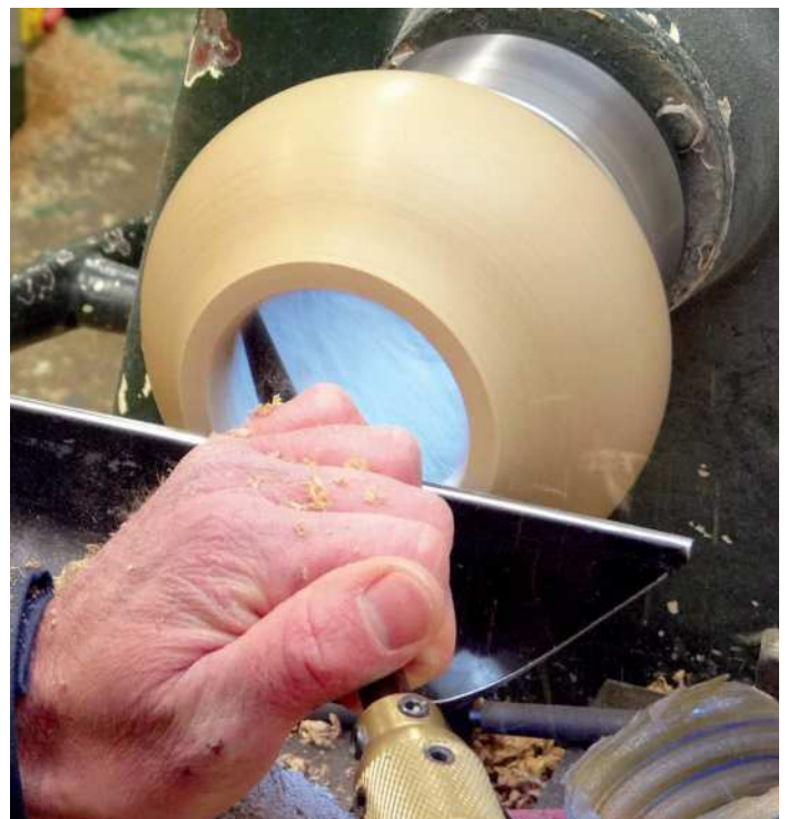
Working deeper with the carbide probe
