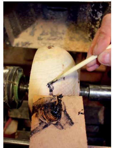
Applying the filler
