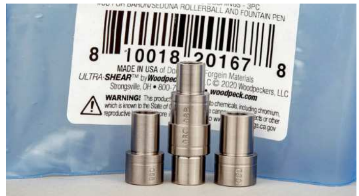
Each package of bushings indicates the kits that the bushings are designed for. Notice the C(ap) and B(arrel) markings added to the bushing numbers to indicate orientation
