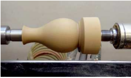
The first stage of turning the spout looks like a bottle
