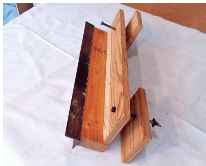
You can easily and cheaply make a long toolrest to fit your lathe
