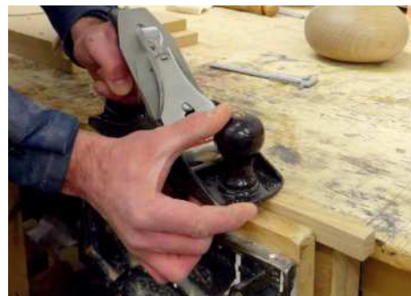
Plane between rips to ensure the smoothest surface
