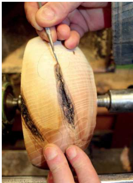
Widening and cleaning the cracks
