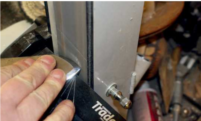
Touching up a negative-rake scraper
