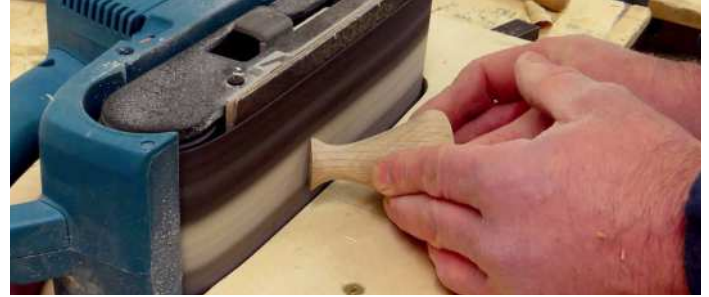
Shaping the spout on the sander
