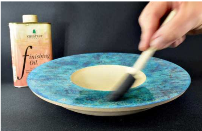
Oil on: adding oil to stained rim with a foam brush
