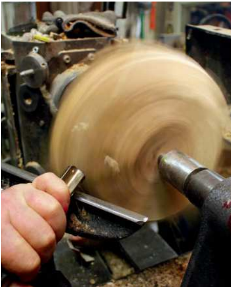
Using a large bowl gouge to rough down
