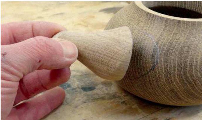
Marking the position of the spout
