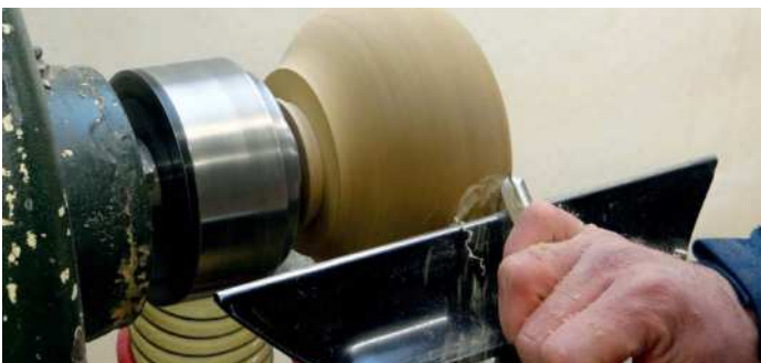
Shear cutting to refine the surface of the teapot
