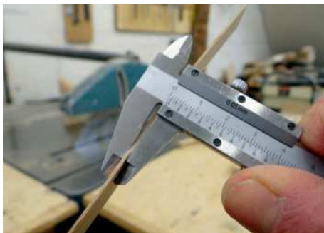
Each layer is exactly 1mm thick
