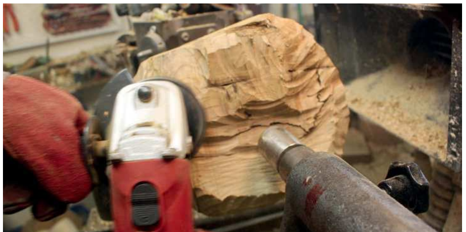
Roughing down with the spindle locked
