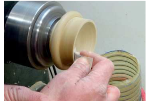
Sanding the underside of the lid
