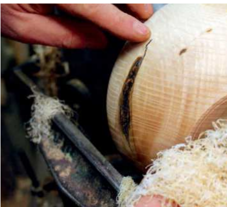
Checking the infill after a pass with a negative-rake tool
