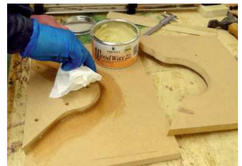
Waxing the former to prevent sticking
