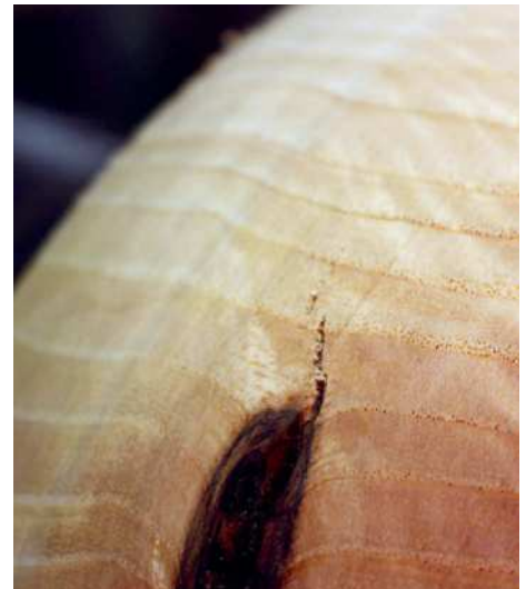
Small fractures at the end of the inclusion
