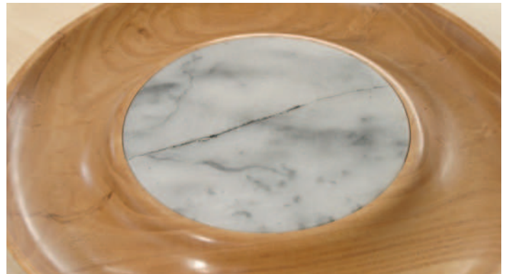
Movement in poorly dried wood caused marble insert to crack under movement forces
