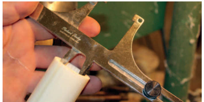
Using a Sorby chasing gauge to determine the tenon size
