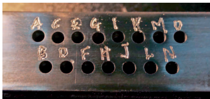
20: Holes drilled and labelled in the vee-pocket shaft
