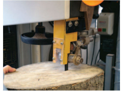
Converting a section of log into a blank
