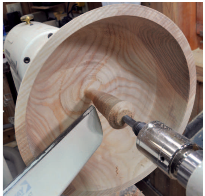
Deep hollowing with tailstock support
