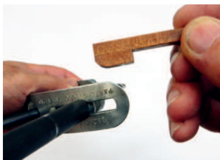
13: Setting the Vari-Grind 2 angle arm with the gauge
