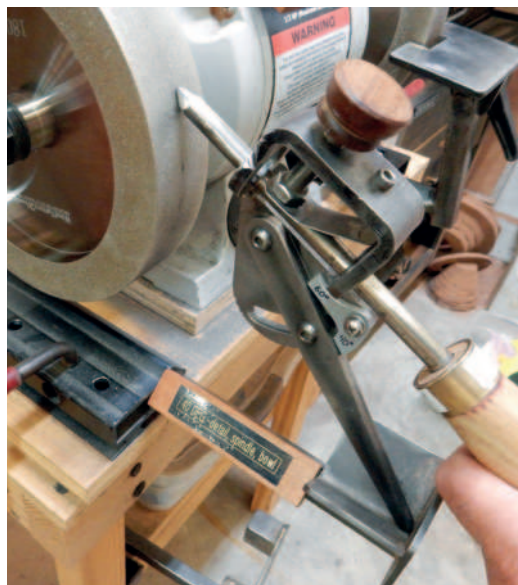
7: Setting the vee-pocket position with a gauge stick
