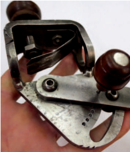
Setting the original Vari-Grind angle arm position
