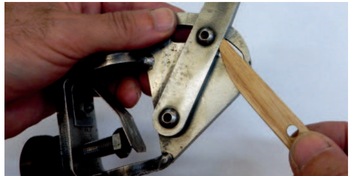
4: Using the gauge to set the angle arm
