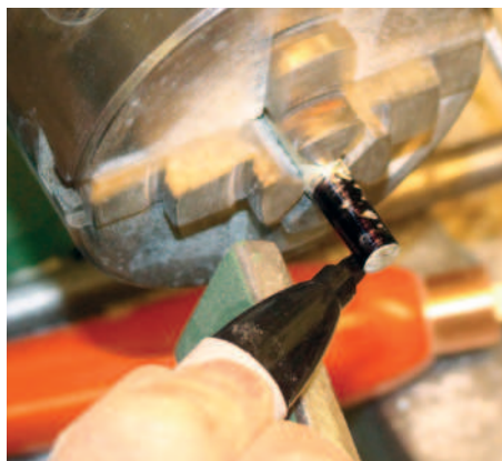
Blacking the rod for marking out
