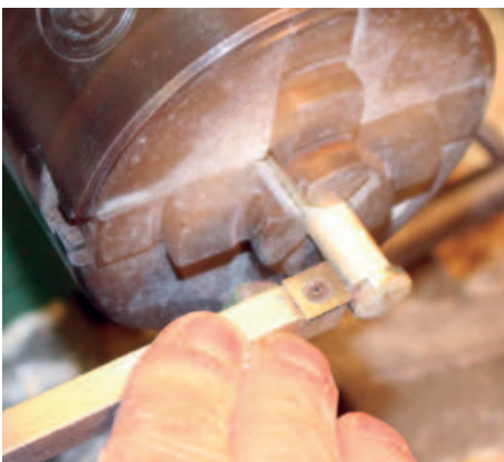
Roughing down the cast rod with a carbide tool
