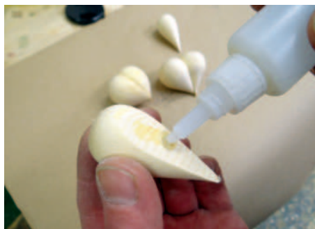
The prototypes are joined with CA
