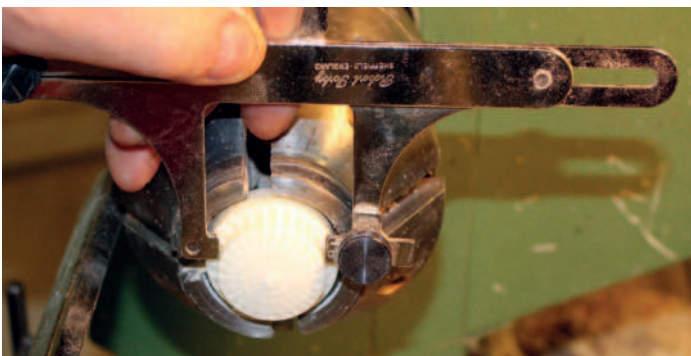
Checking the tenon size
