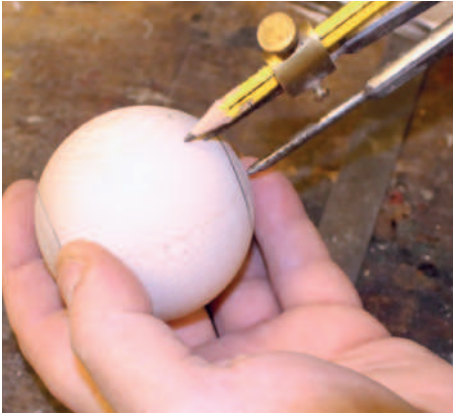
Marking to find the mid-point
