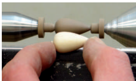
Matching the tiny teardrops to ensure accuracy
