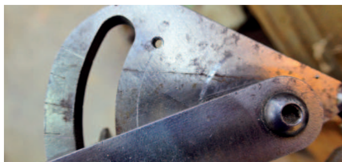
18: Line scored along the path of angle arm. Here's the process to modify the Vari-Grind jig:
