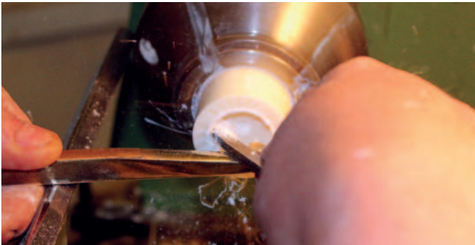
Cutting a relief slot at the base of the recess
