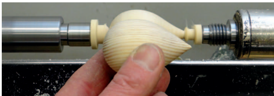
Using the first teardrop to check the shape of the second
