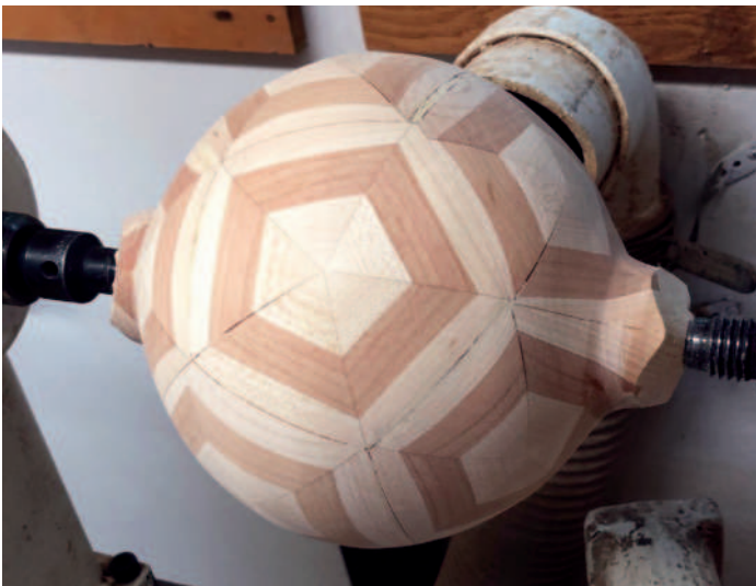
First-stage turning completed
