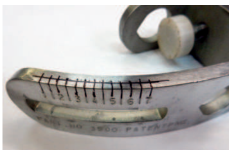
21: Layout for holes to be drilled into the V2 RIGHT: 22: Drilling holes in V2 for arm position pin at full and half intervals stamped on jig
