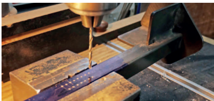
19: Drilling the gauging holes in the vee-pocket shaft
