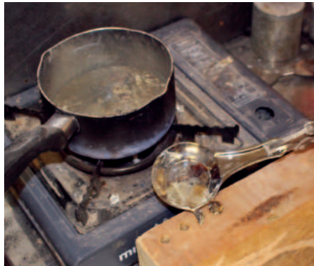
Pouring the molten pewter into the cast
