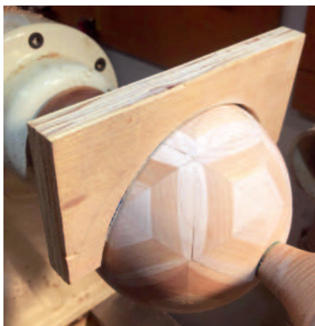
Testing the abrading jig for fit
