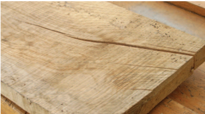
Board with severe cracks from drying
