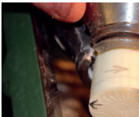
Marking the misalignment
