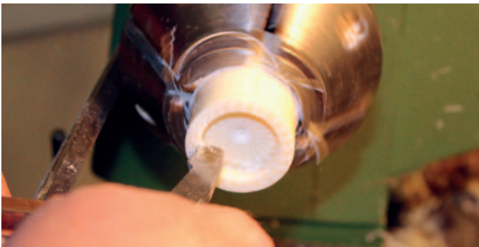
Starting to chase the internal thread
