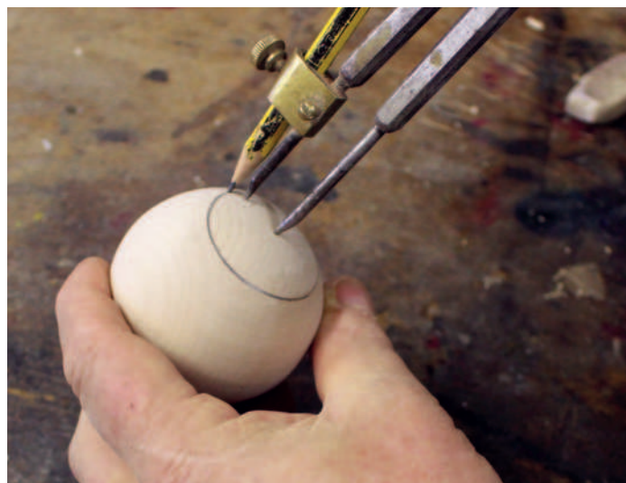
Marking the poles
