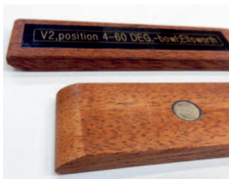
10: Reverse side of spacer gauge showing magnet and chamfer for weld clearance
