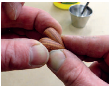
Gluing the hearts together using a rub joint and finger pressure
