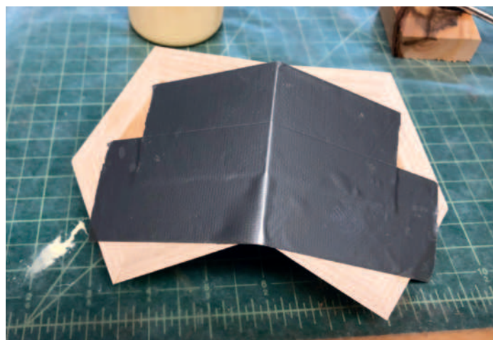
Two pentagons taped for gluing
