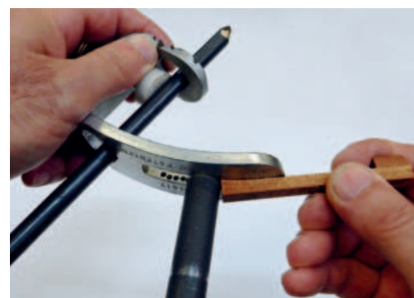
14: Setting the Vari-Grind 2 angle arm with the gauge
