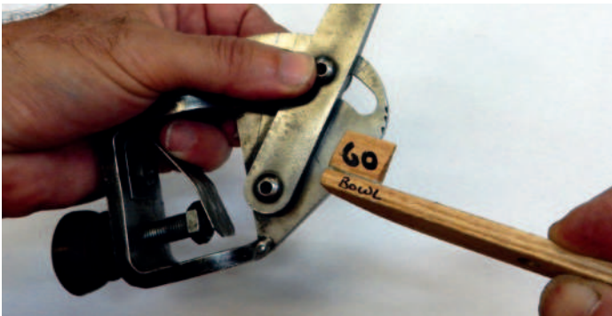
3: Setting the angle arm with the gauge
