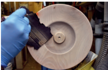
A piece of torn card being used as a template
