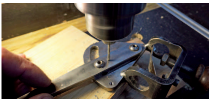
17: Drilling first hole in Vari-Grind jig
