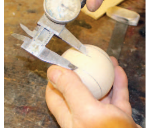
Marking the centre line
