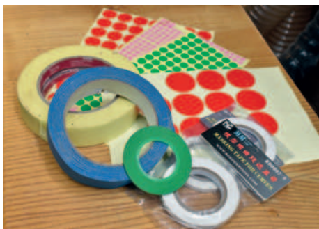
Tapes and stickers used for simple masking
