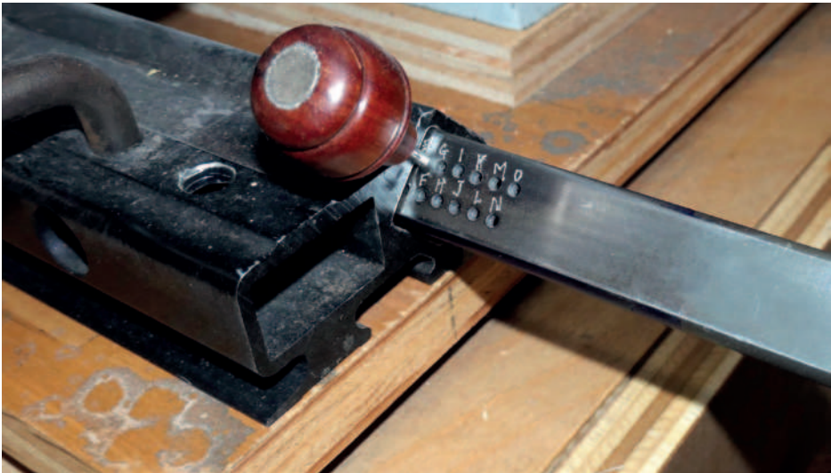
Setting the vee-pocket arm or the pivot arm position
