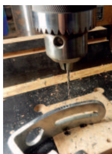
21: Layout for holes to be drilled into the V2 RIGHT: 22: Drilling holes in V2 for arm position pin at full and half intervals stamped on jig
