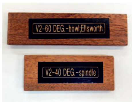
9: V2 pivot arm spacer gauges for two of my favourite grinds
