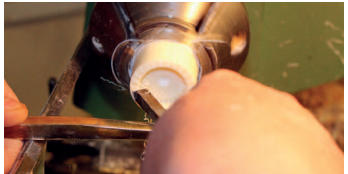
Cutting a chamfer on the lip
