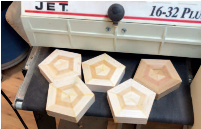
Running the pentagons through the overhead sander
