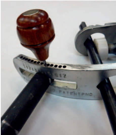
Setting the Veri-Grind 2 angle arm position
