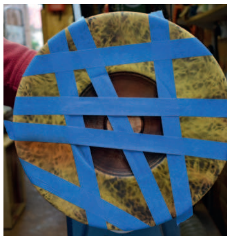
Use painter tape or masking tape to protect the top layer of colour
