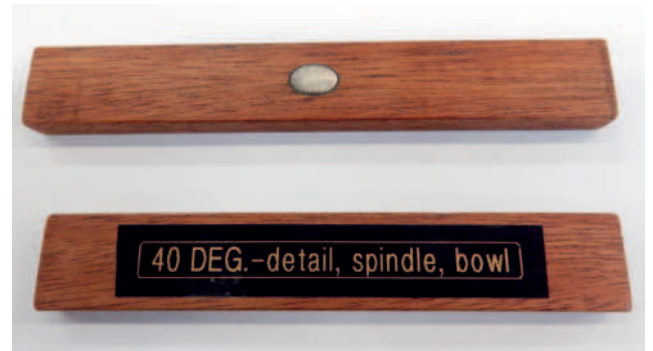
6: Magnet on one side of vee-pocket spacer
