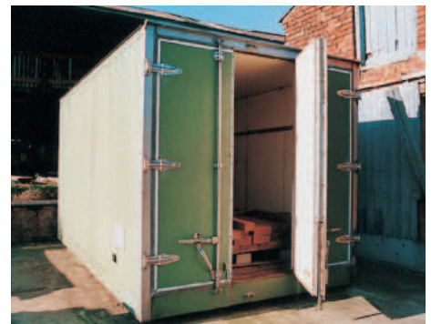
Repurposed refrigerated truck body kiln
