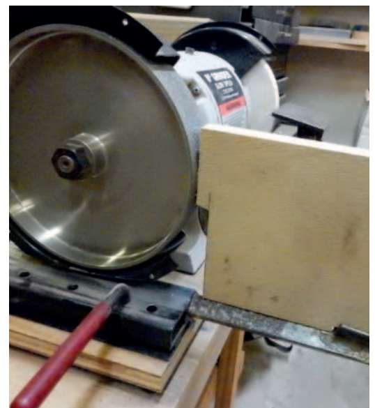
8: Setting the vee-pocket position with a wood block when using an aluminium oxide wheel (shown on a CBN wheel)
