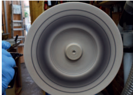
Wider, less saturated and defined lines are achieved just by moving the airbrush further back from the wood
