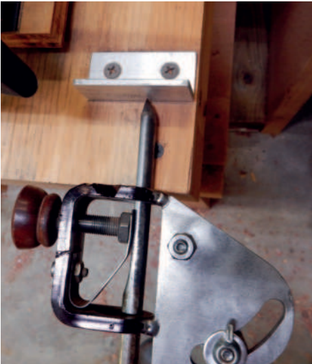
Stop block to set 1 3/4in (45mm) protrusion of the gouge beyond the Vari-Grind
