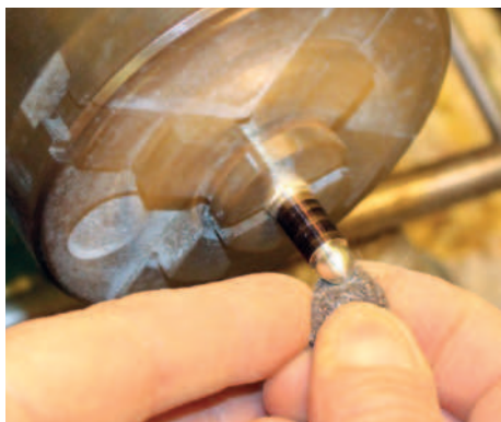
Abrading with a pad of 0000 wire wool
