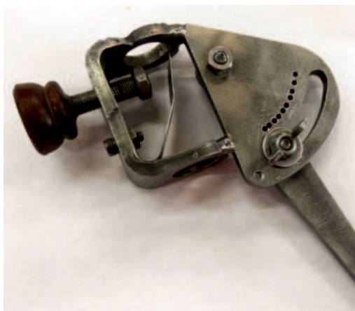
15: Holes drilled in Vari-Grind jig
