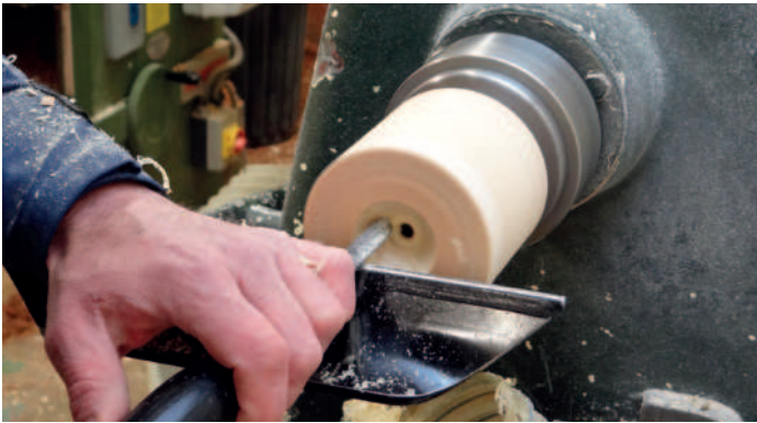
Beginning to hollow the securing ring
