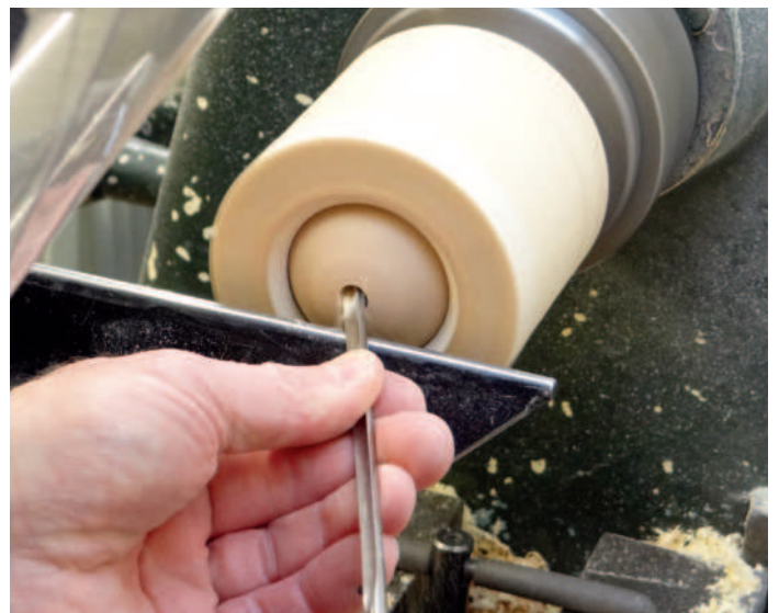
Enlarging the hole with my 6mm spindle gouge
