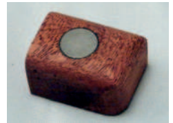
Block of wood with a magnet used for the two facet relief bevel
