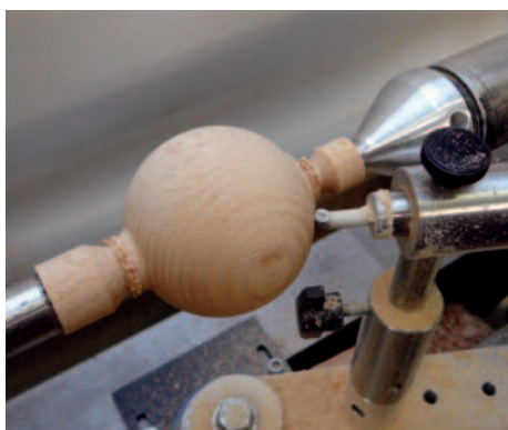
The sphere jig can't get right round the ball
