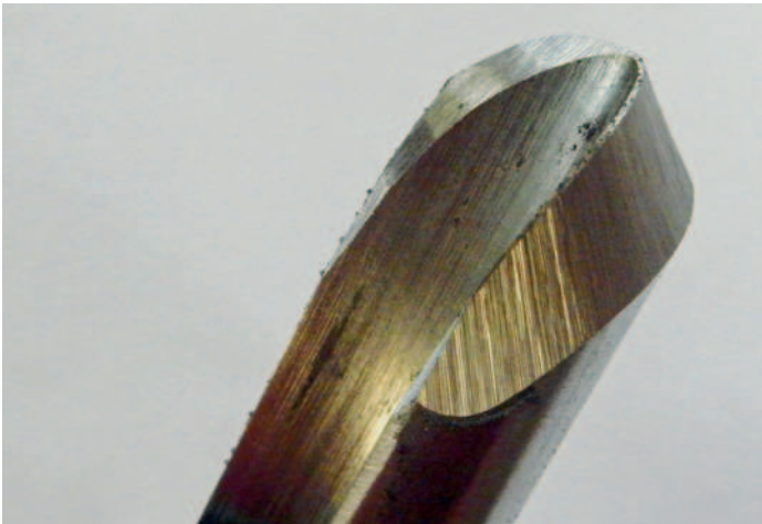
One side ground to proper shape; one to go
