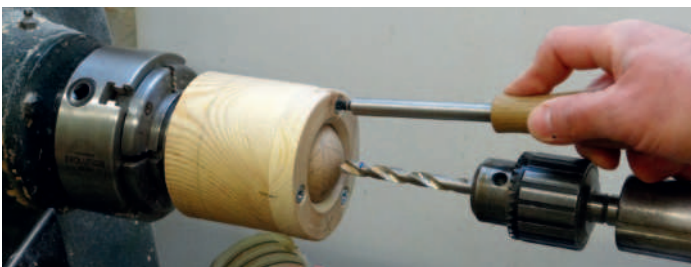
Securing the sphere in the jig
