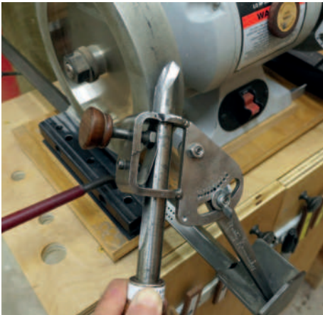
Grinding the side bevel on the fine wheel
