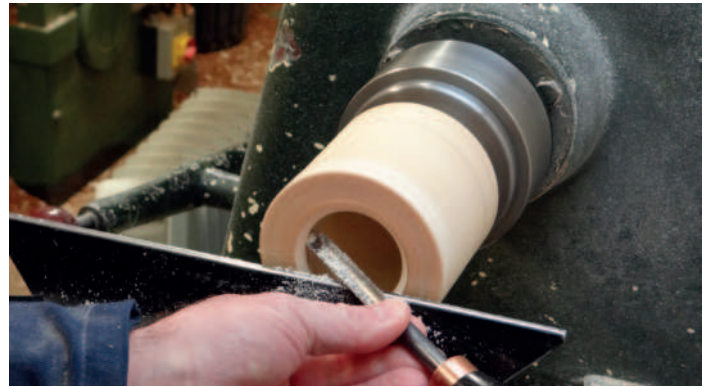
Relieving the underside of the ring to hold the sphere in place
