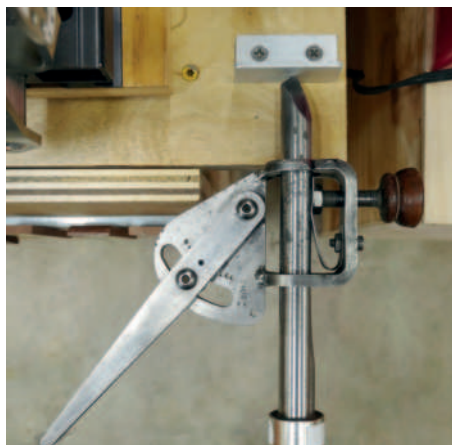
Setting protrusion length. Stop block to set Vari-Grind at 1\frac{3}{4} inches (45mm)
