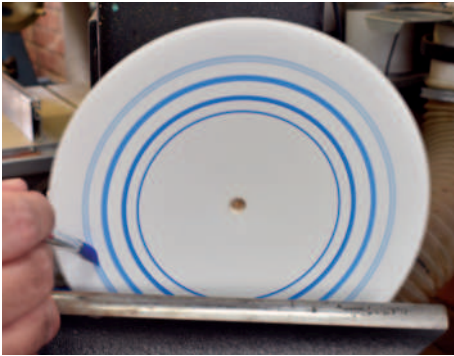
Metallic blue paint being added while the lathe spins at low speed
