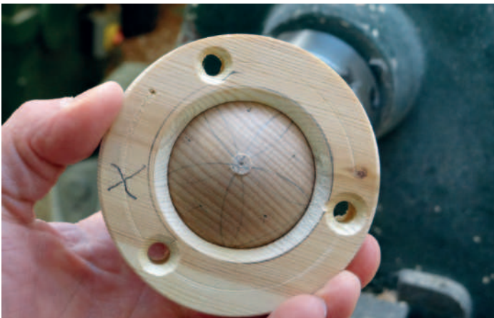
Testing the fit of the securing ring
