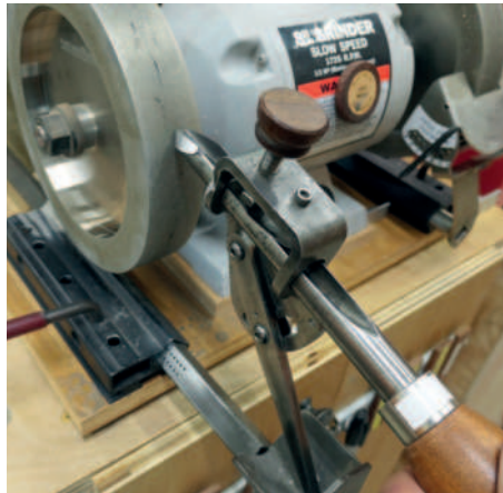
Swinging the tool to grind the nose
