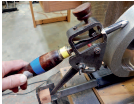
Grinding the relief with the block in the \frac{1}{2} in orientation
