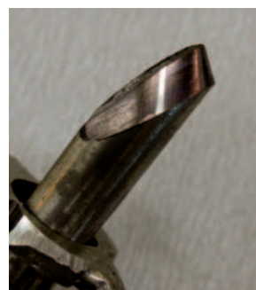
Top to bottom scratch on side bevel
