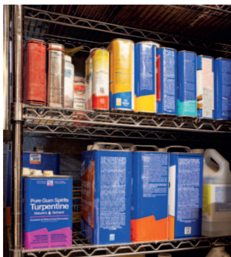
In my shop, all of my chemicals except for the working transfer containers, are stored in one place. They are tightly capped, stored in the original containers, and off the floor
