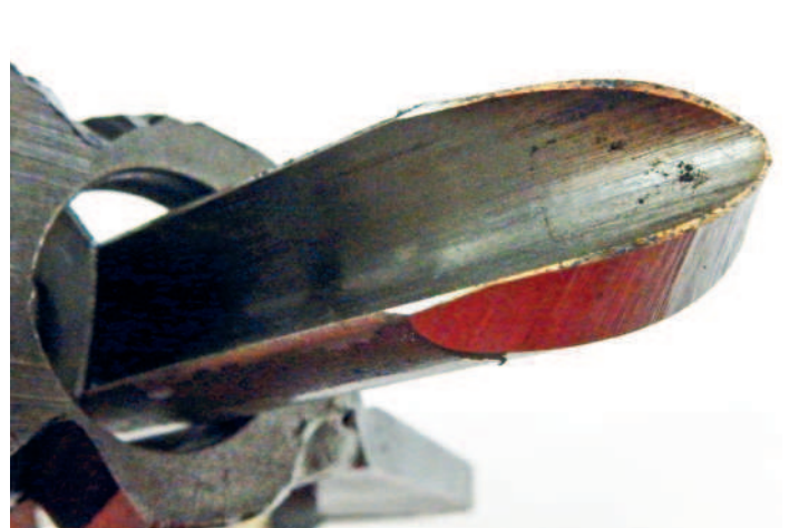
Both sides ground to proper shape but still a bit of flat on the edge
