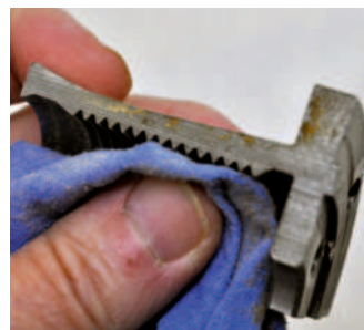
Clean all the debris off the jaws and dig out debris from screws before removing
