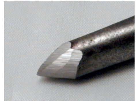
Grind a second bevel
