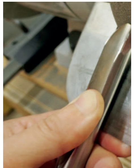
Grinding the nose angle
