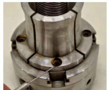
Clean all the debris off the jaws and dig out debris from screws before removing
