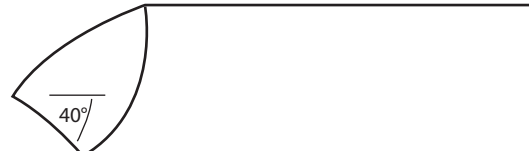
Bowl gouge with short wings ground with a 180 grit CBN wheel
