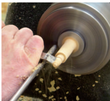
Turning the point of the spike
