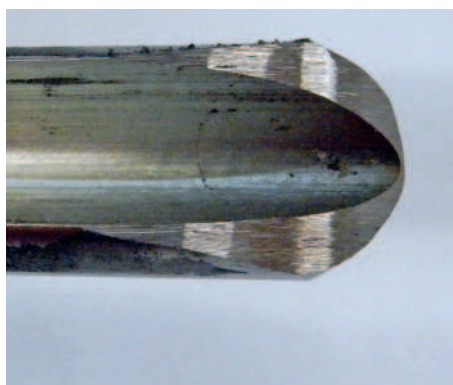
Corners ground off
