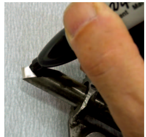
Painting the bevel with an indelible marker
