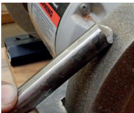
Grinding the corners off; flute facing the wheel
