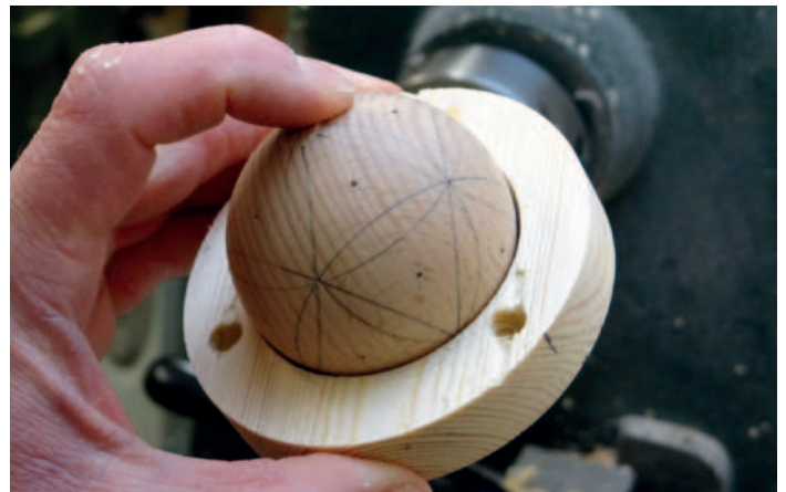
Testing the fit of the securing ring
