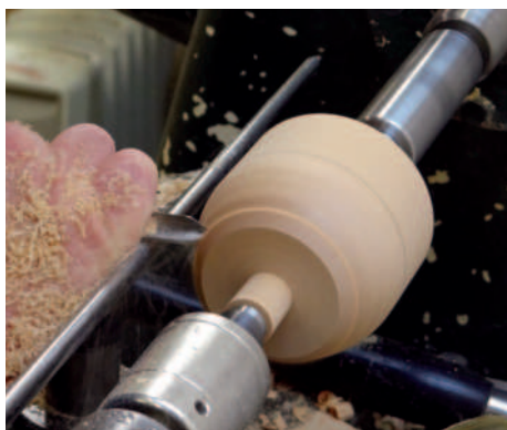
Turning a ball freehand
