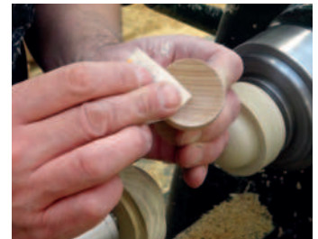
Sanding the sharp edges of the cups
