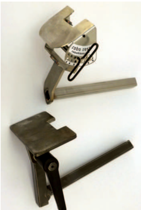
Lower unit is original Wolverine platform with a notch that I cut; upper unit is a Robo Hippy platform that fits the Wolverine system
