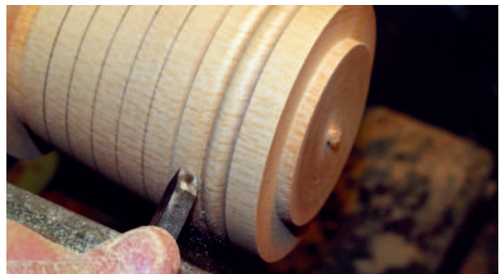
Forming a bead with a parting and beading tool
