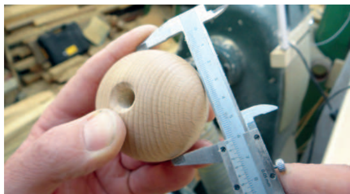
Checking the size of the finished tama
