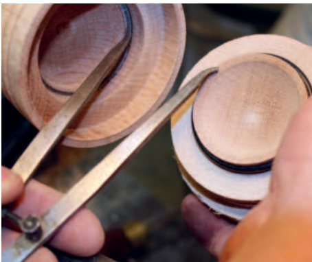
These two surfaces must mate
