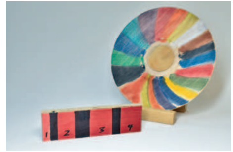
Stains and dyes test sample on wood. Notice how subsequent coats of red intensify the colour but still allow the grain to be seen
