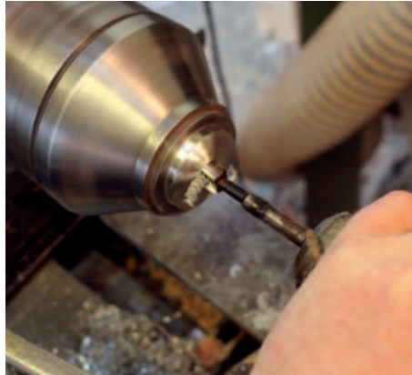
Drilling for the finial
