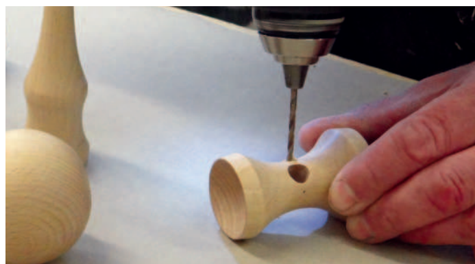
Drilling the sarado
