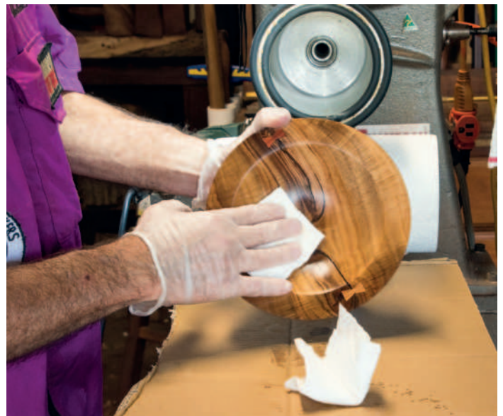
Using wadded clean paper towel to spread the CA
