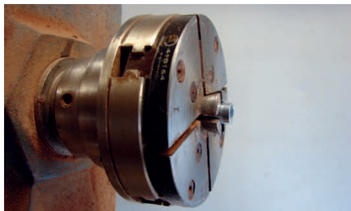
Spare internally threaded tube used for mounting hold
