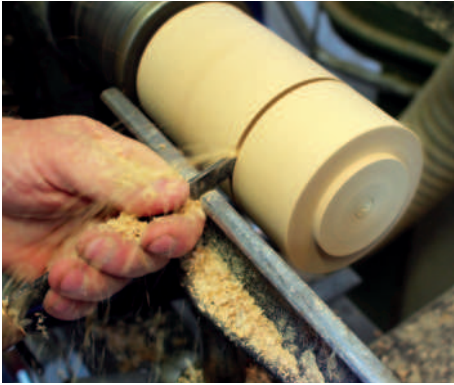
Parting off the lid section
