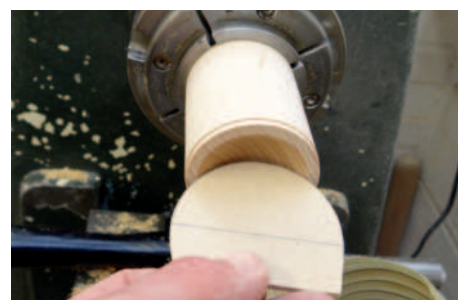
Checking the cup is deeper than the ball with a template
