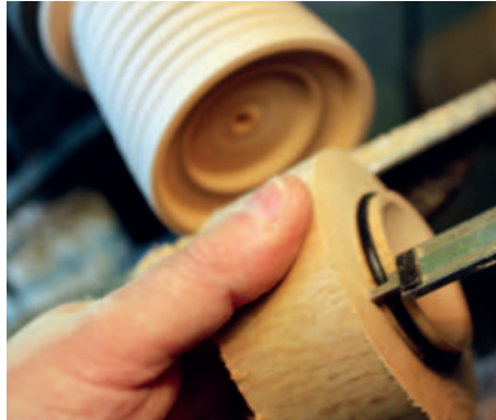
Measuring the depth of the sealing tenon
