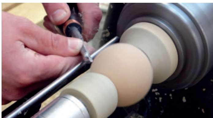
Correcting the shape between wooden cups
