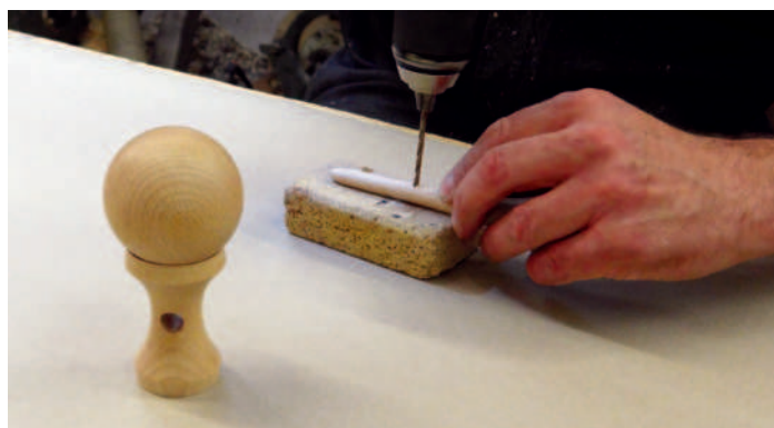
Drilling the ken
