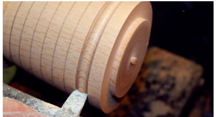
Turning a bead with a dedicated tool
