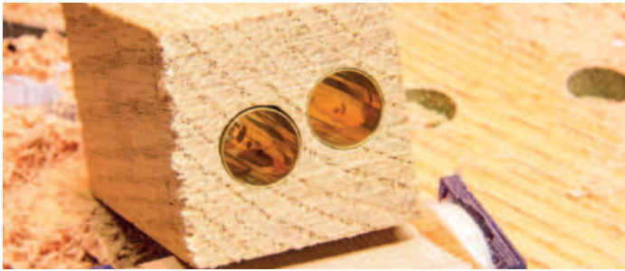
Regardless of the kit spellout, pick the drill sizes you want based on your desired clearances for your selected adhesive
