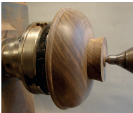
Base screwed on ready for turning
