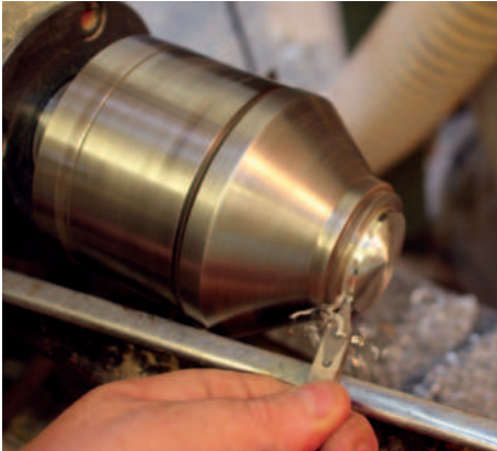
Cutting a chamfer
