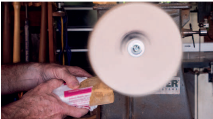
Loading the mop with compound
