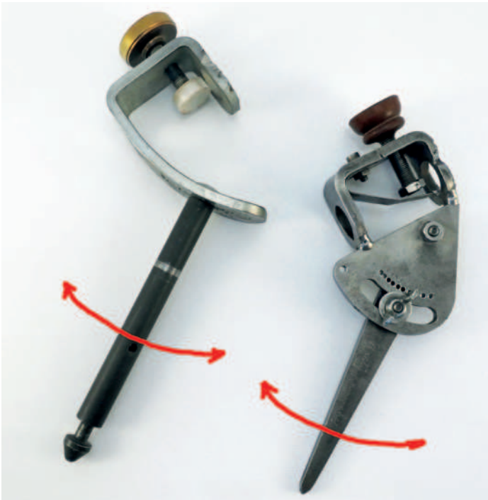
Left: Vari-Grind 2 jig; Right: original Vari-Grind; red lines indicate travel of the angle arm
