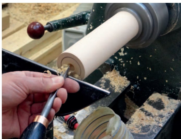
Beginning to turn the base cup in the ken
