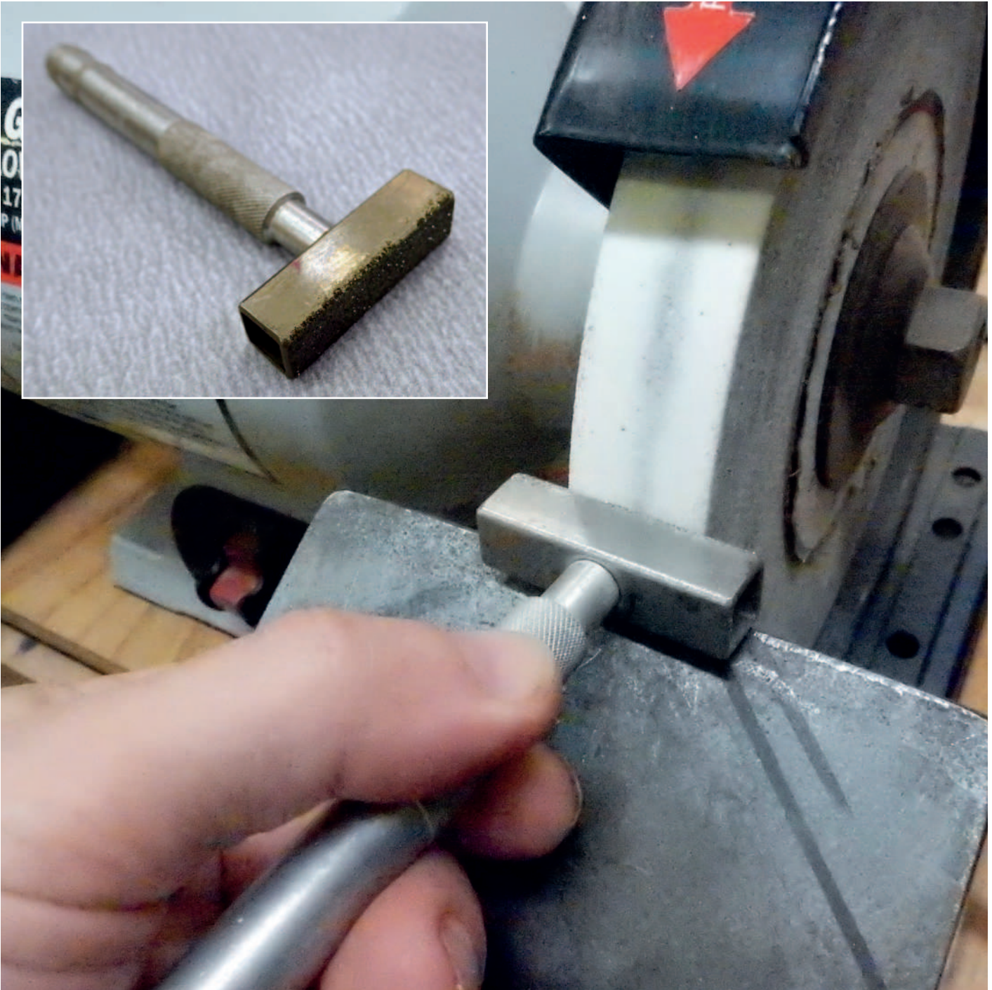
Diamond wheel dresser, cleaning and flattening aluminium oxide wheel. A diamond wheel dresser (use either a cluster diamond or point diamond; don't use a star dresser) is used to clean, true, and flatten stone wheels. It's never used for CBN wheels
