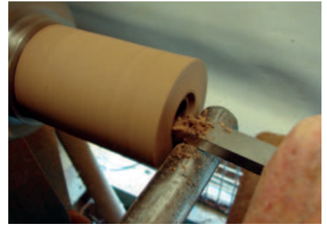
Shaping the hole
