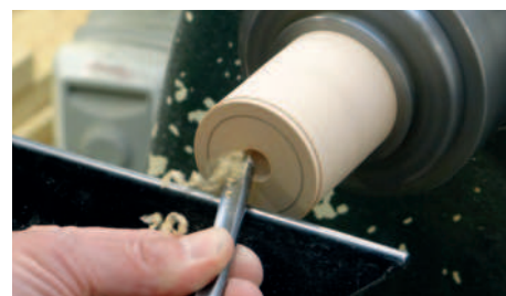
Beginning to turn the cup with a spindle gouge
