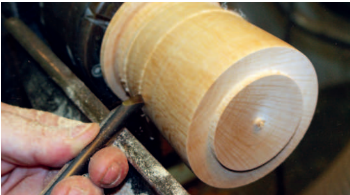
Shaping to the 70mm base diameter
