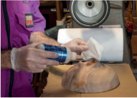
Applying CA to the base
