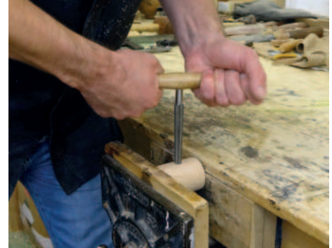
Reaming the hole in the sarado
