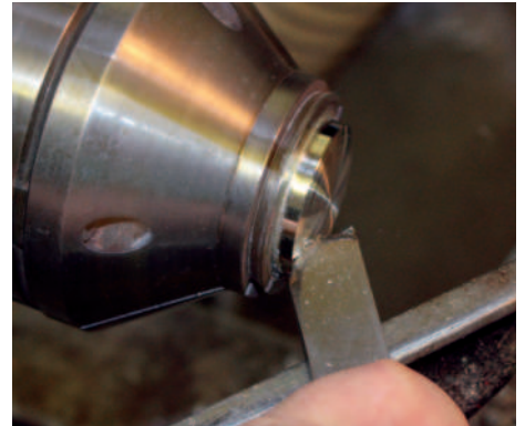
Cutting a convex surface with a negative rake scraper
