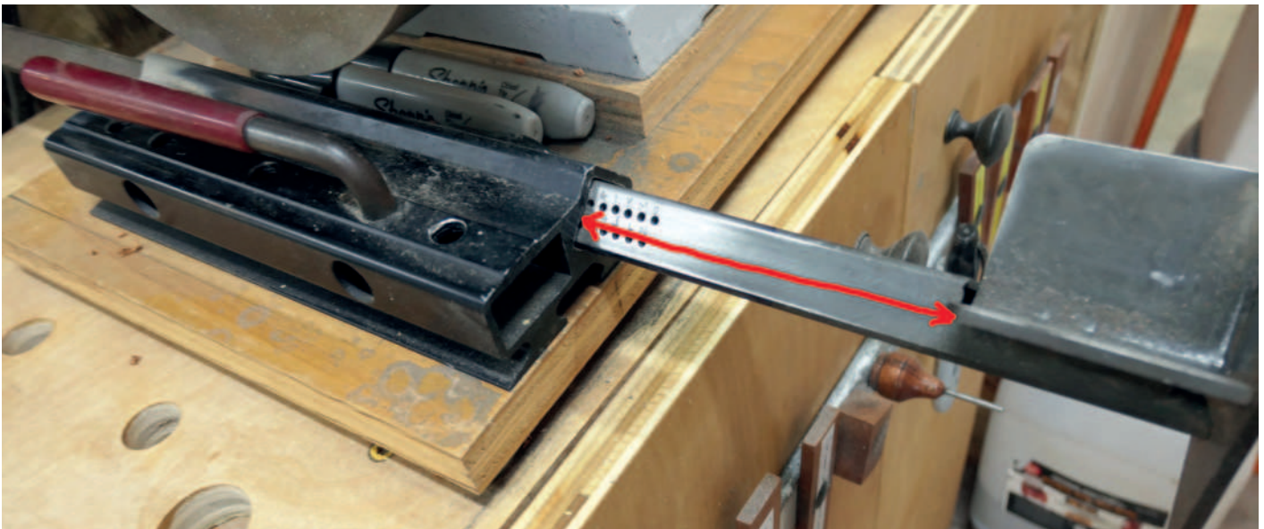
Base unit with vee-pocket; red line indicates vee-pocket extension distance
