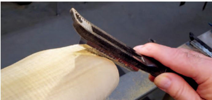
Shaping with microplane
