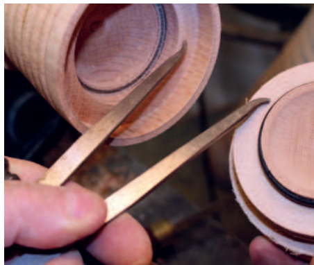
These two surfaces must also mate
