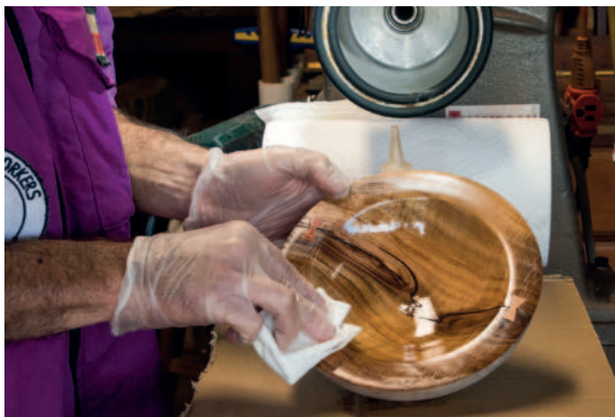
Spreading the Parfix to cover the bowl
