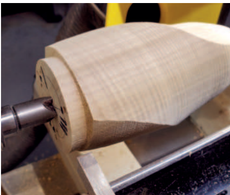
Re-cut the tenon
