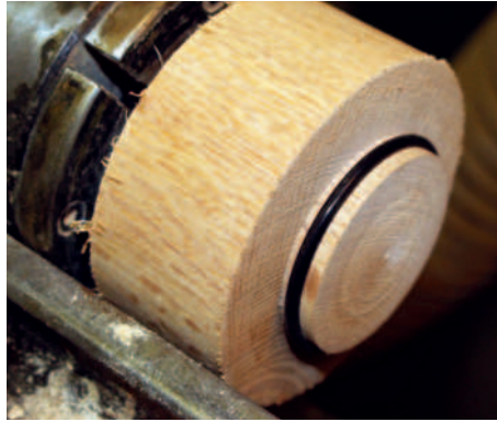
Test-fitting the O ring
