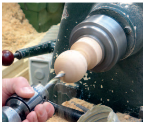
Drilling the hole in the tama
