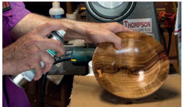
Applying Parfix accelerator
