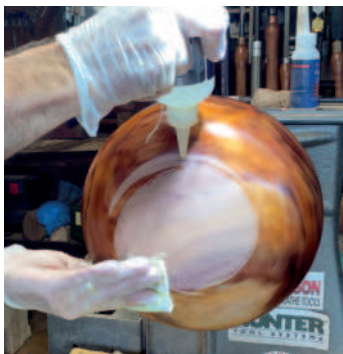
Applying Parfix with the lathe running slowly
