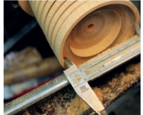
Measuring the primary recess diameter
