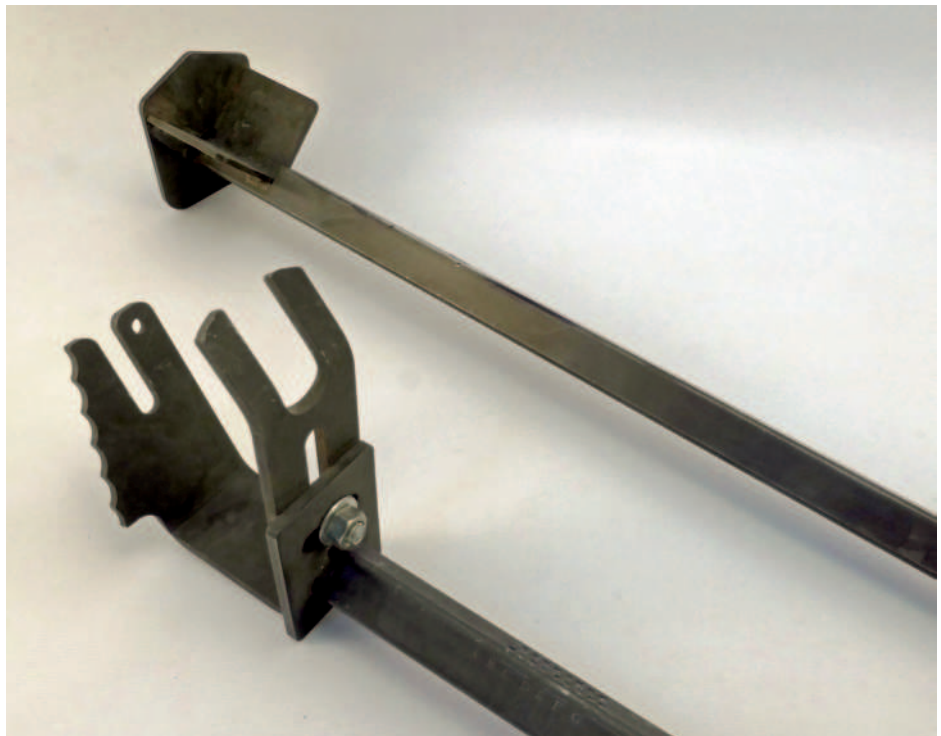
Upper: vee-pocket for original Vari-Grind; lower: Pivot arm for Vari-Grind 2
