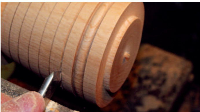
Making a V-cut with the skew
