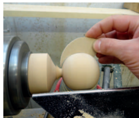
Checking against the template before parting off
