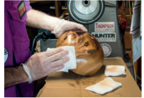
Removing the excess to allow curing
