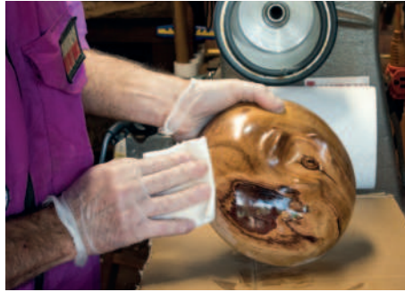
Applying the CA
