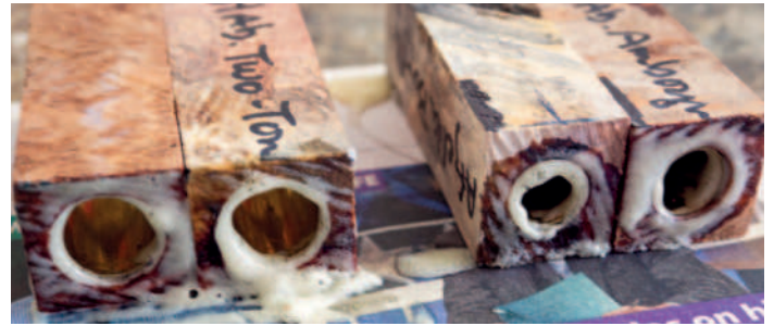
My adhesive of choice is polyurethane, the small gap-filling foaming cure. Its forever pliability eases the wood cladding's life of movement
