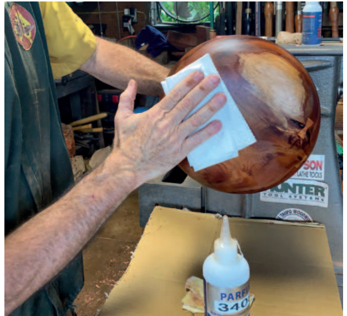
Wiping off the excess CA, in a circular motion, with the bowl on the lathe
