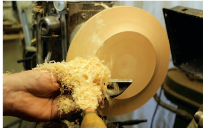
Refining with a negative-rake scraper
