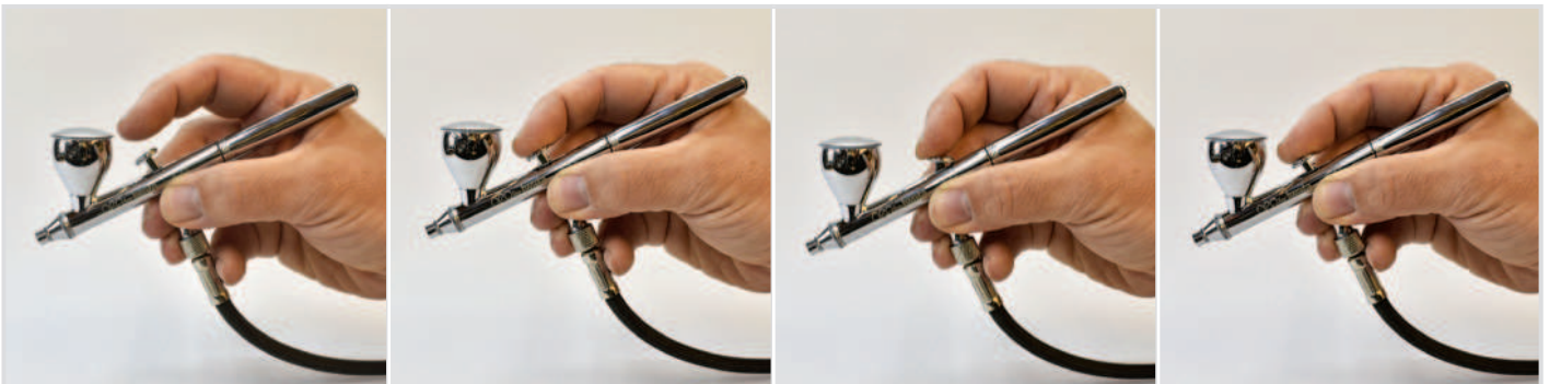
A double-action airbrush: control sequence – from left to right: air/paint off, air on, paint on, paint off
