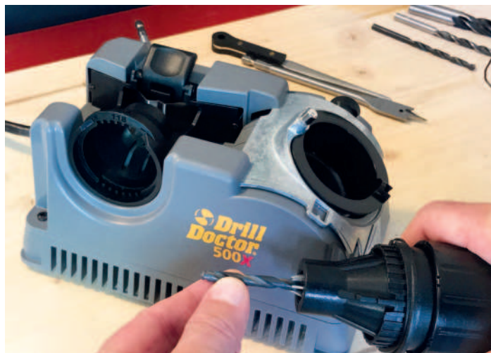
This machine utilises a chuck that holds a twist drill bit in the proper position during the sharpening process
