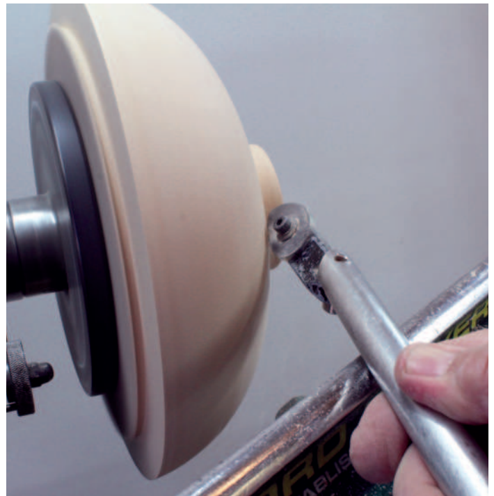
An interchangeable scraper being used as negative rake
