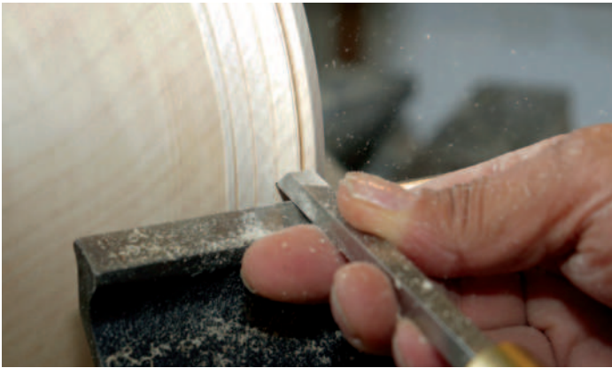
Using the points of a beading tool to create equally spaced V-cuts
