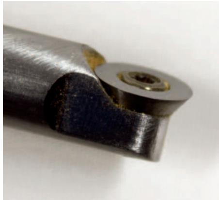
A modern carbide 'cutter'
