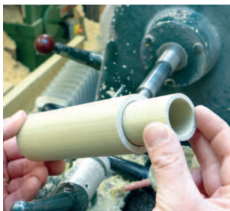
Testing for fit
