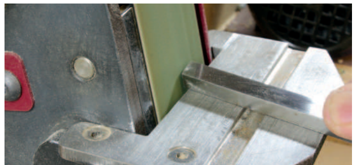
The grinding table set at 80^\circ
