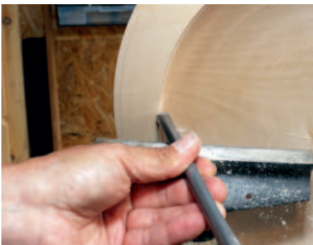
Taking a cut with the flute pointing to 3 o'clock
