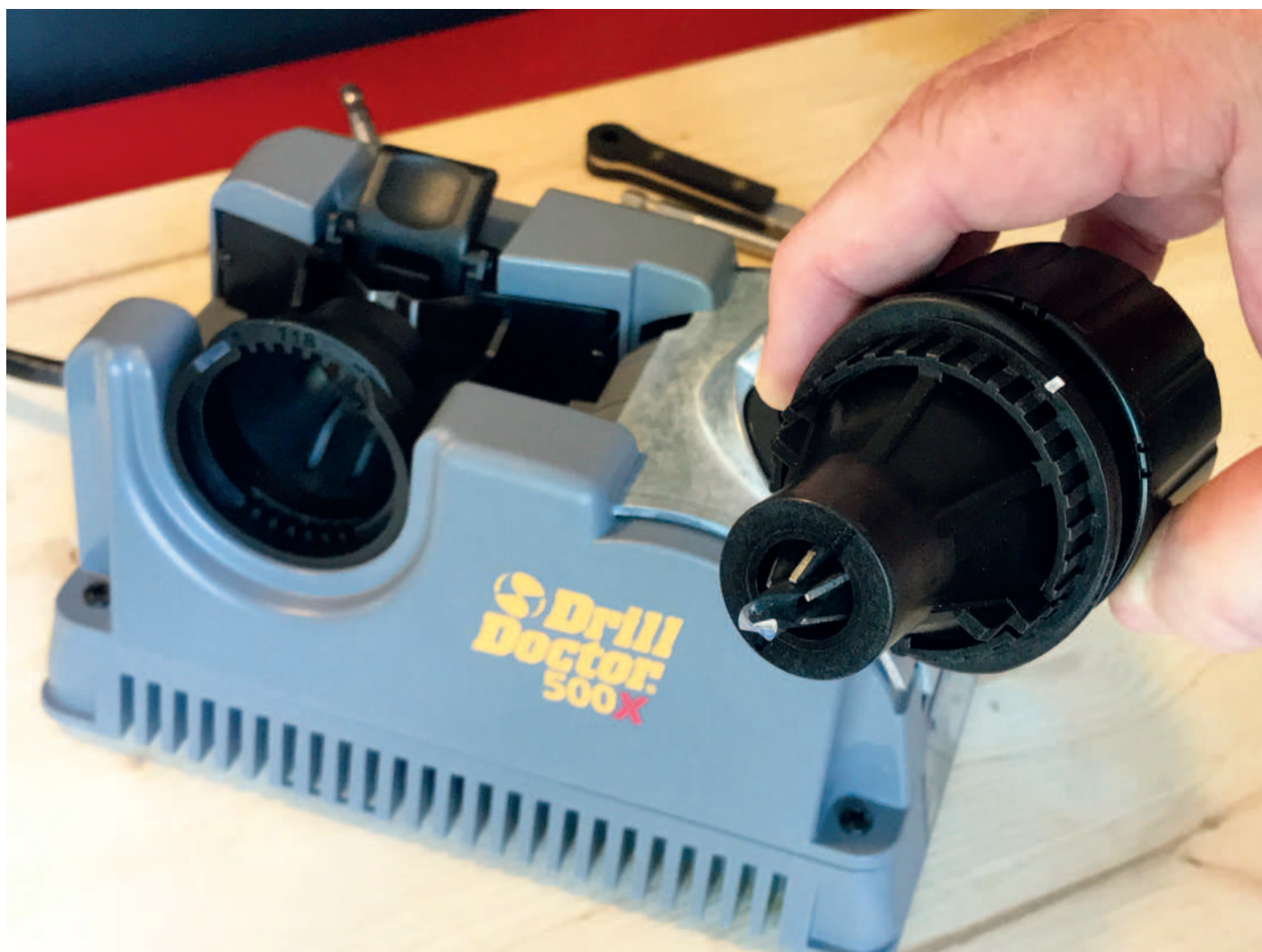
You can sharpen any twist bit in just a few seconds. A drill bit can be sharpened many times before it needs to be replaced
