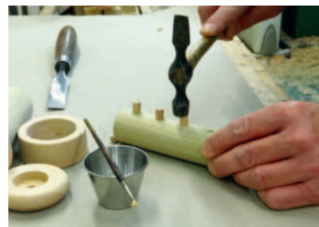
Gluing the dowels in place
