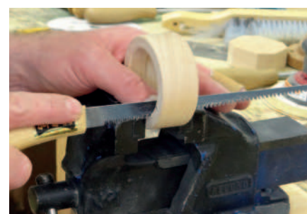
Sawing the notches into the rings
