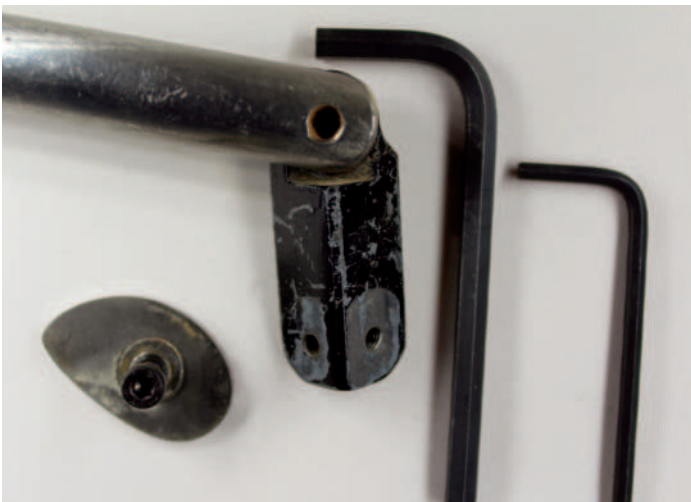
The Munro shear scraper head, offset to one side
