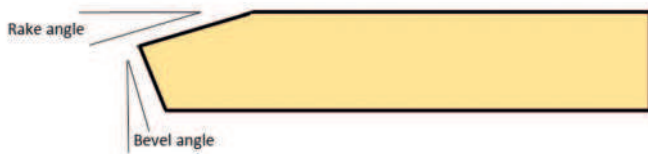
Negative rake grinds can vary considerably
