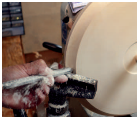
Conventional round-nose scraper in trailing mode
