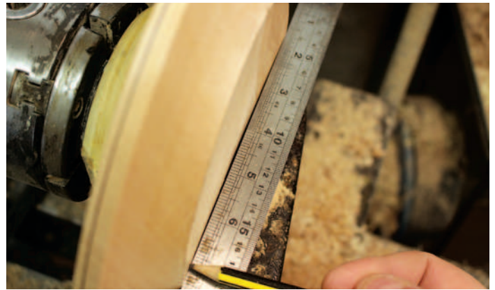
Checking the hollow
