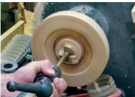
Drilling the end cap
