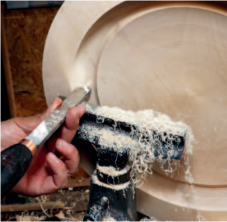
Round-nose scraper in trailing mode
