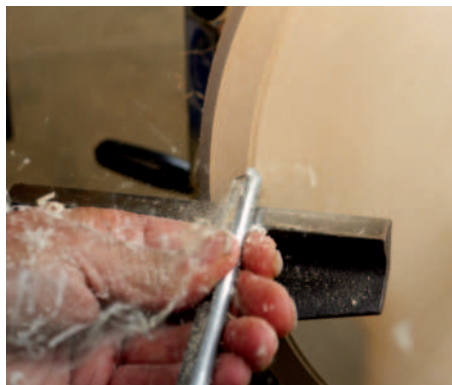
Cutting with the grain towards the rim
