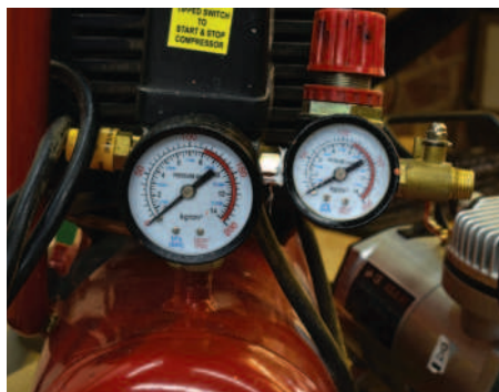
Ensure your compressor's air tank is empty at the end of each session
