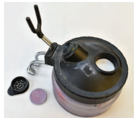
A new filter fitted to the cleaning pot
