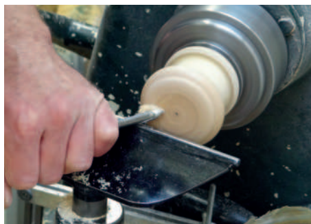
Completing the end cap held on a jam chuck
