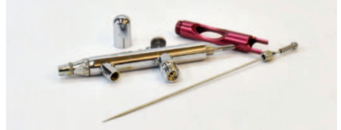
Partially disassembled airbrush with a 0.4mm needle
