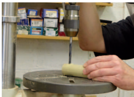
Drilling for the dowels
