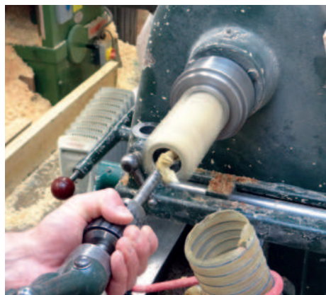
Drilling the tubes
