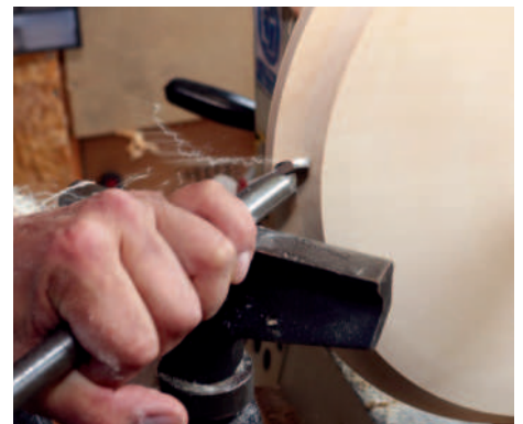
Cleaning the surface with a scraper
