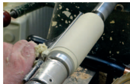
Turning the tenon to fit the end caps
