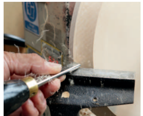
Skew being used for detailing
