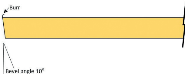
The profile of a traditional scraper
