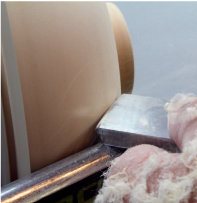
This grind can produce ultra-fine shavings
