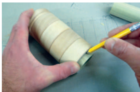
Marking the position for the fixed ring
