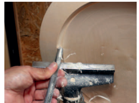
Progressing the undercut
