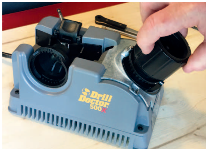
A diamond-coated wheel inside the unit grinds the tip of the drill bit at the proper angle as you rotate the chuck in the sharpening port
