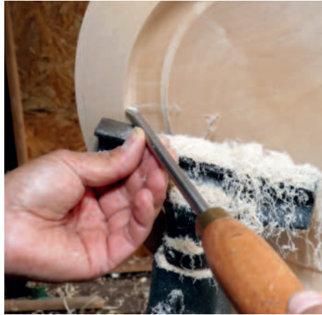
Using a round-nose box scraper to create the undercut
