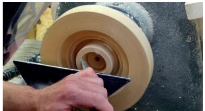
Hollowing the discs to make rings
