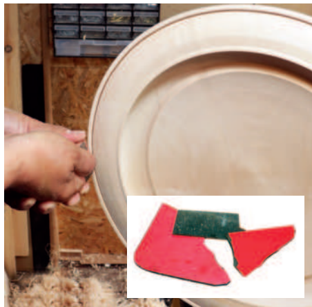
Burning the detail lines with Formica and hardwood wedge
