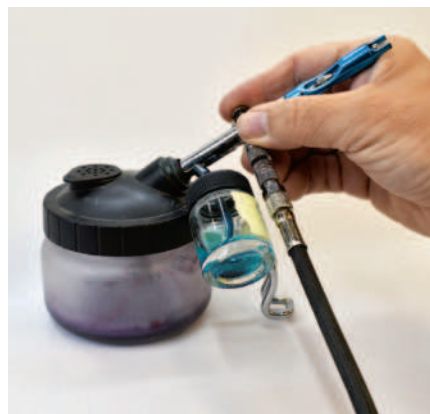
Using a cleaning pot
