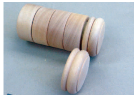
The end caps dry-fitted in place, including the fixed ring
