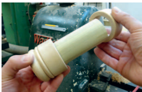
Test-fitting the rings on the outer tube
