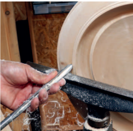
Cutting a convex detail
