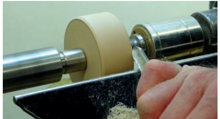
Adding a chamfer with the wing of my gouge
