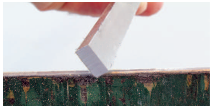
This clearly shows the peril of tilting the traditional scraper
