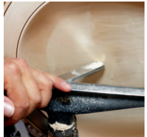
Cleaning the surface with a round-nose scraper
