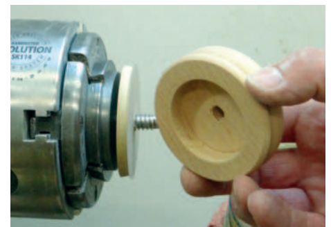
The end cap is mounted on my screw chuck
