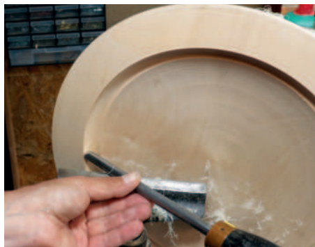
Flute opened up to the 2 o'clock position
