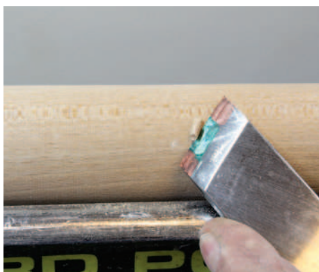
Position the tool at 45° to the lathe axis
