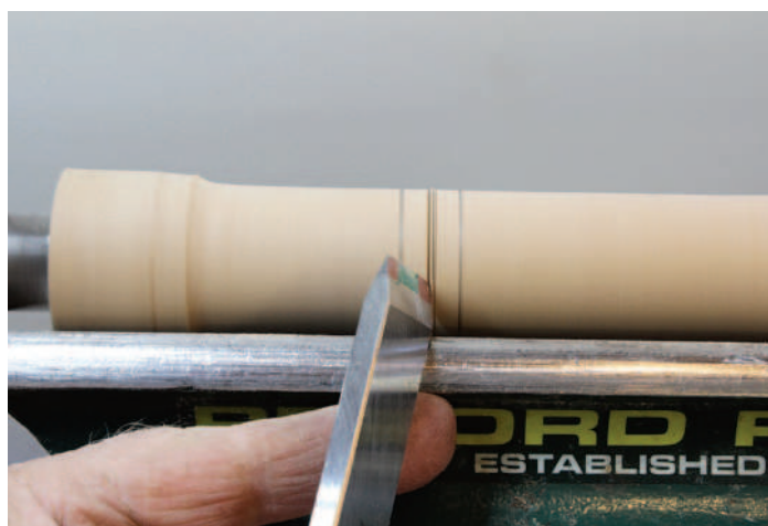
Cutting the left-hand side of the V
