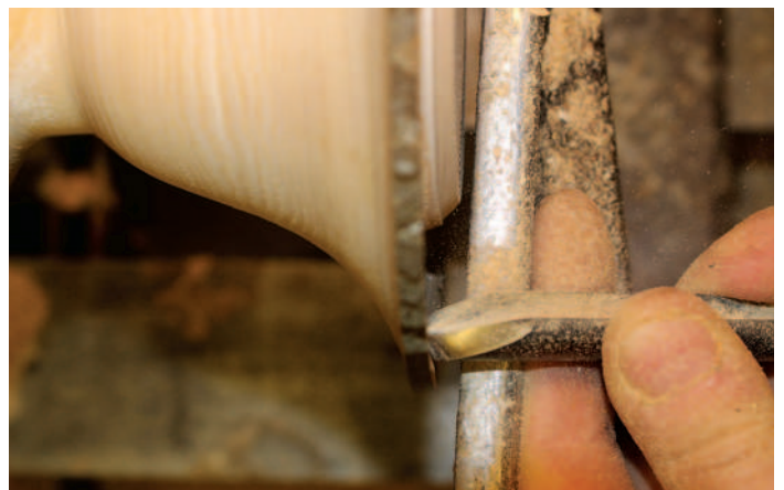
The wall thickness setting cut
