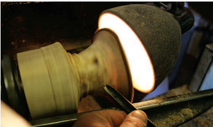
Following the interior curve to complete the exterior shape
