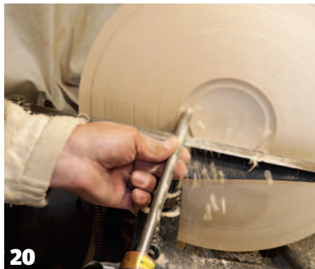
Hollowing the interior
