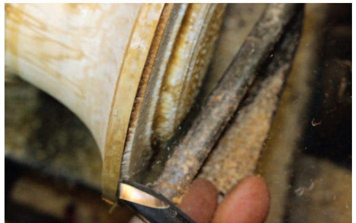
Push cut on interior lip
