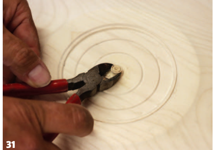
Using electrical snips to remove central pip
