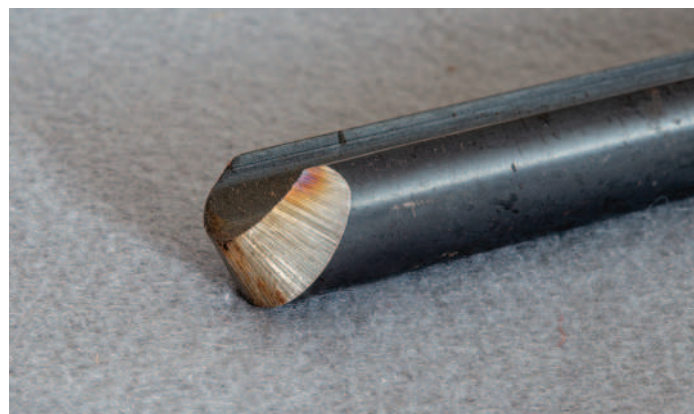
For HSS and beyond, if your tool is shaped correctly and cuts well, you can accept any unsightly heating discoloration as cosmetic only
