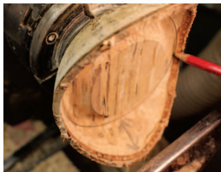
The depth of the wall thickness-setting cuts
