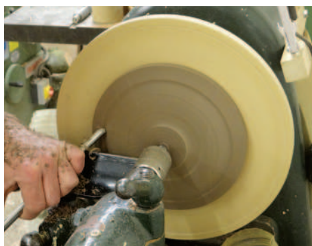
Turning the underside of the bowl
