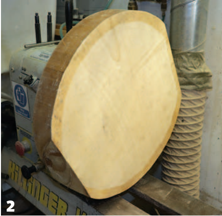
Blank mounted and ready for shaping the base
