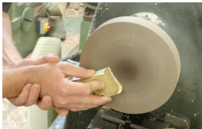
Final sanding on the lathe
