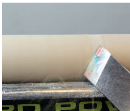
Cutting in the centre one-third of the cutting edge
