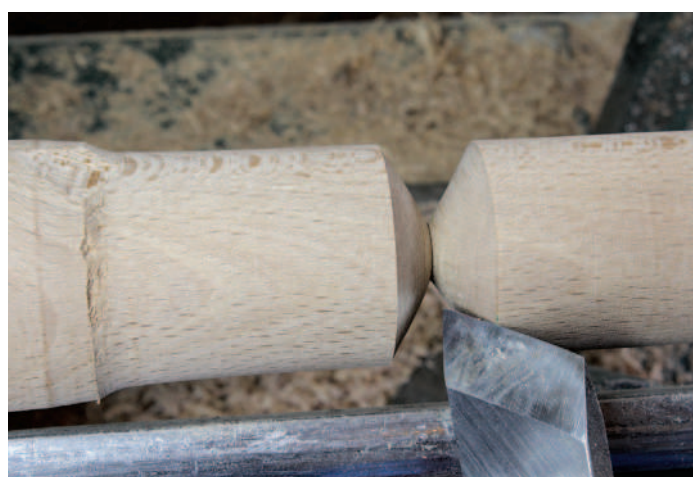
Rolling the tool too far will cause a catch
