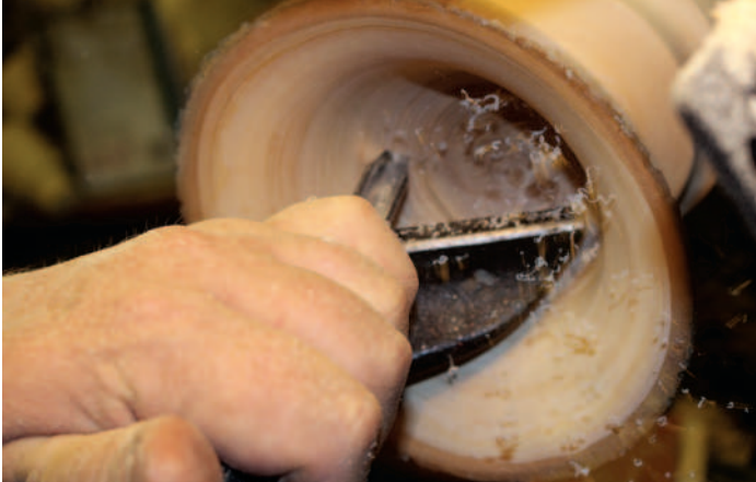
Following the curve using the bevel
