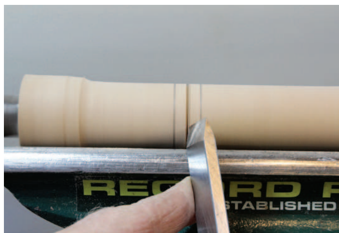
Cutting the right-hand side of the V
