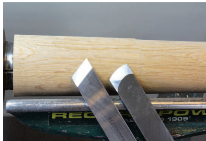
Comparing the skewed end with the radiused end
