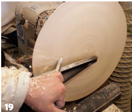
Cleaning the surface with a pull cut
