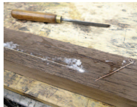
Wires fitted to the flat board
