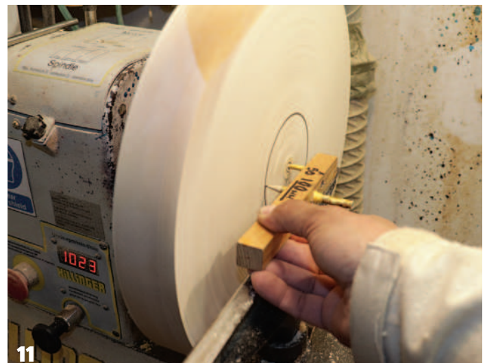
Homemade marking gauge
