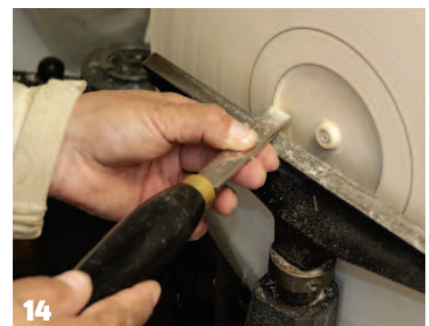
Using a skew to complete the recess shoulder
