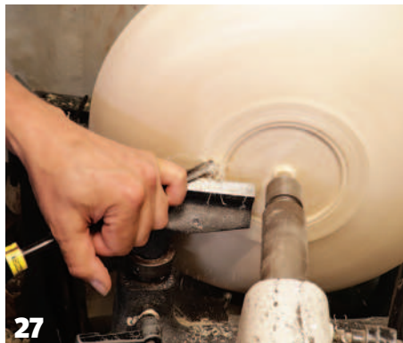
27 Refining the recess with a spindle gouge
