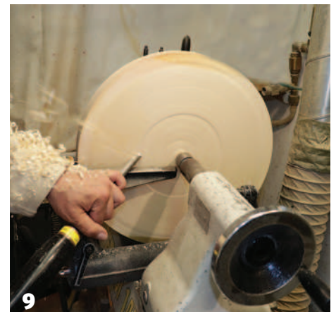
9 Cleaning up the face
