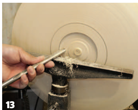
Refining and completing the recess with a bowl gouge
