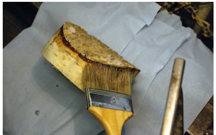
Sealing the bark edge on a cross-grain blank
