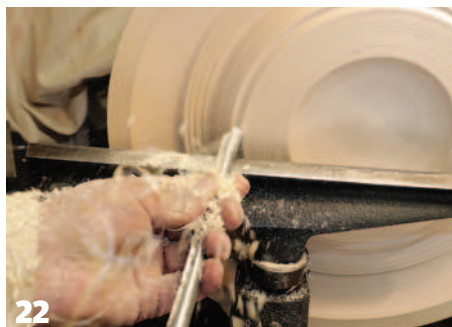
Cutting towards the final wall thickness
