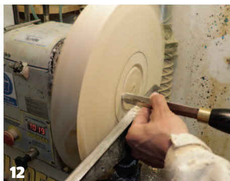
Plunge cut with the parting tool
