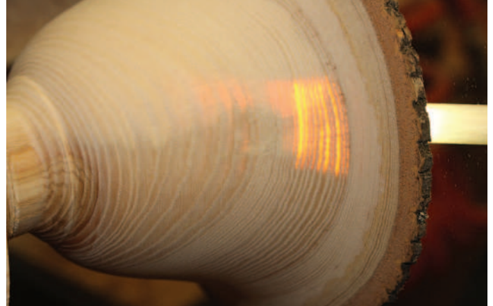
Different intensity of light on consistent-thickness wall
