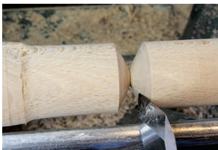
Always maintain that slight gap at the top of the cutting edge
