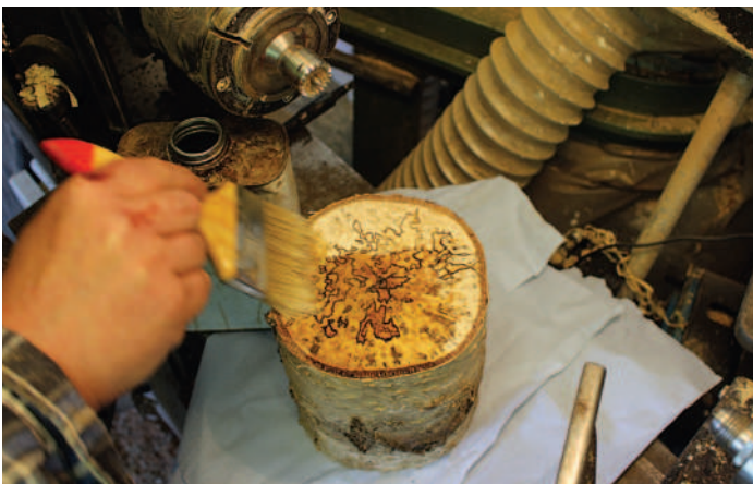
Sealing the end grain and bark edge
