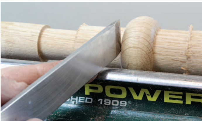
The final position of the tool on the left of the bead...
