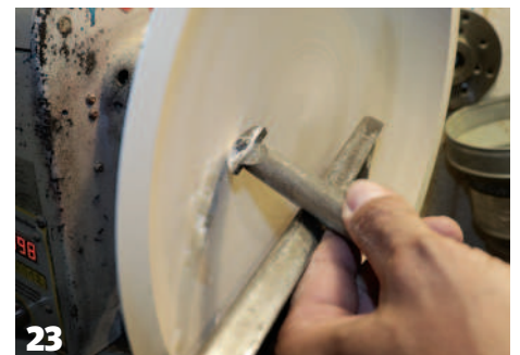
Refining with a French-curve scraper
