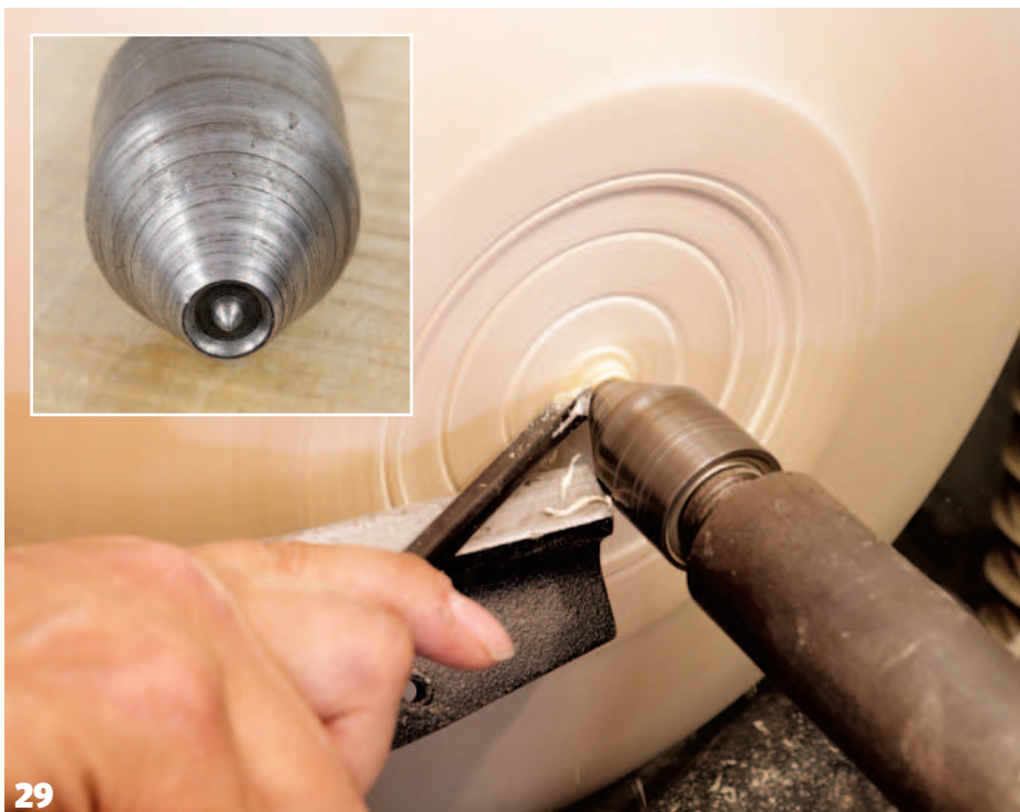
29 Cutting to the cone centre
