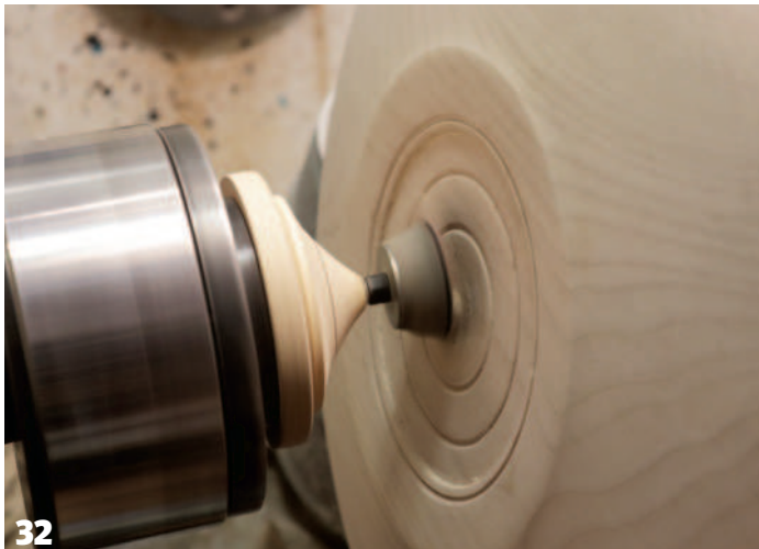
Using a lathe-mounted sanding arbour
