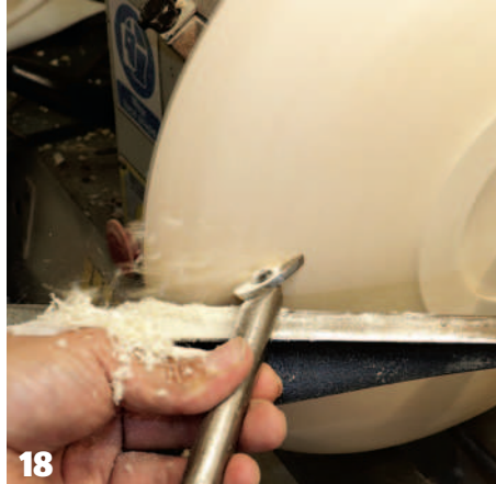
Using the square edge of a scraper to refine the surface
