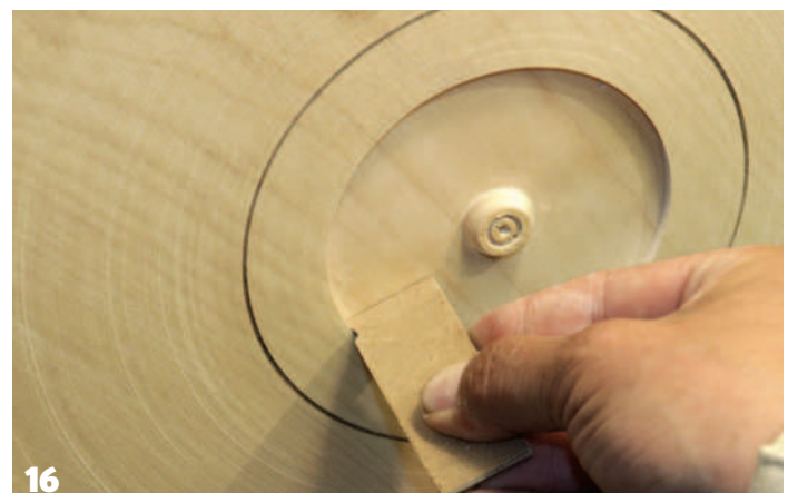
Using the template to check the recess
