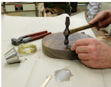
Tapping the brass rods into place
