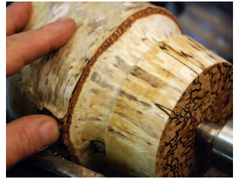
The headstock end can be treated at the same time
