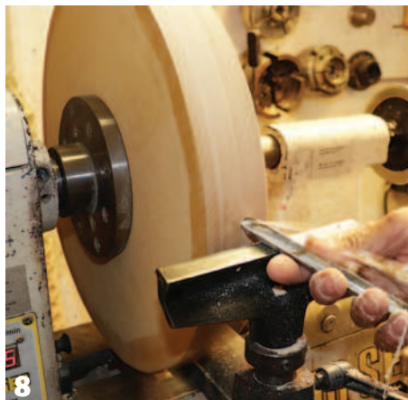
8 Turning the blank concentric
