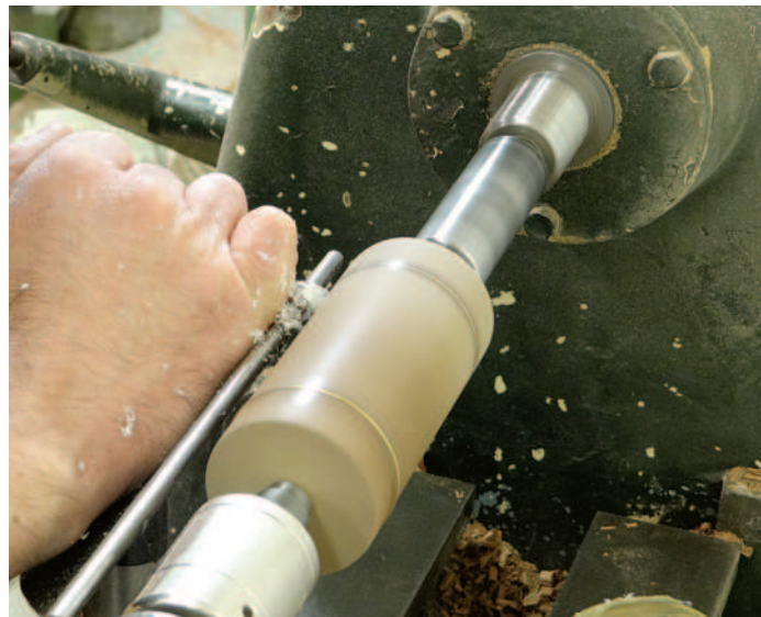
Turning the wire in the groove
