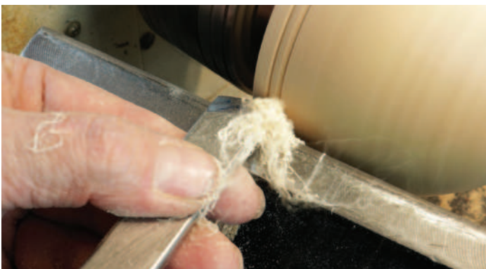
Forming a bead with a skew chisel in scraping mode
