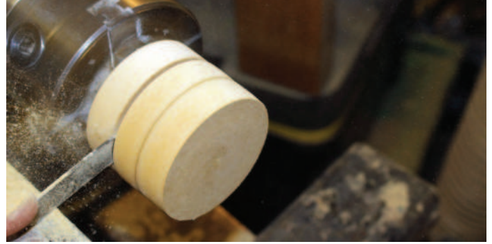
Truing the block and parting off a ring
