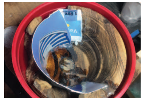
Ready for resin filling
