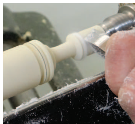
I even manage to roll the ball with my 'skew'
