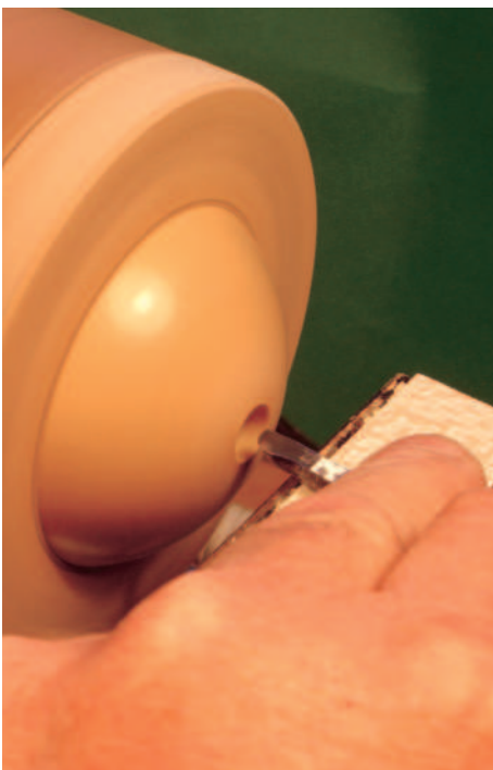
Fig 11.7 Beginning to cut with the profile tool
