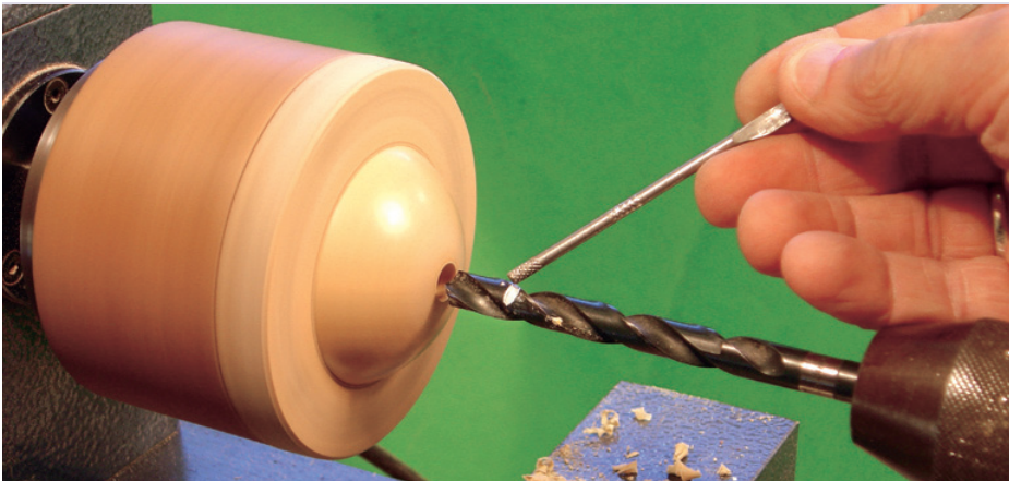
11.5 Drilling out the hole to the marked depth; the pointer indicates the depth mark on the drill
