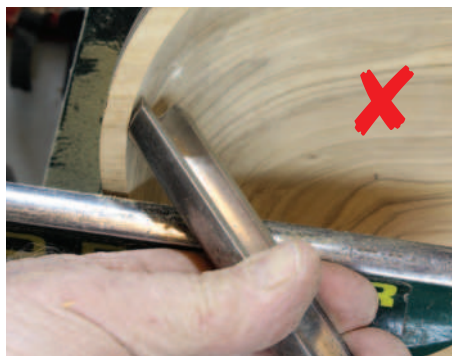
NEVER use your spindle roughing gouge in this way...
