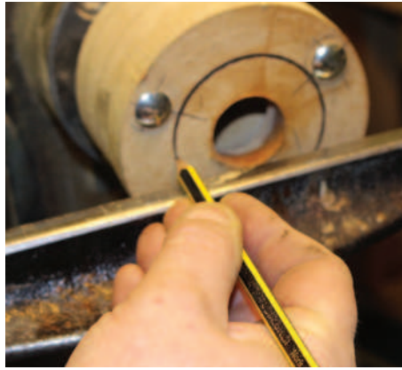
Turning the inside curve on the outer chuck face
