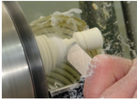
Turning with the curved negative rake scraper
