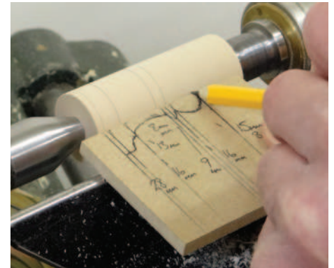
Marking the positions of details on the wooden blank
