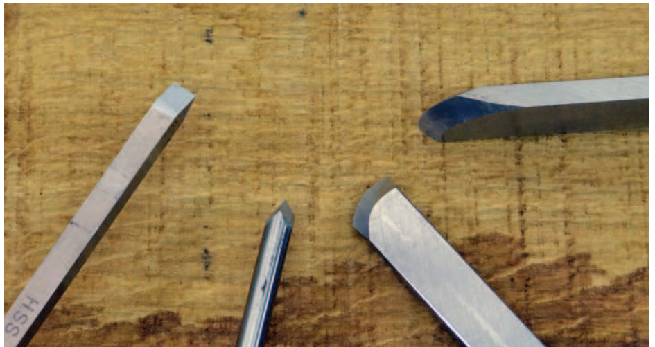
The negative rake scrapers I use, including a side view of the curved scraper
