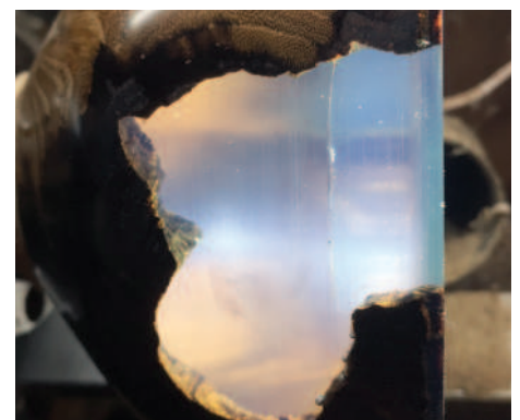
The resin join line which was hidden by a 10mm bead
