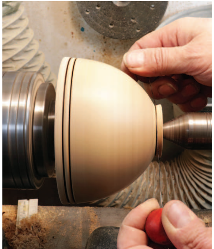
Burning lines wire with ball-shaped handles each end
