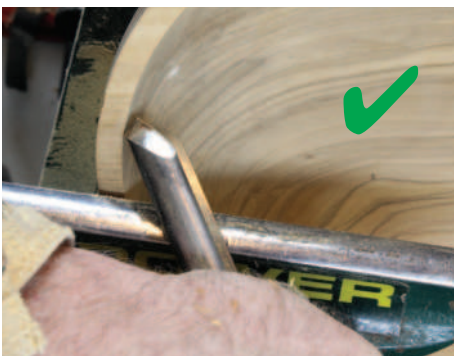
A correctly placed bowl gouge ready for turning the inside of a faceplate-oriented grain bowl
