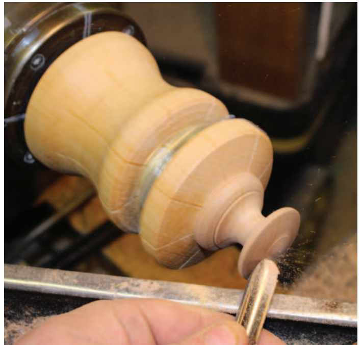
A small drawer knob turned in the collet chuck
