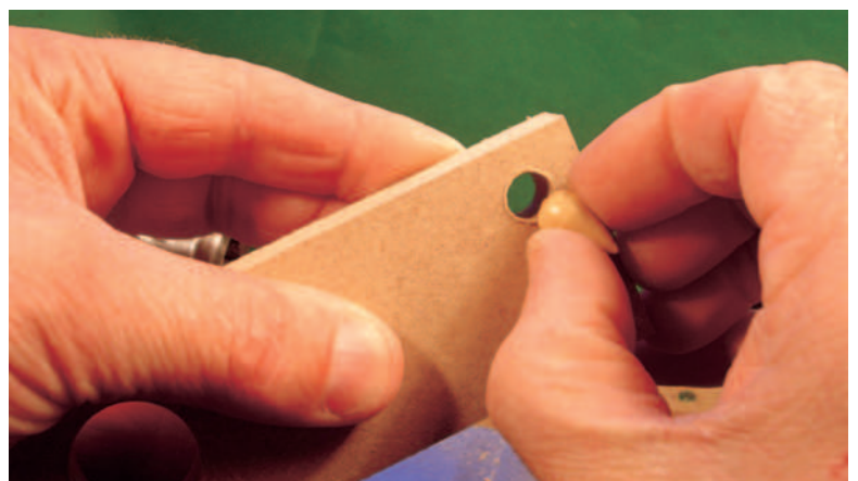
1.13 Testing the teardrop in the drilled hole
