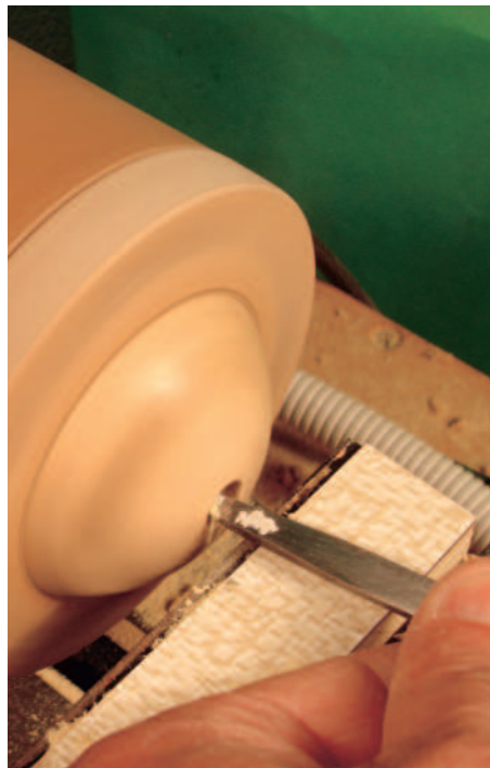
11.8 Moving the profile tool to the left as it approaches the entrance of the hole
