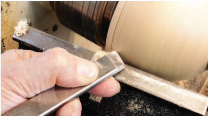
Forming grooves with a skew chisel in scraping mode
