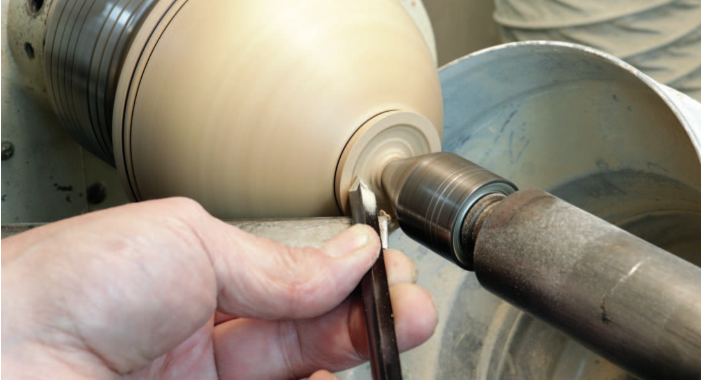
Finishing the base with spindle gouge
