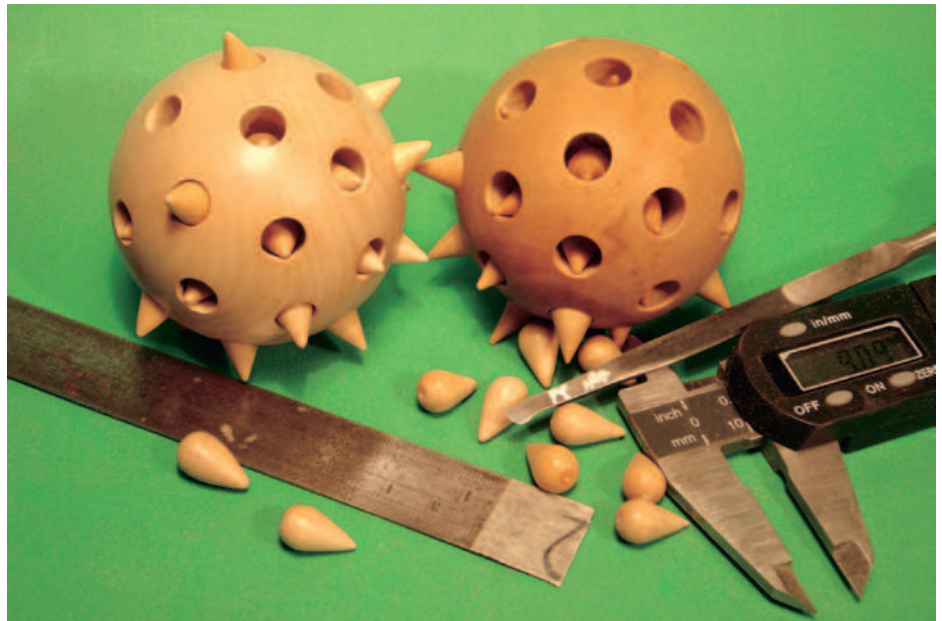
II.1 Two finished balls are shown with a spare set of 'teardrops', the specially shaped profile tool, template and callipers
