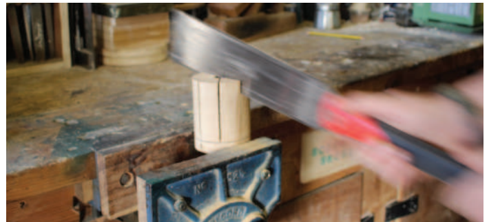
Cutting the jaws with a pullsaw
