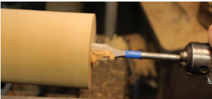
Drilling out the trued-up cylinder
