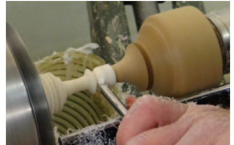
Using the point tool to roll the ball
