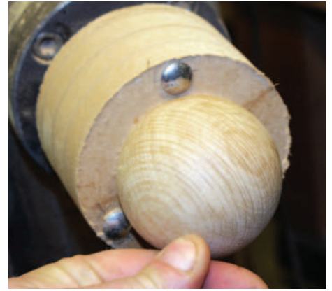
Checking the outer curve on the outer chuck face
