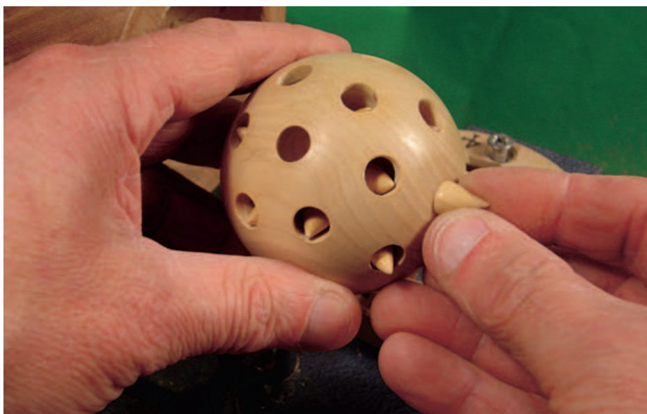
11.15 Pushing the teardrops into their holes
