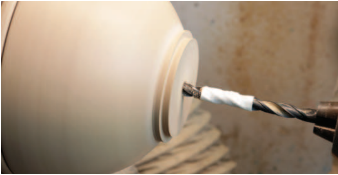
Drilling a hole
