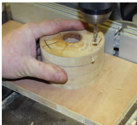
Drilling the 6mm holes
