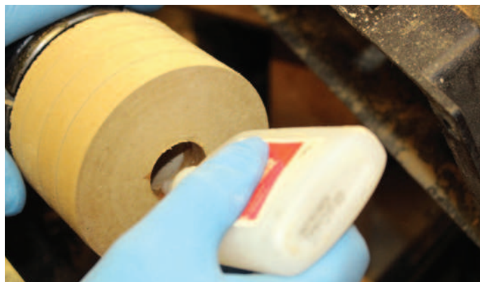
Firming up the wall of the hole with CA glue
