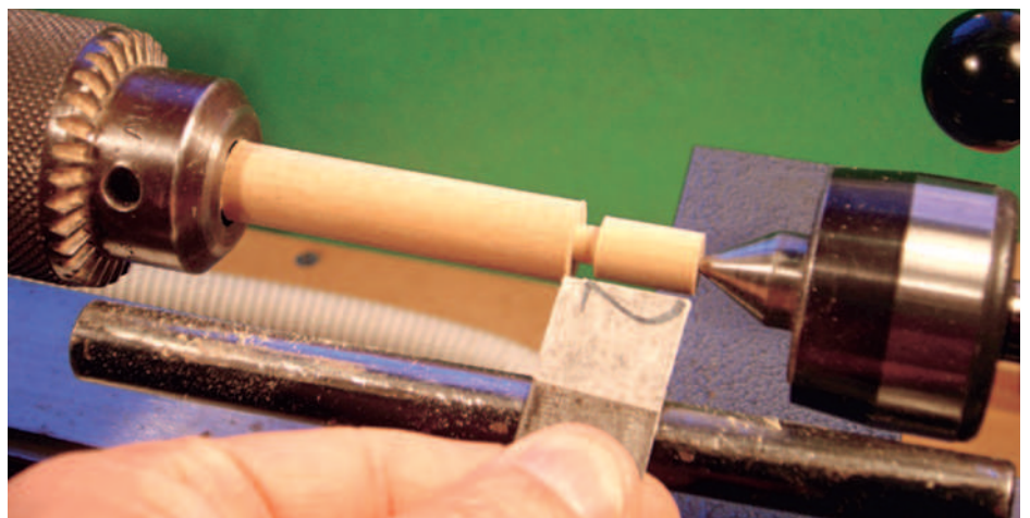
1.10 Using the template to judge the shape of the teardrop
