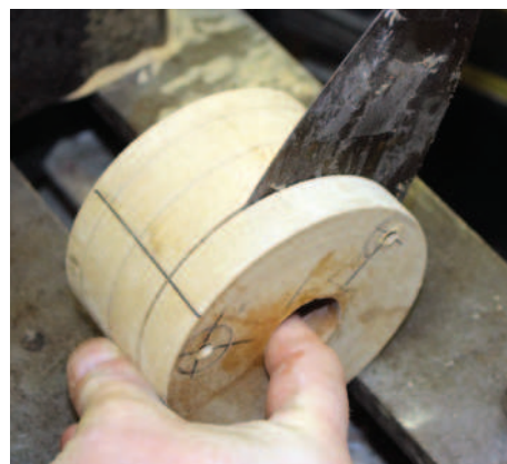
Parting off the single layer board
