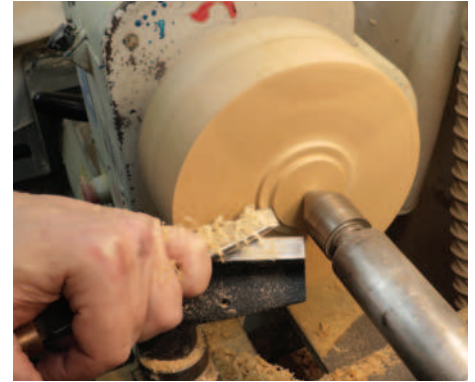
Skew chisel used as a scraper to refine the spigot
