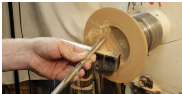
Handle low &amp; flute pointing in the direction of travel to form the top of the opening
