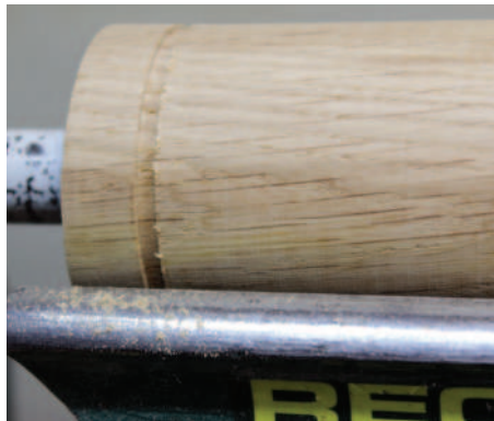
Torn grain at the start of a peeling cut
