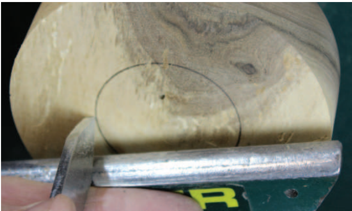
Tool correctly angled
