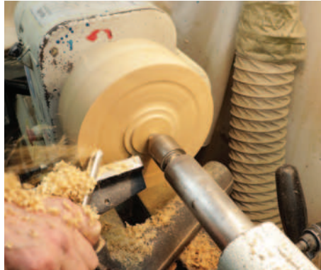
A pull cut being used to remove waste wood
