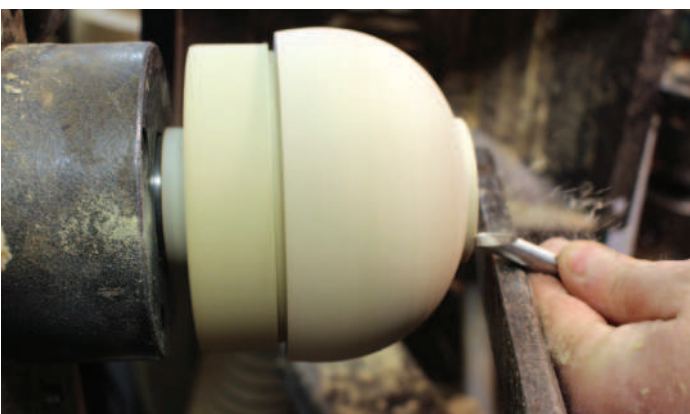
Bowl mounted on tenon turned on jam chuck
