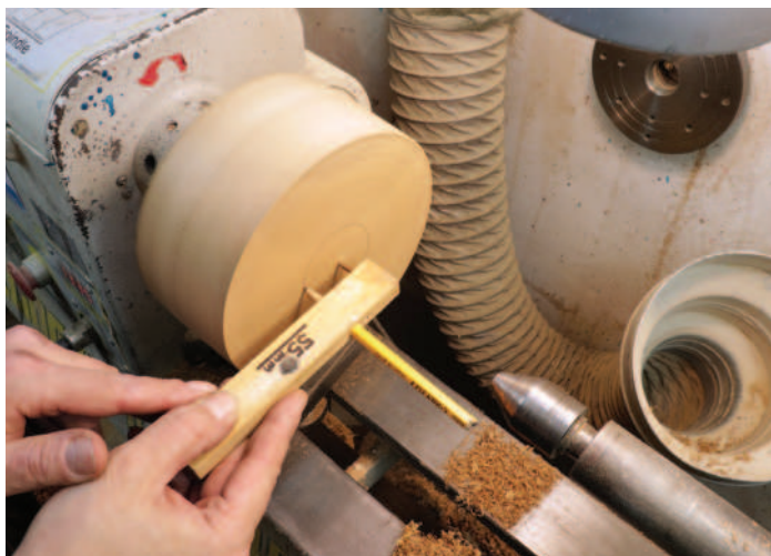
Marking a spigot or recess width to suit a set of specific chuck jaws
