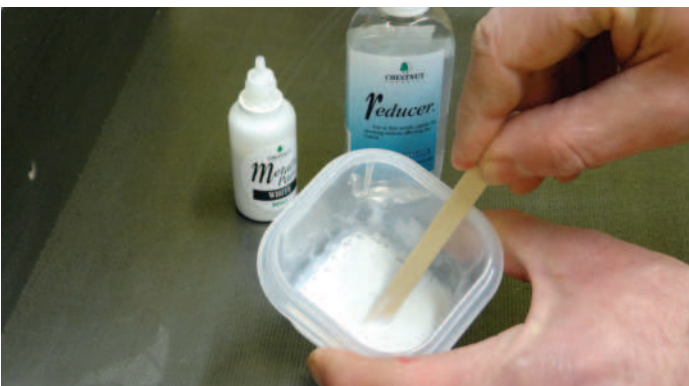
Thinning the paint with reducer and mixing with a lolly stick
