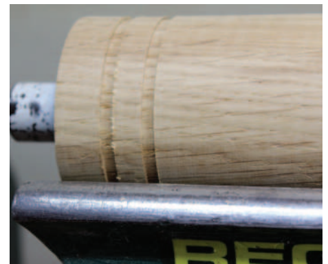
An improved surface achieved by a gentle scraping cut
