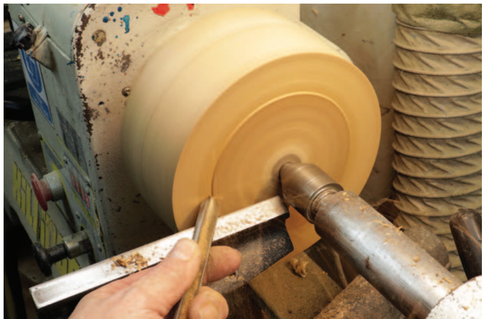
Cleaning up the face of a bowl blank at the tailstock end of the lathe
