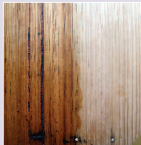
Feature-grade face grain showing insect holes and gum vein, previously considered low-grade wood and used for fence palings, structural material and garden stake
