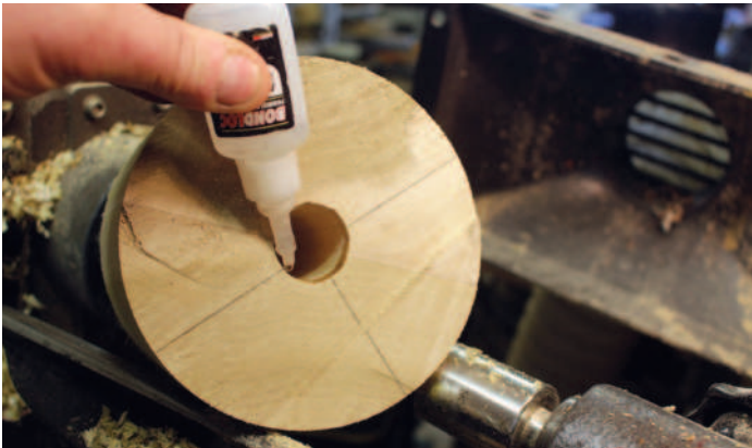
Applying thin CA glue to the wall of the pilot hole
