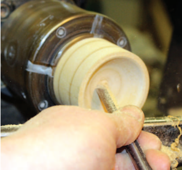
Shaping the drive centre
