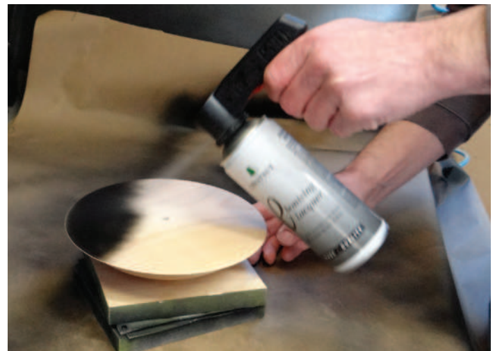
Spraying the first coat of ebonising lacquer
