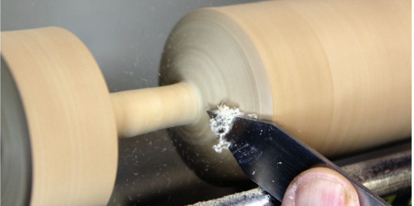
Scraping produces ultra-fine shavings
