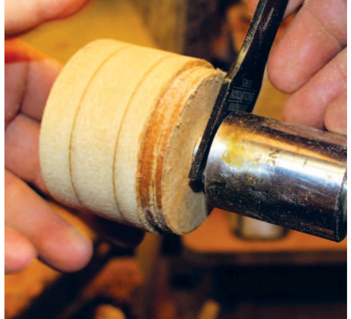
Fitting the tailstock drive head
