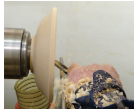
Beginning to turn the top surface after turning the underside
