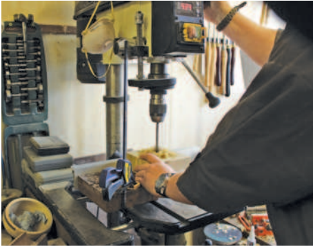
Drilling a pilot hole
