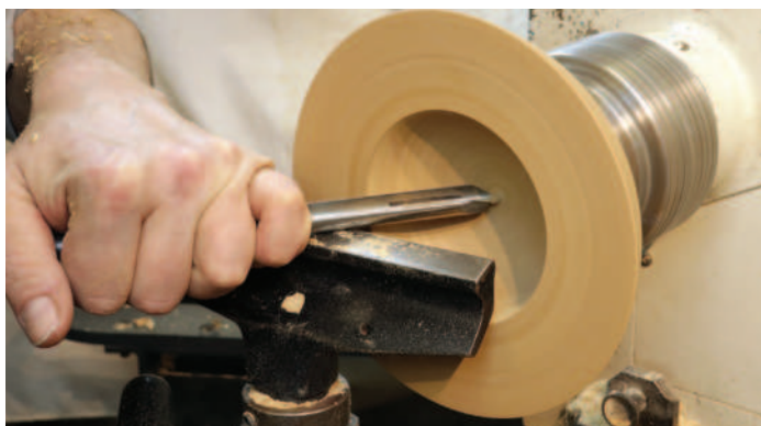
Cutting the very bottom of the inner area
