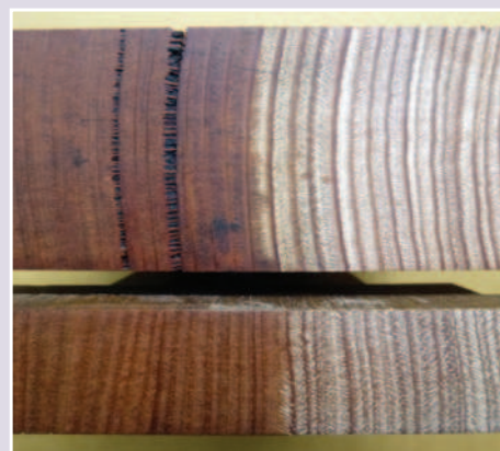
End grain of regrowth wood (approximately 80 years old), top, and old growth below
