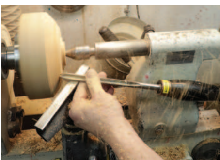
The gouge handle fouling the tailstock assembly
