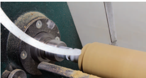
Callipers must have rounded ends
