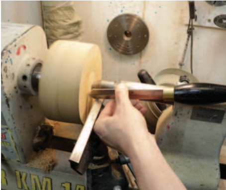
A parting tool making the initial cut for the spigot width
