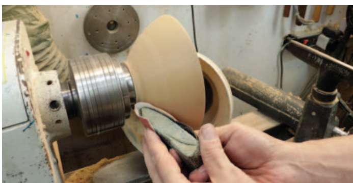
Sanding using a pad to keep fingers away from the chuck
