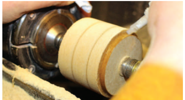
Firming the tenon with CA adhesive
