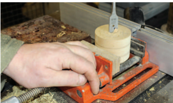
Drilling the pilot hole
