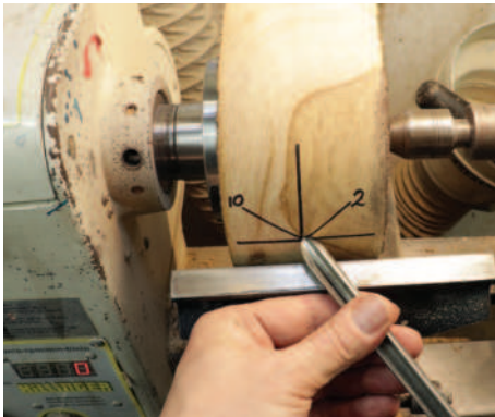
The angle of flute of the gouge and handle when cutting towards the headstock
