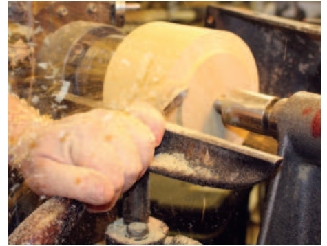
Truing the scrap block
