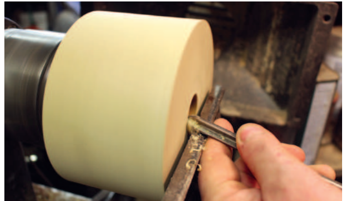
Cutting a chamfer on the edge of the pilot hole
