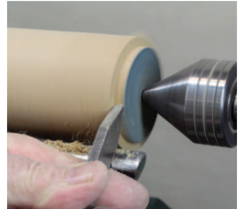
A little sideways pressure prevents drift
