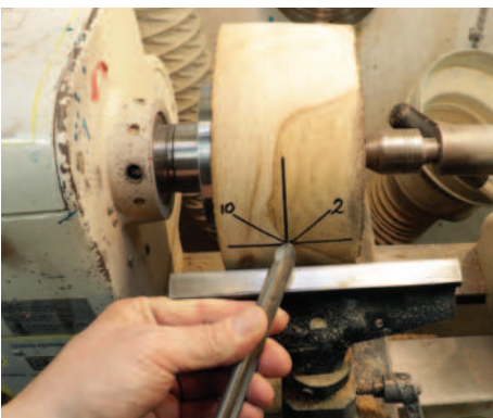
The angle of flute of the gouge and handle when cutting towards the tailstock
