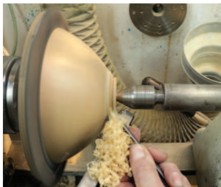
Refining the foot area
