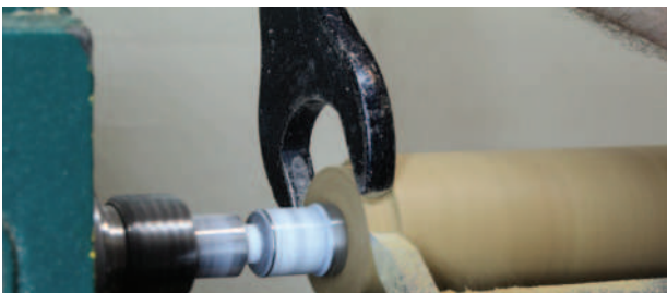
A spanner the right size with rounded ends can be handy
