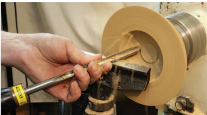
Handle more towards the horizontal to reach the bottom area
