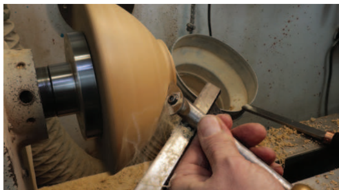
Shear cut with a scraper
