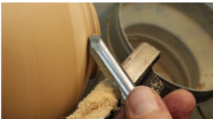
Shear cutting with the long edge of the gouge
