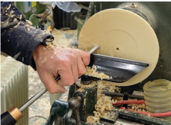
Shaping the top face of the bowl
