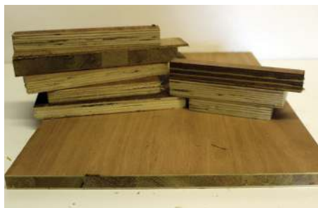
Marine and faced ply (to right) suitable for chuck making
