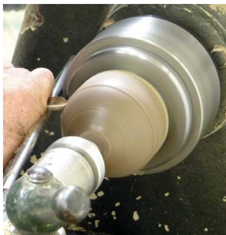
Turning the top of the dome
