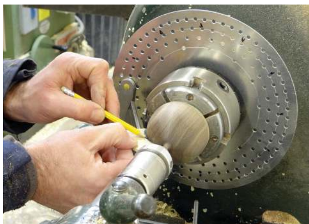
Marking out using my indexer
