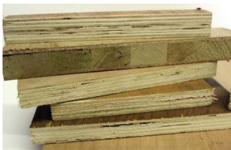
Poor quality construction plywood
