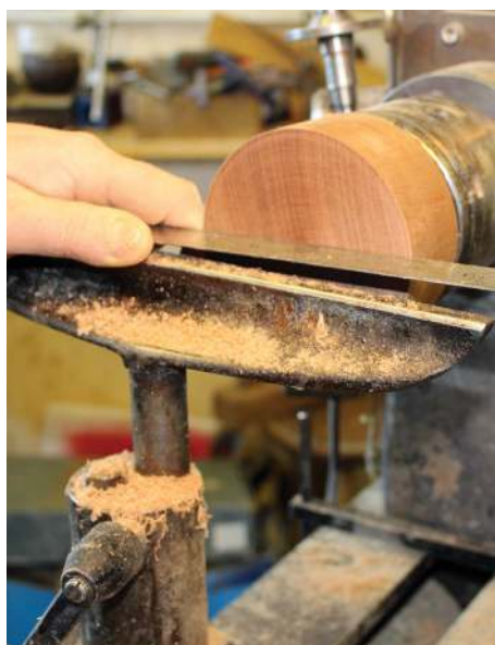
Checking for flatness
