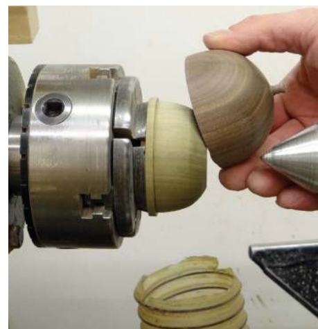
It is mounted over scrap in the chuck
