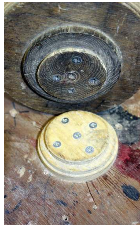
Glued and screwed tenons on chucks
