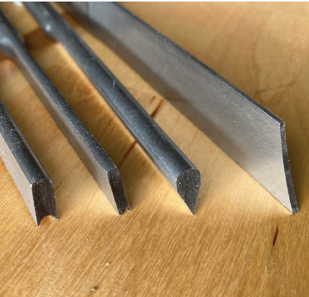
\frac{3}{16} in and \frac{1}{16} in bead-forming tools, diamond tool – aka tear-drop tool and a thin \frac{1}{16} in tapered parting tool
