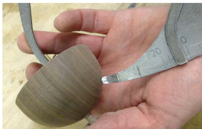
Callipers confirm a 3mm wall thickness
