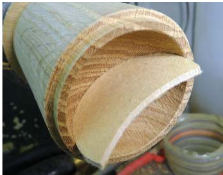
Checking the inner shape against another template
