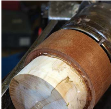
Blank secured and glue cured and cooled
