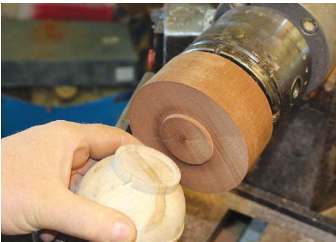
Tenon turned on platen to take bowl foot
