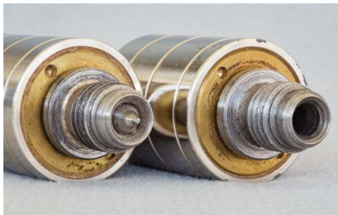
I find use for both a revolving tailstock center with a point and with the point removed or withdrawn
