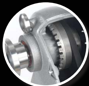
Heavy-duty spindle lock and 24 point indexing
