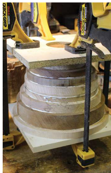
Clamping the vessel for curing
