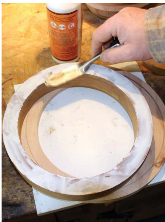
Applying wood glue
