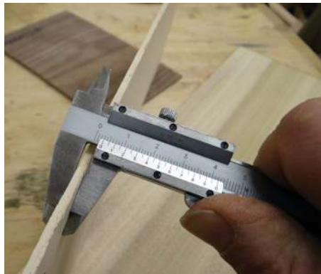
Checking the thickness with a Vernier
