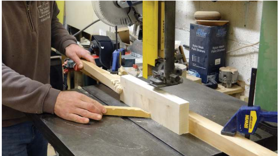
Cutting 3mm-thick pieces on the bandsaw
