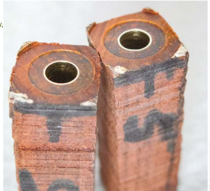
Pen blanks with a tube glued in and faced ready for turning
