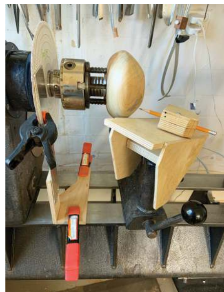
Angle the platform for marking diagonals, creating unique designs
