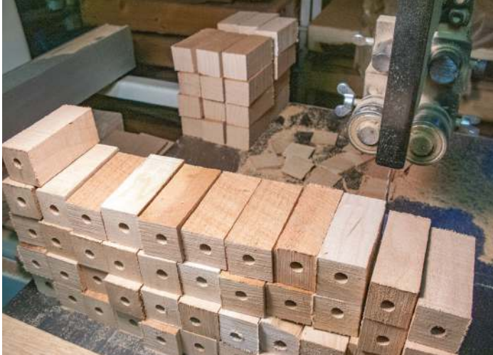
Bandsawn pen blanks ready for tube insertion
