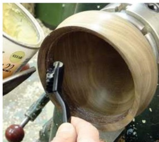
Waxing the thread to smooth the cut
