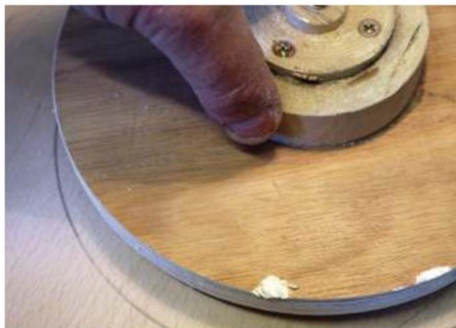
Mating the chuck to the blank
