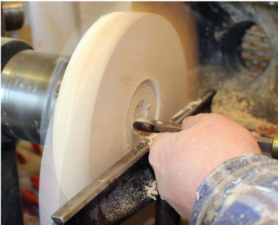
Turning the mechanism/mounting recess
