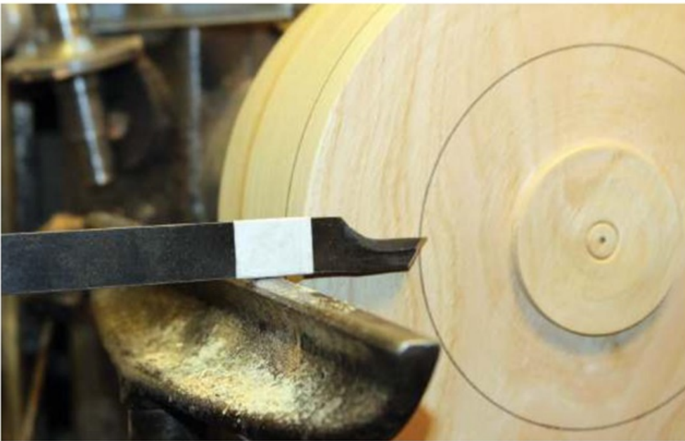
Cut depth marked on coring tool
