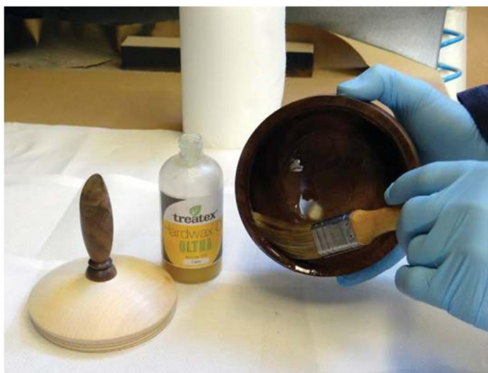
Oiling the bowl, brushing into the threads
