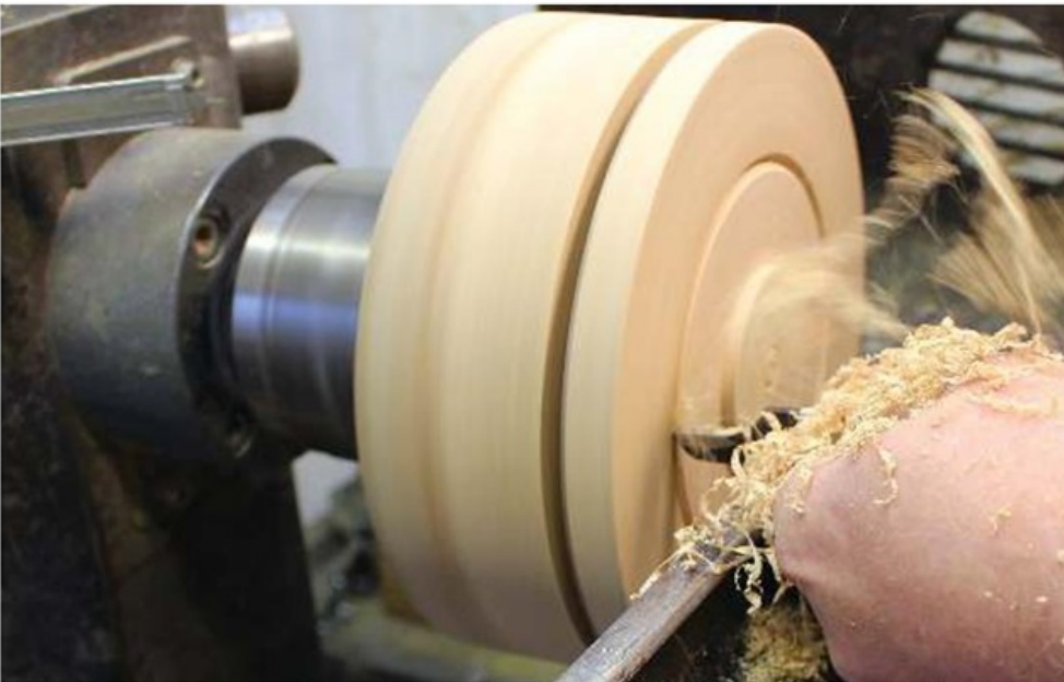
Making the face cut
