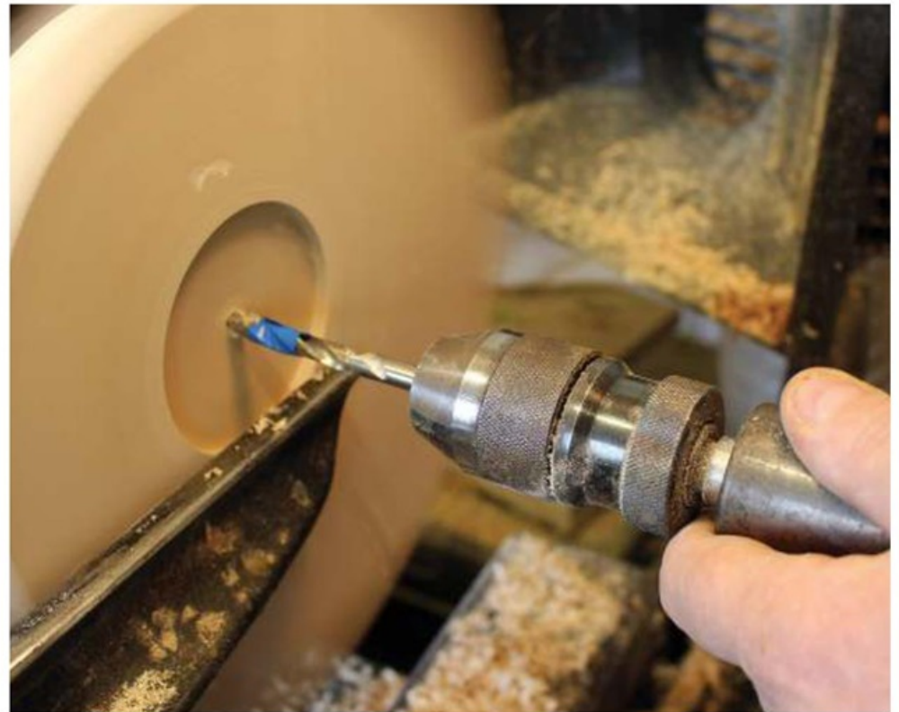
Drilling the clock stem hole
