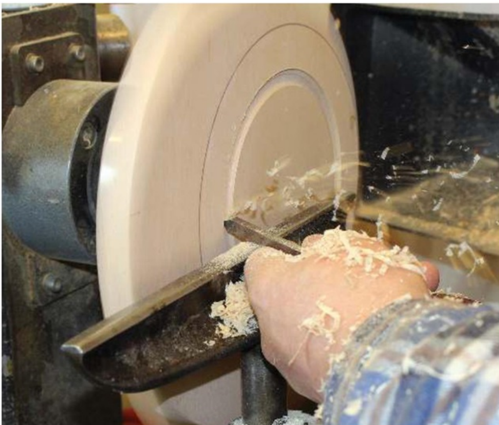
Cutting the recess
