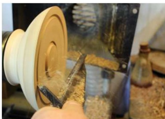
Lining up the coring cut
