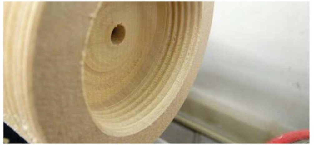
The result of the inside thread
