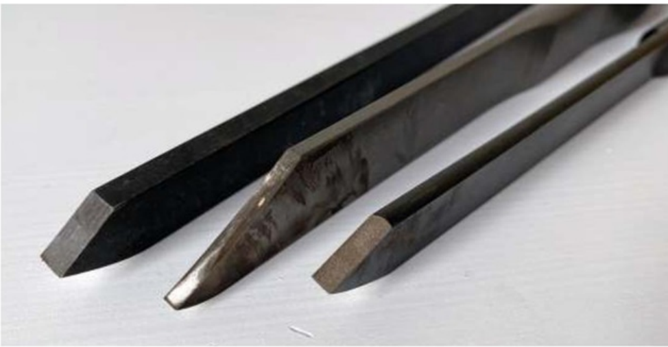
Some heavy-duty parting tools suitable for cutting rings
