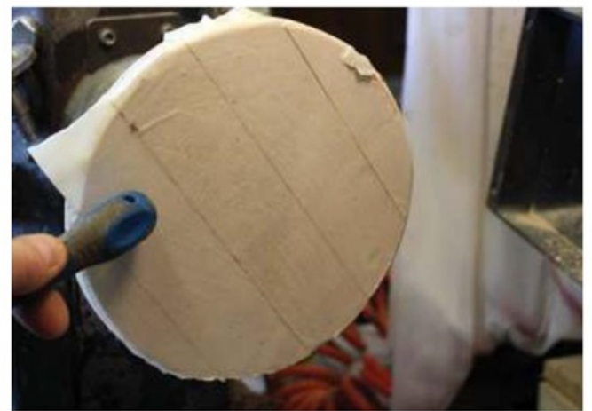
Double-sided tape applied to mounting chuck
