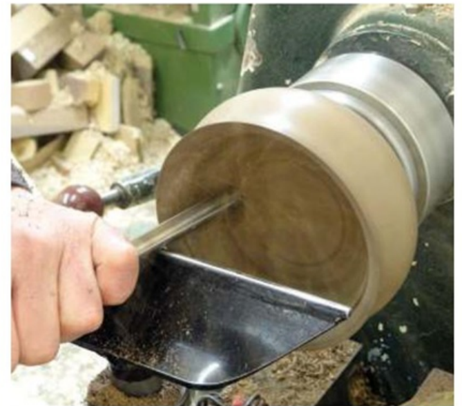
Turning the inside of the bowl
