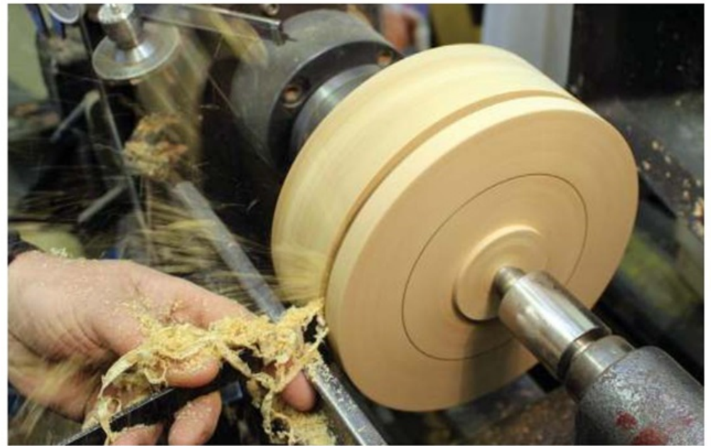
Making the back cut
