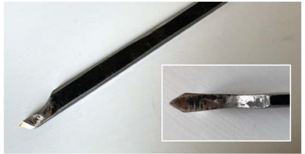
Kel McNaughton small straight coring blade. This is also the blade we will use for coring out later
