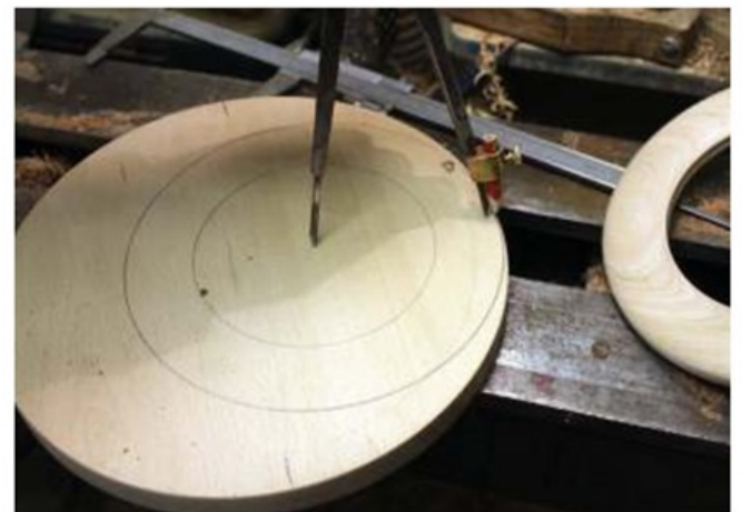
Scribing the dimensions of the saved ring
