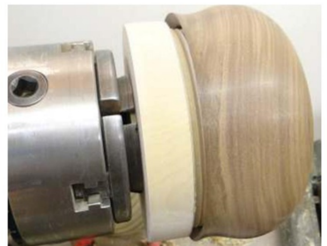
Testing the fit of the threads
