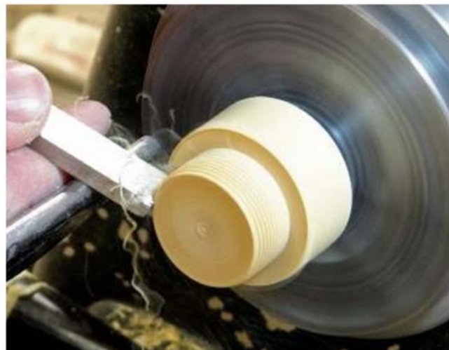
Chasing the outside thread
