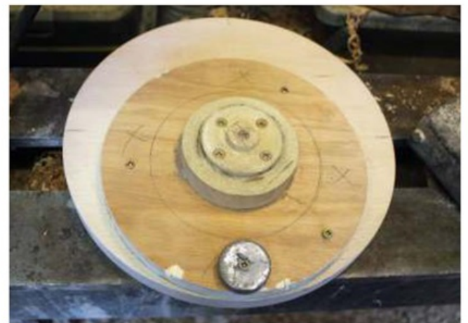
Workpiece mated to platten with counter-balance weight
