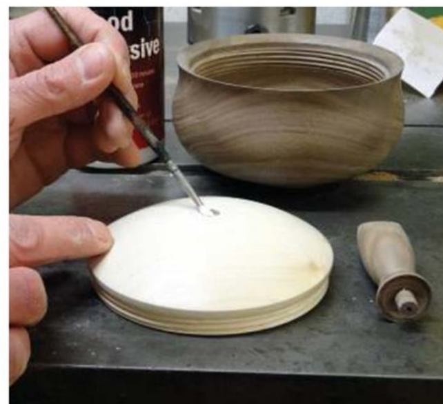
Fitting the finial
