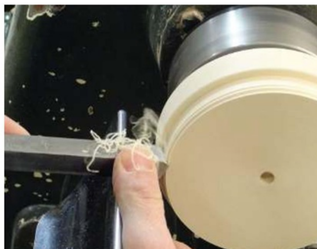
Cutting the thread on the lid
