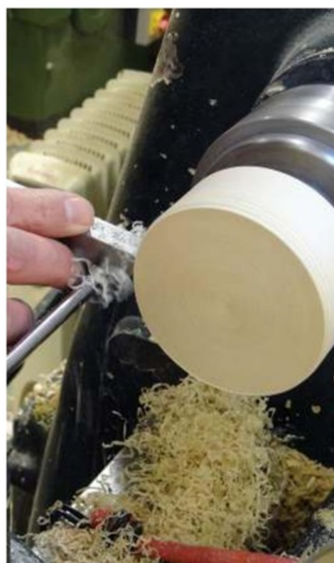
Chasing the outside thread on the sycamore blank
