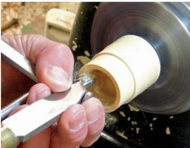
Chasing the inside thread
