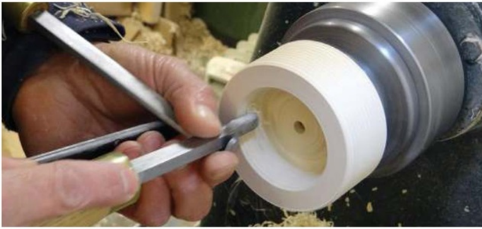
Chasing the inside thread in sycamore
