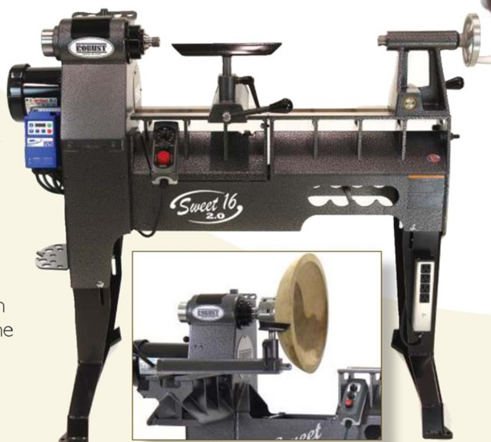
Turn diameters up to 32" by removing the Sweet 16's gap bed.
