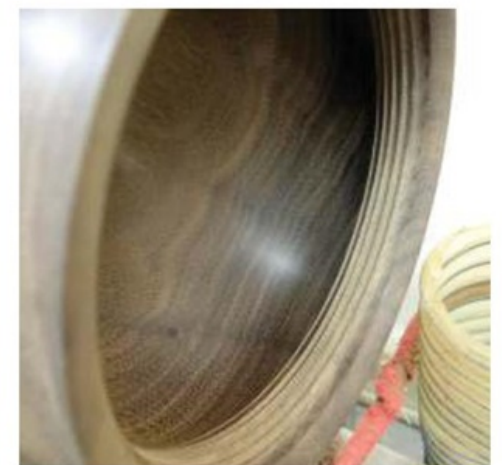
The finished thread
