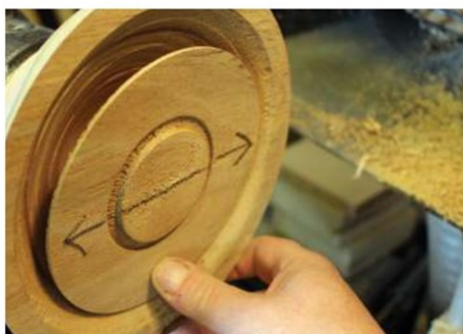
Parting the cone core
