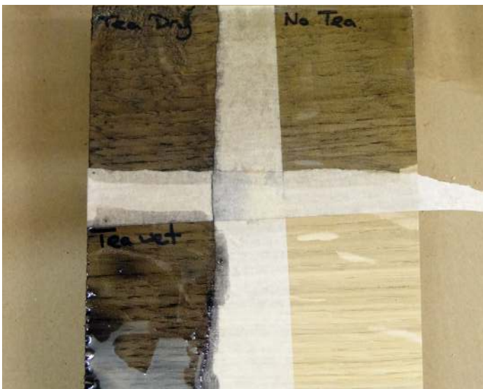
The tea experiment with freshly applied ebonising solution
