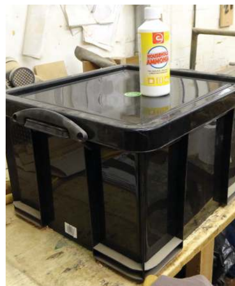
Left to fume for 24 hours in the sealed box
