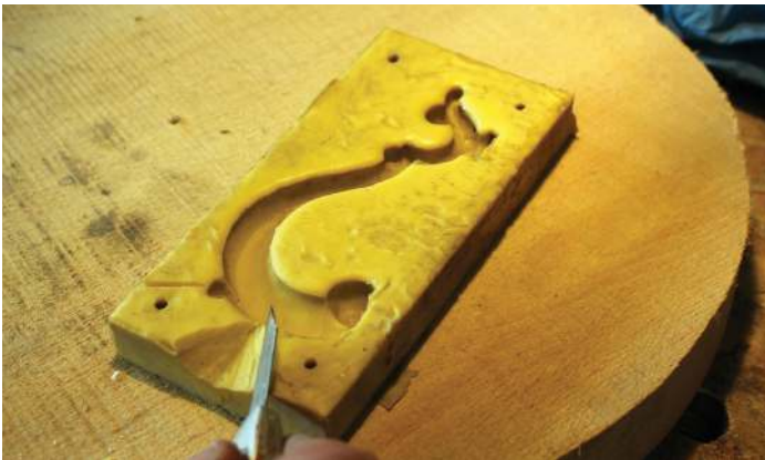
Cutting a vent and sprue
