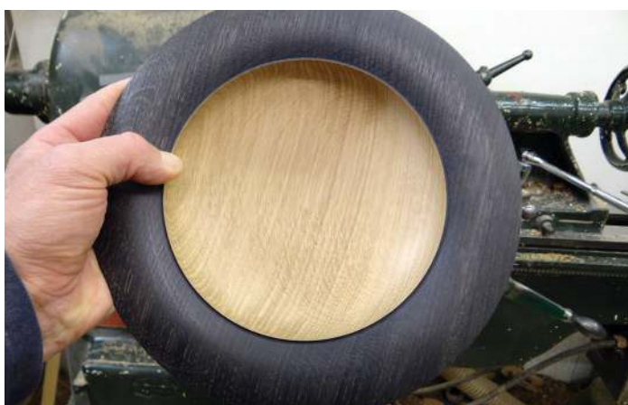
Slight colouring on the back of the edge sands off easily
