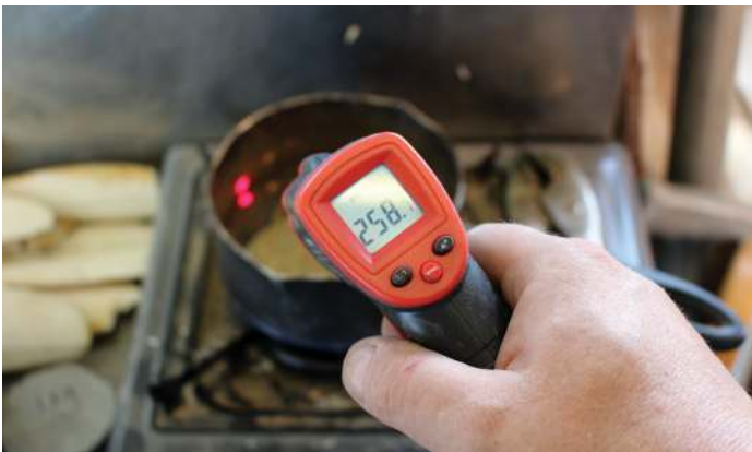
Checking temperature of molten pewter
