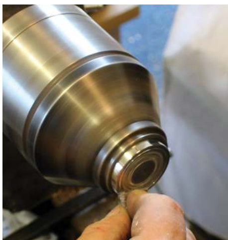
Cleaning the surface with wire wool
