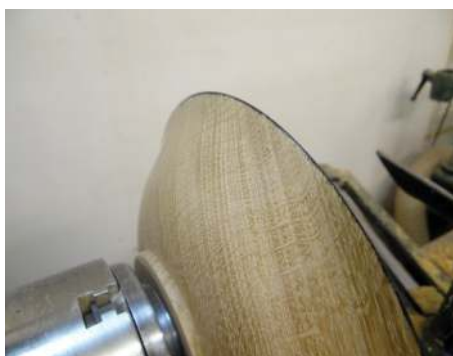
Slight colouring on the back of the edge sands off easily
