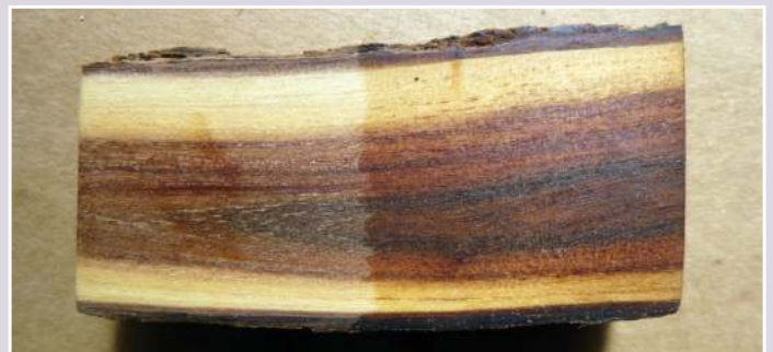
A cross-grain section of root wood, showing drastic contrast in colour between sapwood and true wood
