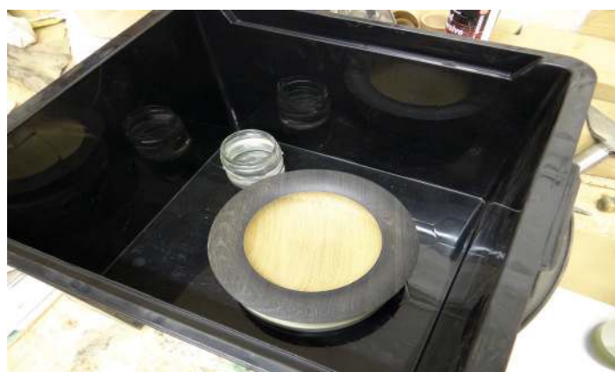
LEFT: The finished bowl before fuming ABOVE: Bowl in the fuming box
