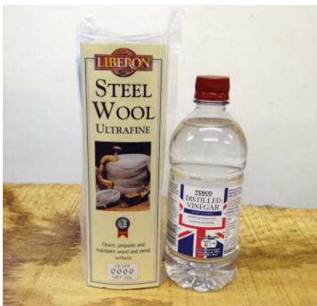
Distilled vinegar and steel wool to make the ebonising solution
