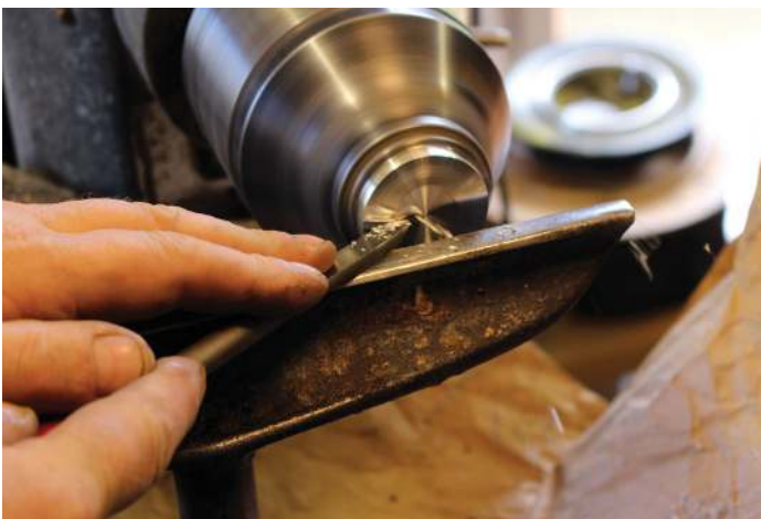
Cleaning the face with a negative rake scraper
