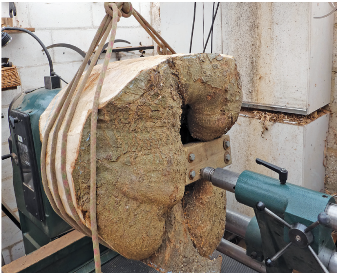
The sweet chestnut blank being hoisted on to the lathe. A block of timber was fastened with coach screws to offer a temporary location for the tailstock centre during initial turning. The shape can be adjusted with the Arbortech to get a better balance if necessary. Tailstock support is brought up whenever possible. The outside shape is turned followed by the inside shape, leaving the tailstock in place for as long as possible
