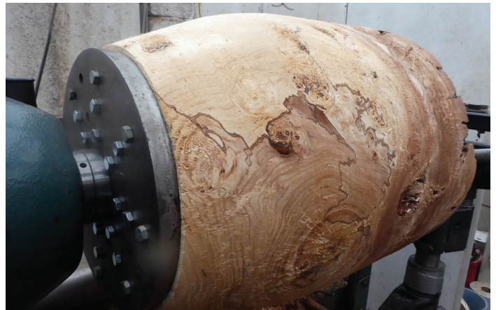
Alternative fixing method. This decayed and spalted English elm ( Ulmus procera ) is mounted on a faceplate. The finished piece was parted off at a later stage, sacrificing the lower part of the blank into which the coach screws were placed
