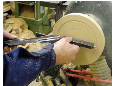
Using the sliding bevel to guide the angle of my cut
