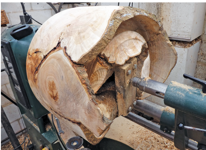
For security, as much waste as possible is removed and turning of the inside done with a very low lathe speed while the tailstock is in place
