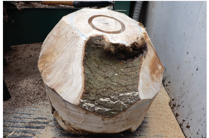
The sweet chestnut blank shaped with a chainsaw showing the mounting spigot cut with a plunging router
