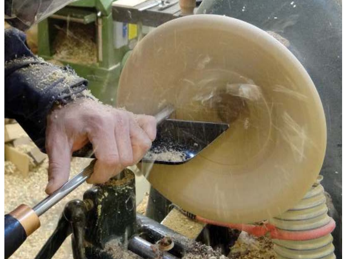
Turning the inside of the bowl
