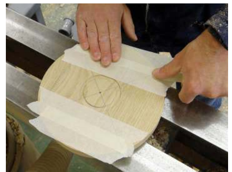
Adding masking tape to the back of the disc
