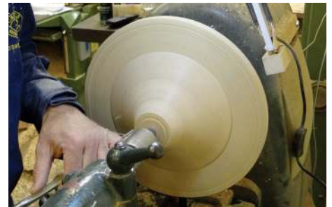
Removing the tenon
