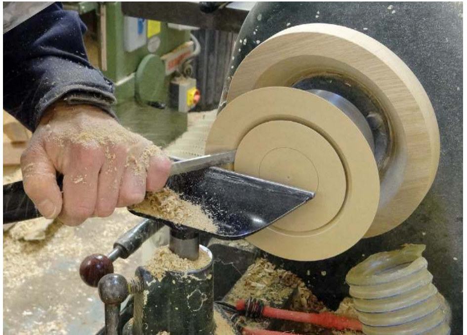
I cut the second ring with the first safely out of the way
