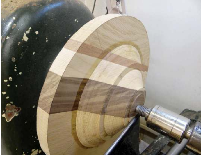
Laminated bowl out of cramps and ready to turn
