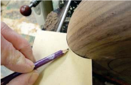
Checking against the template, which shows where more wood needs removing
