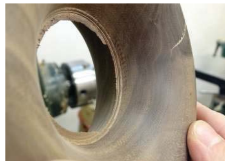
The curves meet well with just a slight seam line to remove
