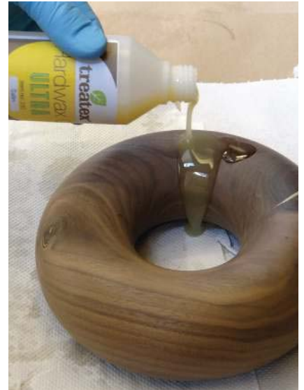
Applying oil to the torus
