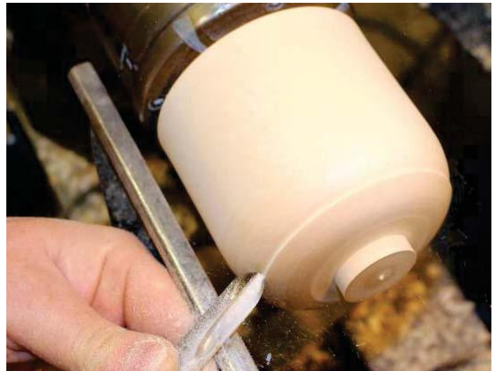
Initial shaping of top section
