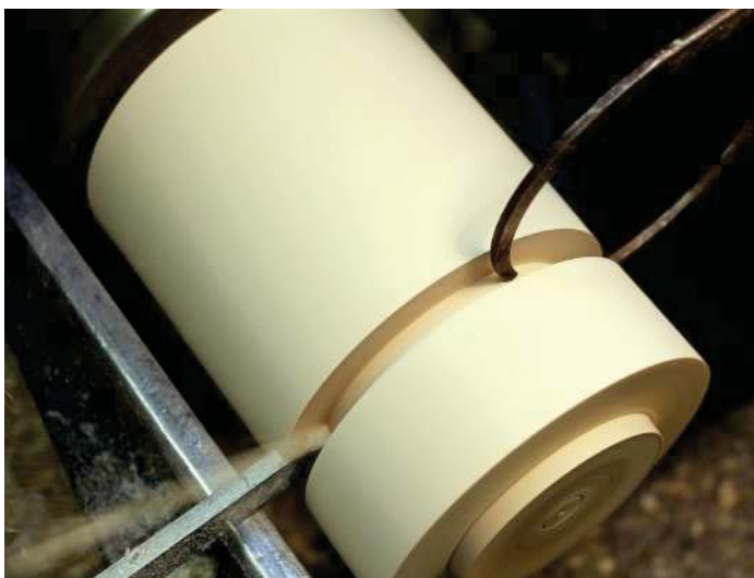
Blank mounted, trued and tenon turned
