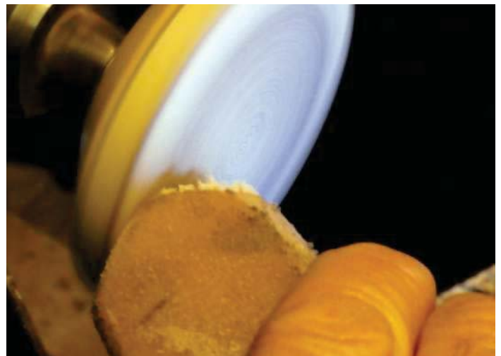
Cleaning the sanding disc with a rubber block
