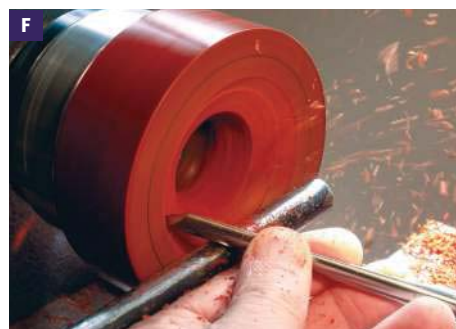
F The work is flipped over and the curve is turned down towards the centre
