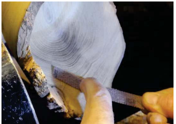
Pulling a strip of mesh-backed abrasive under a finger
