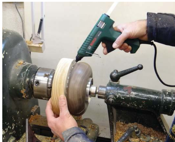
Additional glue to reinforce the joint
