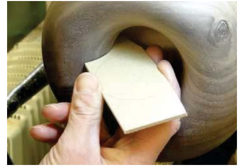
Checking the curve flows all the way around with the template
