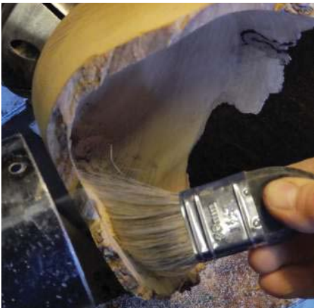
Sweeping the dust into the extractor
