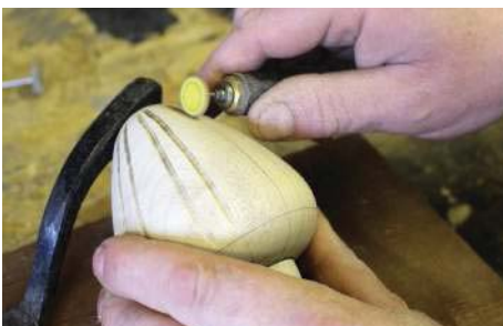
Using a rotary toothed carbide burr
