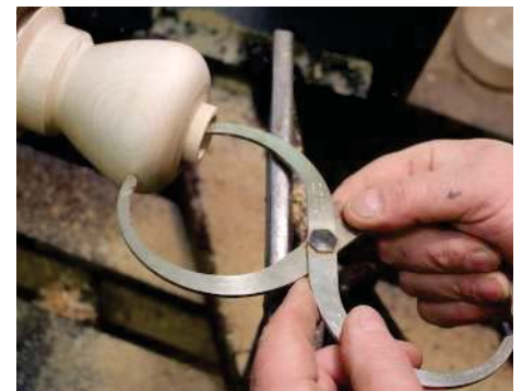
Checking wall thickness with callipers
