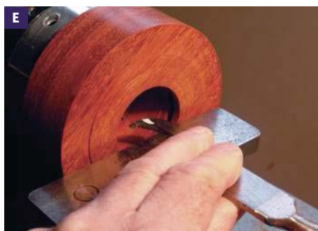
E Cutting the internal groove with the work held on expanded jaws
