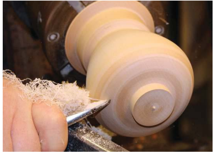
Negative rake scraping the surface
