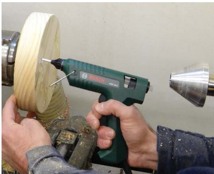
Applying glue to the backboard
