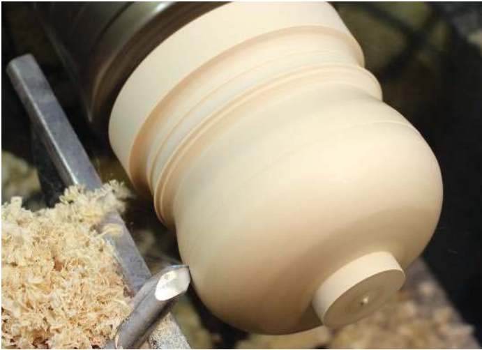
Shaping the part of the bottom section
