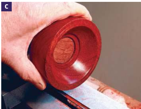
Testing the base on the turned end of the well cap
