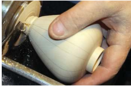
Parting off the vessel
