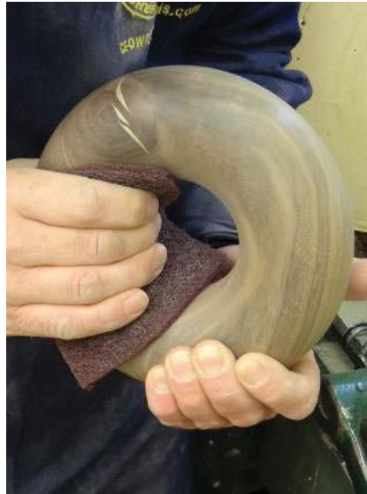
Final hand sand before oiling
