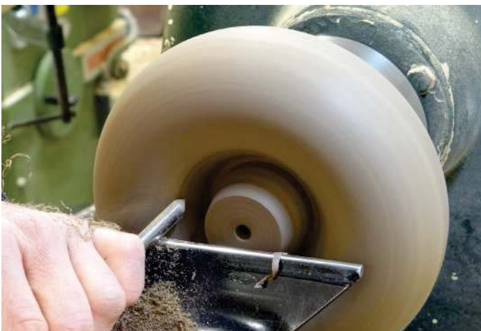
Using light shearing cuts with a spindle gouge
