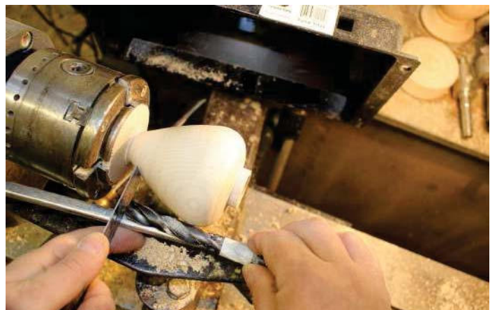
Marking interior depth on the outside
