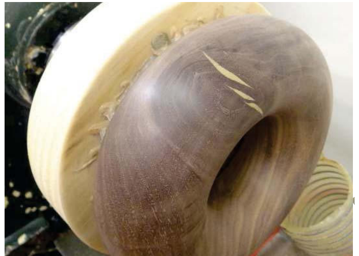
The result of filling the cracks
