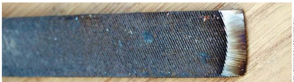
A home-made scraper which can present a real danger to the user
