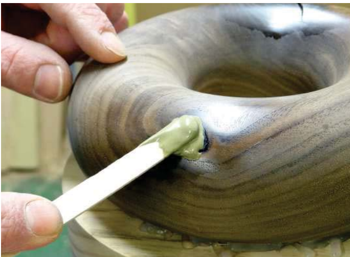
Applying the brass powder and epoxy mix
