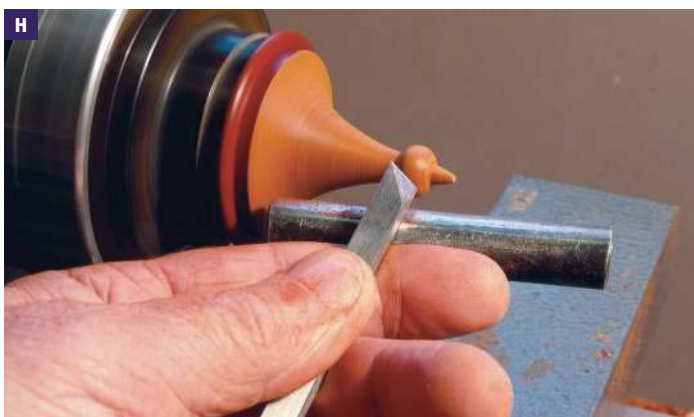
Completing the top of the well cap
