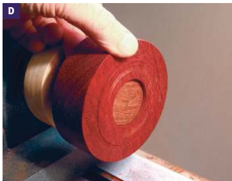
Check the turned step around the base against the turned collar of the well cap
