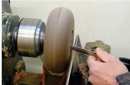
The parting tool cut into the face
