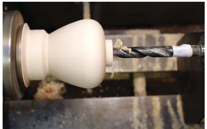
A twist drill bit on a morse taper is used to drill out the central core
