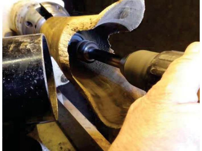
Sanding deep inside with an inflatable bowl sander fitted to an extension arm in a chuck
