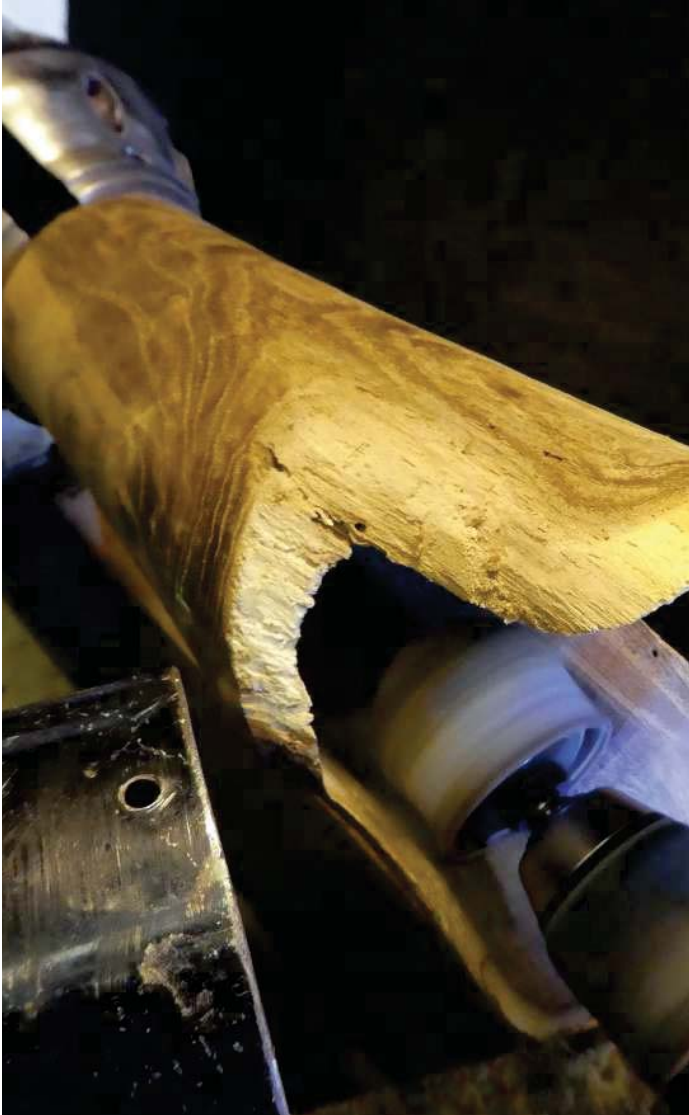
Sanding inside a smaller opening with an inflatable bowl sander
