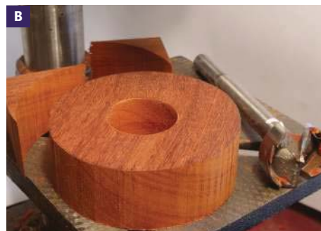
B The drilled square blank is cut round
