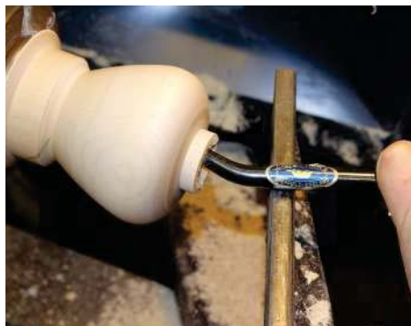
Using a carbide cutter-type tool to take cleaner cuts
