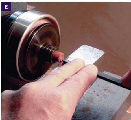
Turning the cup hollow in the end of the spindle, using a small round-nose tool
