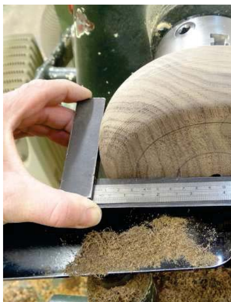
Marking the reverse side using a square
