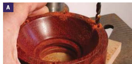
The holes around the top of the well are drilled
