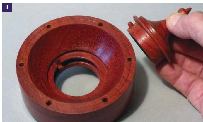
The dowel glued into the edge of the well cap
