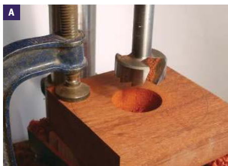
A The square blank is clamped in place while the central hole is drilled
