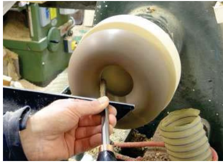
Blending the curves with a shearing cut with a spindle gouge
