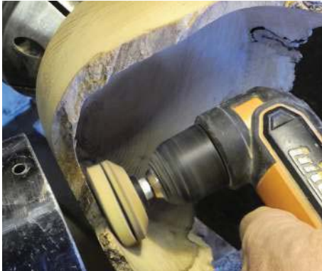
Sanding the inside surface
