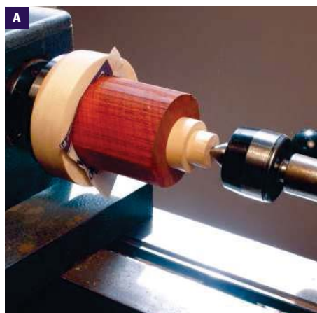
The well cap blank glued, with newspaper between, onto a wood faceplate
