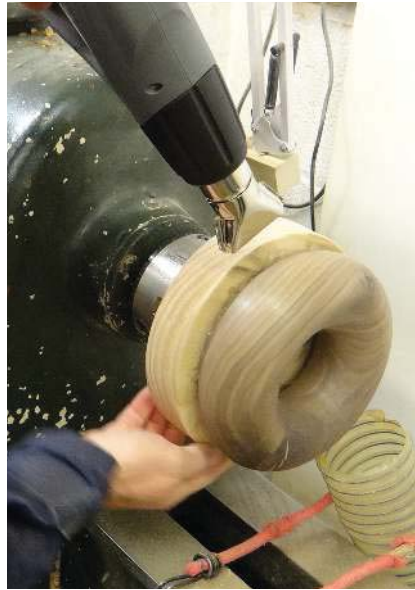
Applying heat to the glue-gun-chuck
