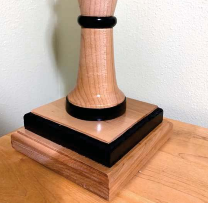
Masking off and the addition of small V-cuts minimises bleeding
