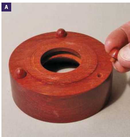
Fitting the turned feet in the base
