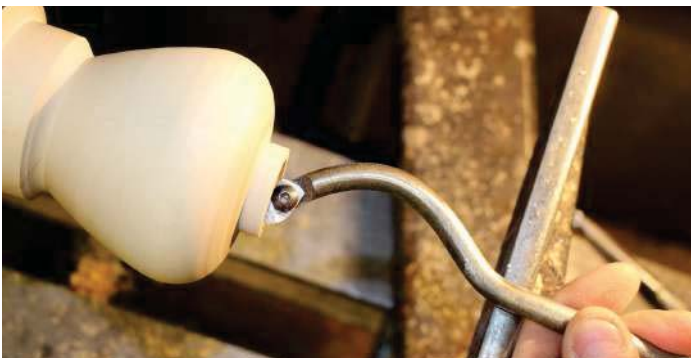
Using a swan-neck scraper tool to finish the interior surface
