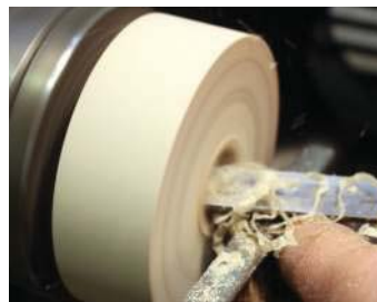
Hollowing the cap
