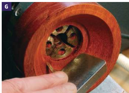
G Turning the internal step
