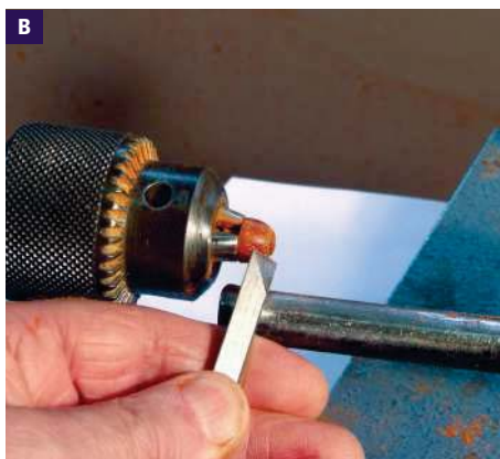
Turning the end of the feet
