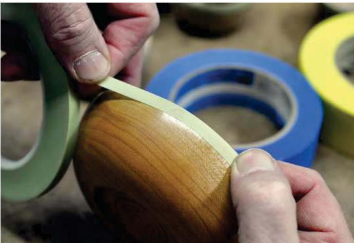
Masking off an area ready for the application of colour
