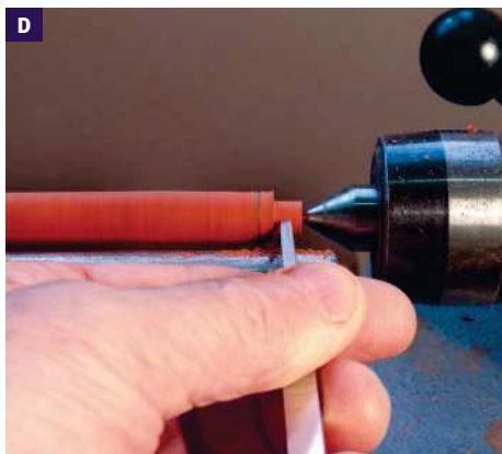
The spigot on the spindle end is turned
