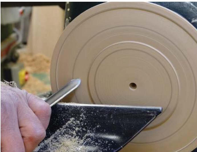
Turning the top surface of the beech bowl
