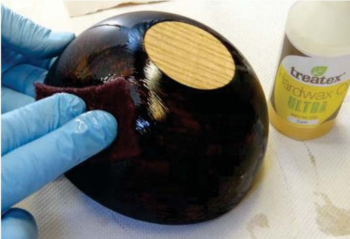
Applying hard wax oil to the ash bowl
