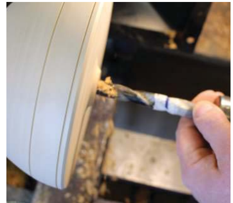
A twist drill bit on a morse taper is used to cut the central core
