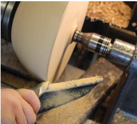
The edge of the top is chamfered to soften it and prevent chipping-out
