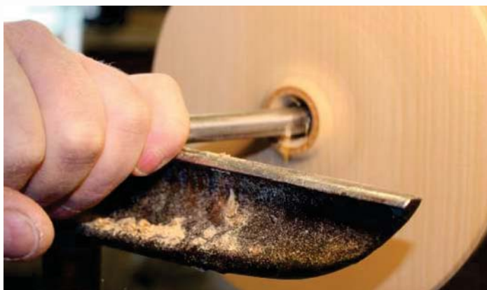
Opening the pre-drilled hole out
