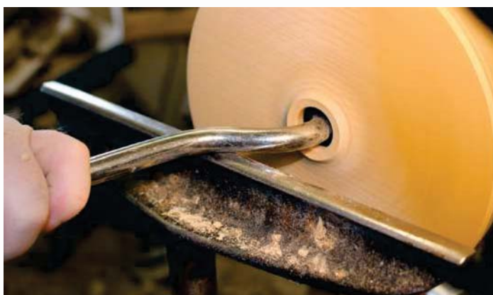
Using a swan-neck deep hollowing tool
