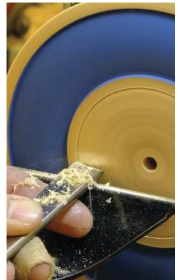
Cutting a groove with a skew
