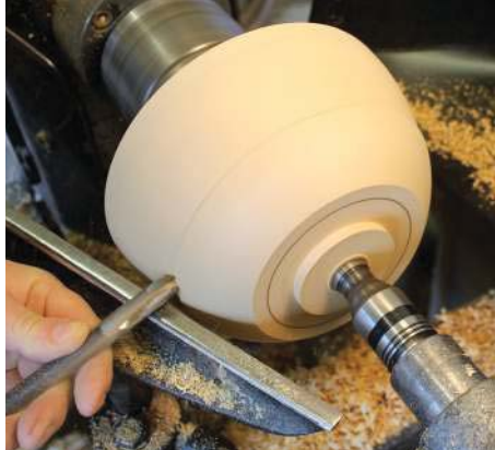
Base diameter marked and turning shape to it
