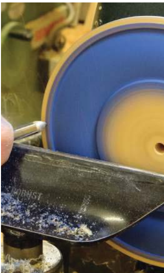
Removing excess paint
