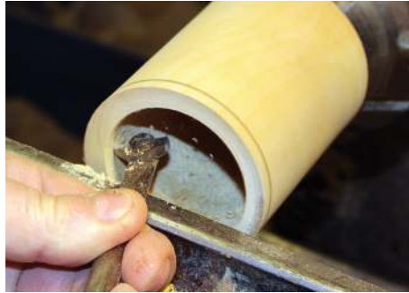
Modified scraper tip and a shop-made rebate tool
