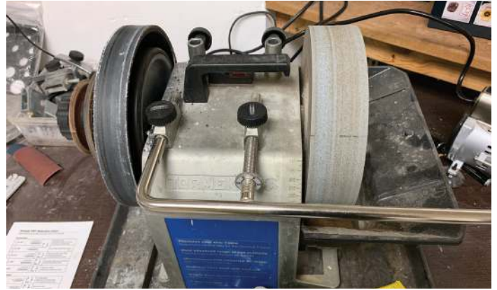
A wet grinder with leather honing system on the opposite side
