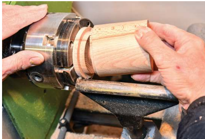
Use the waste as a jam chuck to reverse the box
