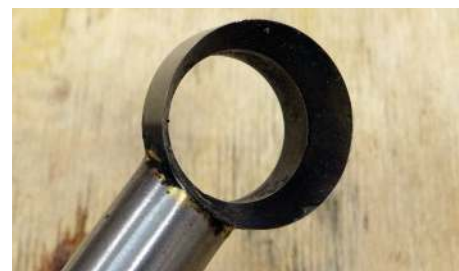
When light reflects from the edge it's a sure sign the tool needs sharpening
