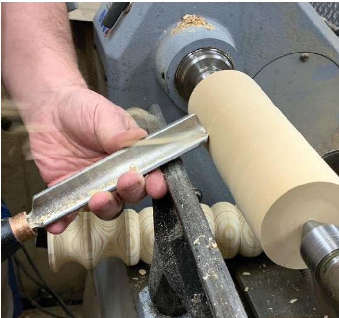
Spindle roughing gouge in use with the flute pointing in direction of cut and the cut occurring on the lower wing
