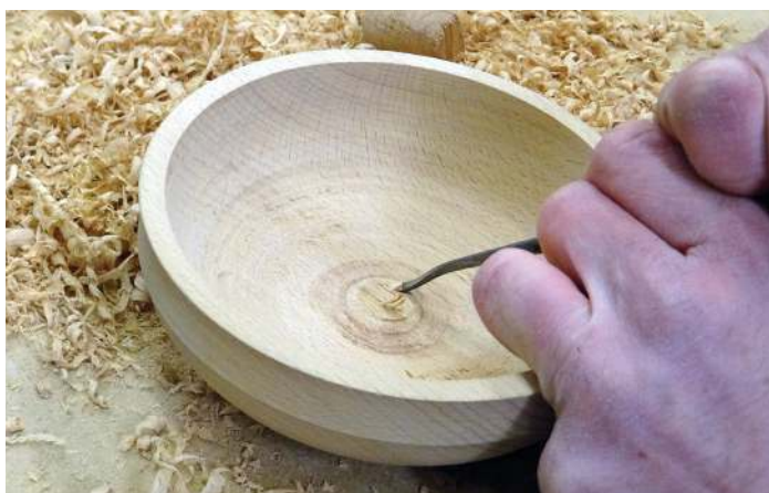
Cleaning the lower inner section with a bent carving tool
