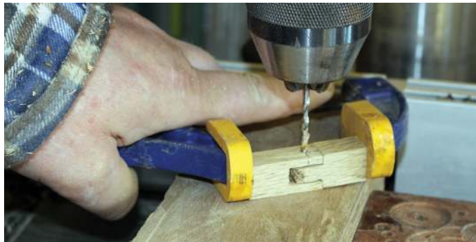
Drilling through for the pin
