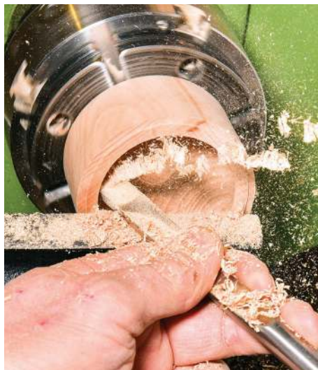
Hollowing small boxes can be accomplished with a spindle gouge
