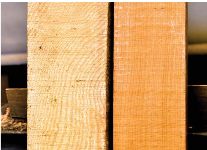
Straight grain blanks make lid grain matching easier
