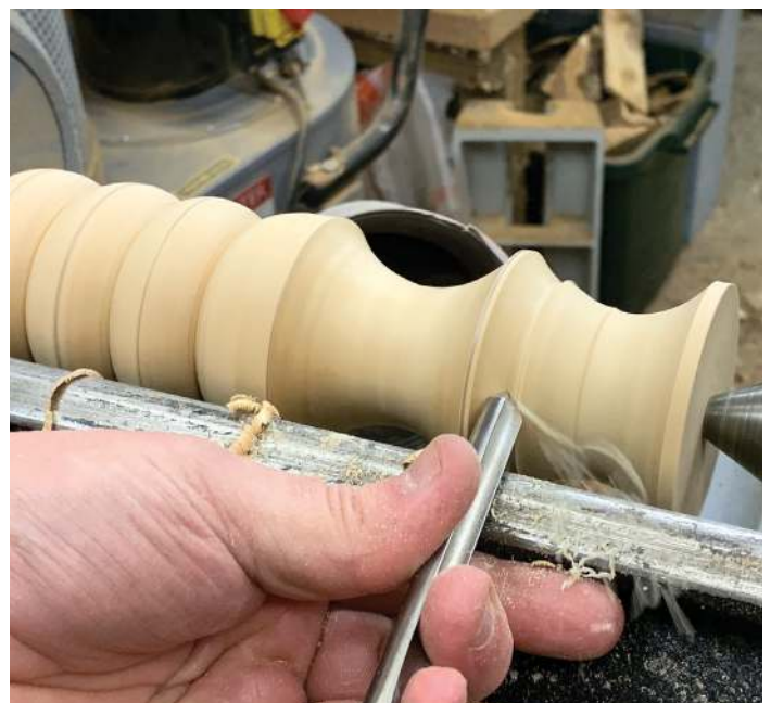
Using a spindle gouge to cut the coved sections
