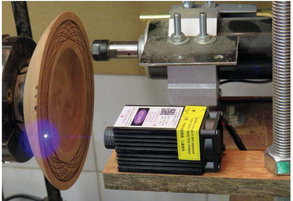
The laser diode mounted on a small piece of wood on a large threaded rod screwed to the compound table
