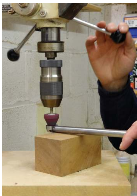
Polishing the inner bevel using the drill press
