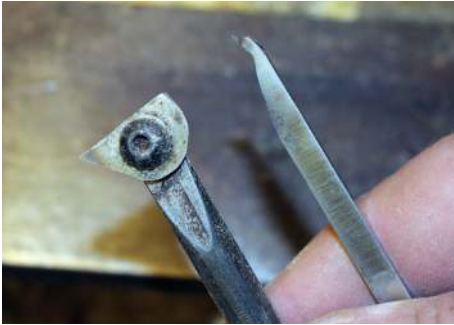
Modified scraper tip and a shop-made rebate tool
