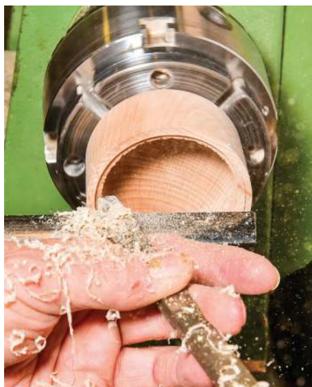
Creating a lid joint recess is easy with a box scraper
