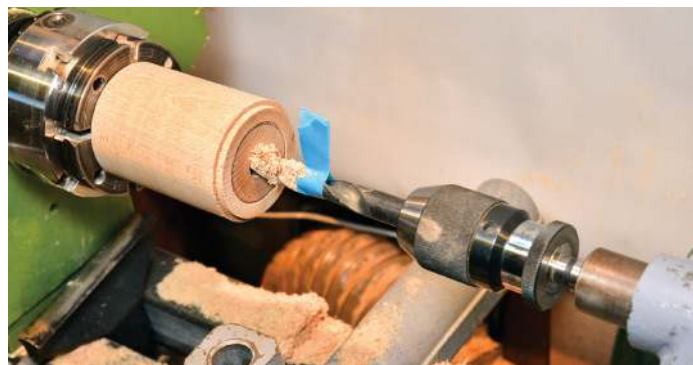
Drill the lid and box to set depth and to ease hollowing
