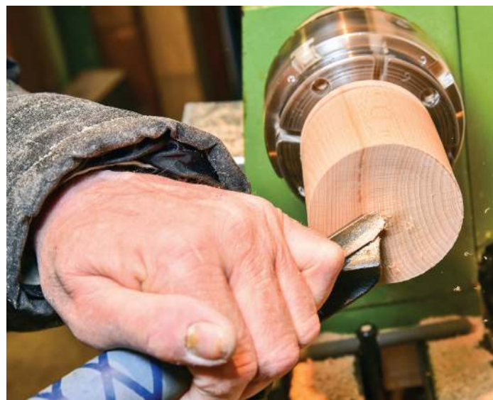
Finish the base on a jam chuck, removing the tailstock at the last moment
