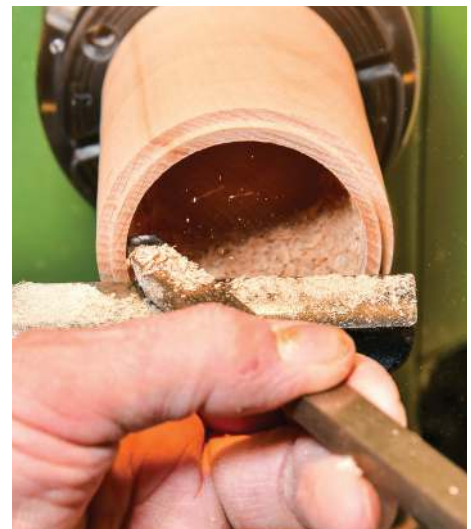
A box scraper helps create parallel walls and a perpendicular bottom
