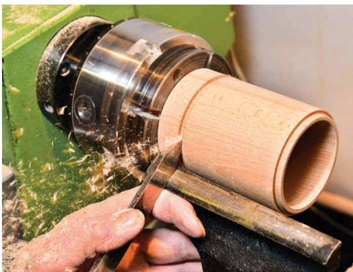
Part off the box by stepping down, stopping to saw off the nub
