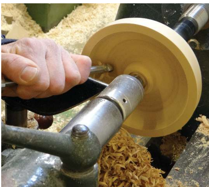
Working along the wall with the outer bevelled edge
