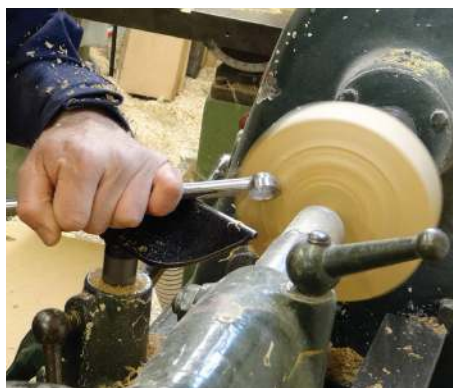
Dropping the handle produces a lighter, more shear, finishing cut
