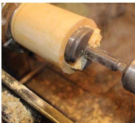
Roughing down and cutting a tenon
