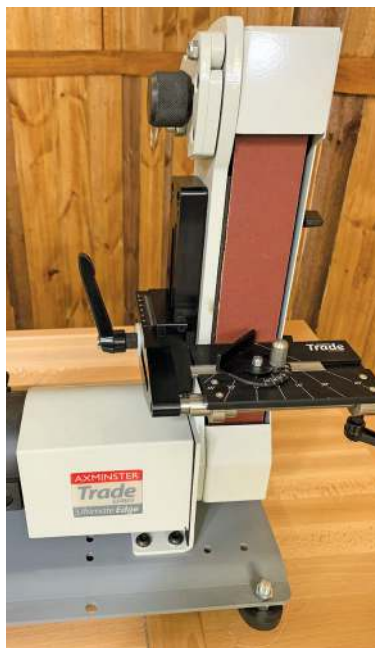
A belt finisher sharpener
