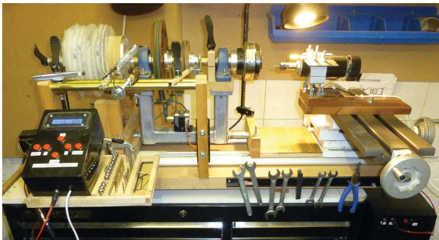
The homemade ornamental lathe
