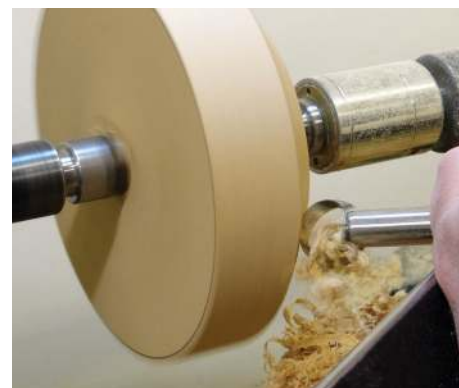
The ring tool in action
