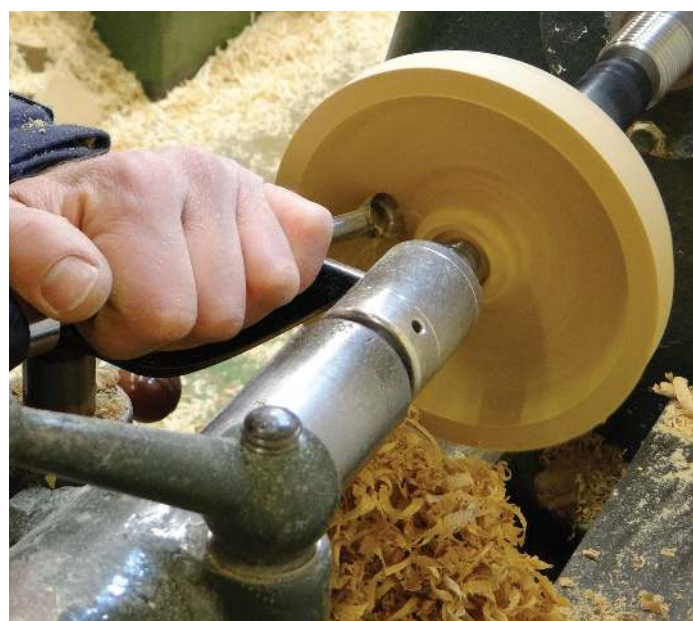
Cutting toward the centre with the inner bevelled edge
