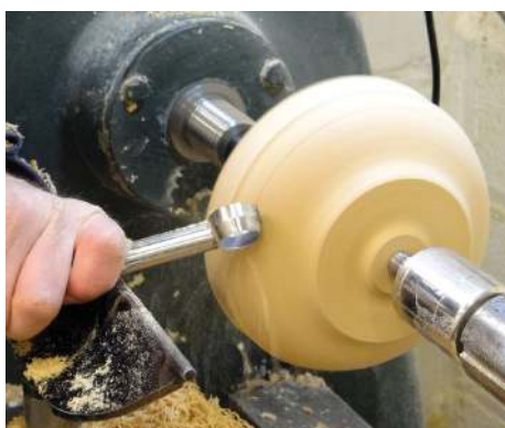
Shearing finishing cut on the outside
