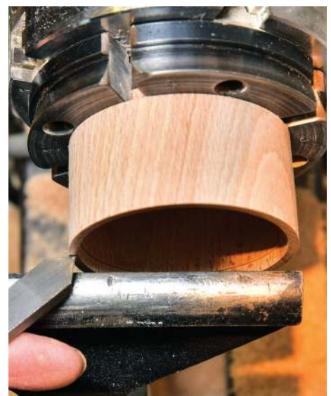
A dovetail scraper helps undercut the lid accurately
