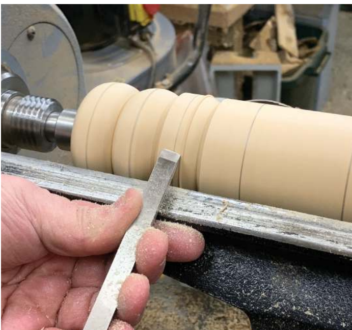
Use the corner of a beading and parting tool to peel the wood away
