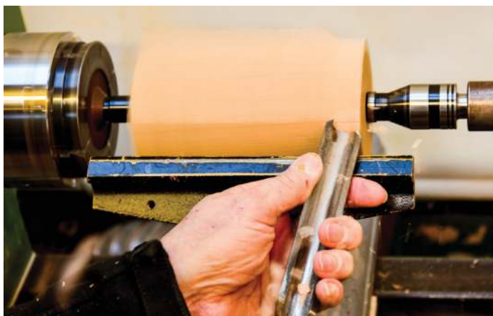
Rough to a cylinder in steps towards the ends
