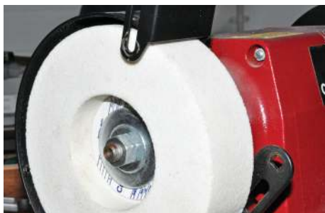
With the end enclosure guard removed the 'blotter' can be seen behind the securing flange and the top plate adjusted close to the wheel
