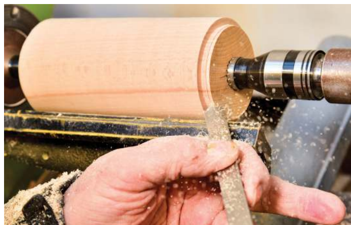
Creating chucking spigots both ends with a dovetail scraper
