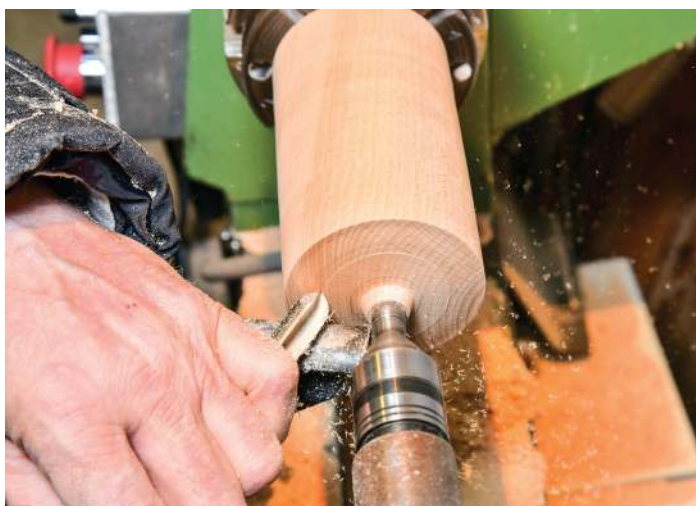
Jam the lid on the base and shape. Re-true the outside walls if necessary
