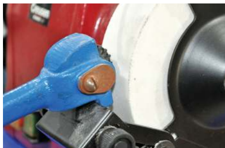
The correct way to use a toothed wheel-type dresser. The lugs should locate behind the toolrest and the handle gently raised to engage. This also helps to ensure a flat, accurate wheel surface
