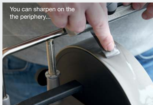
Gouge sharpening with the SVD-186 Gouge Jig.
