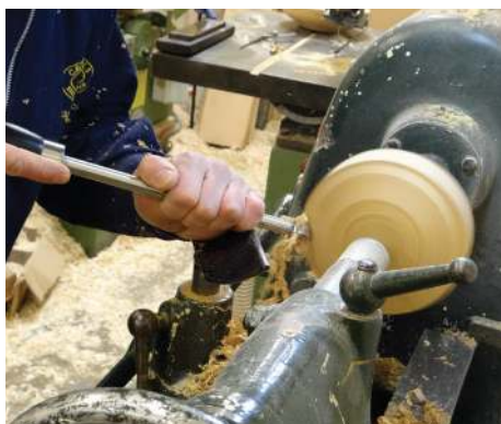
Turning with the tool handle tucked under my arm and the cutting edge trailing
