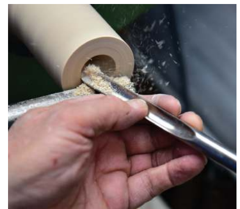
Hollowing with the lower tip of the spindle gouge
