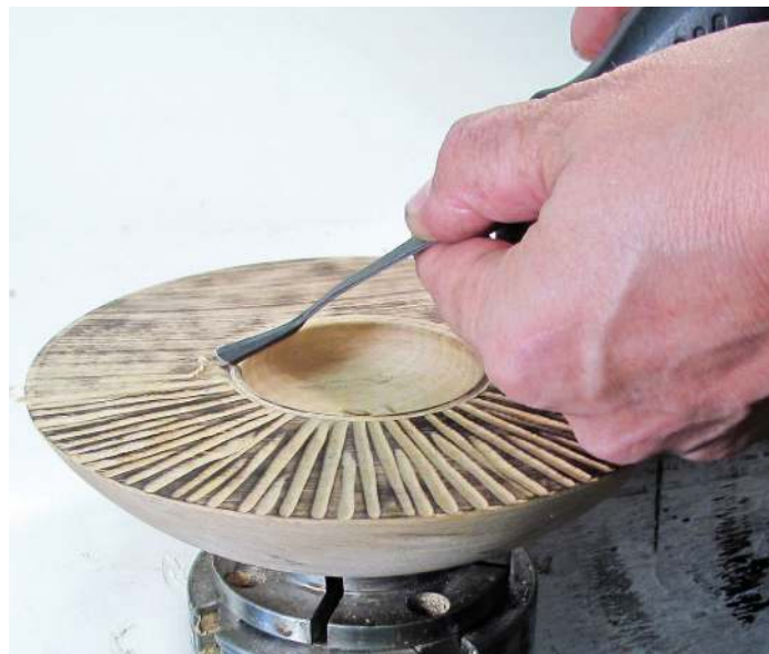
The work is held on the chuck, but the chuck is held in wooden jaws to give better access
