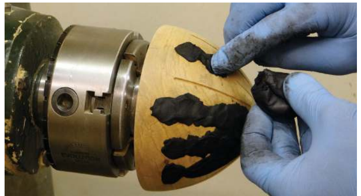
Applying the putty to the grooves
