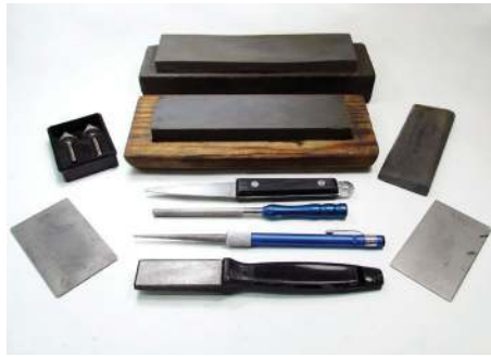
Wet/oil stones and hones of various shapes help shape and maintain the bevel and cutting edge
