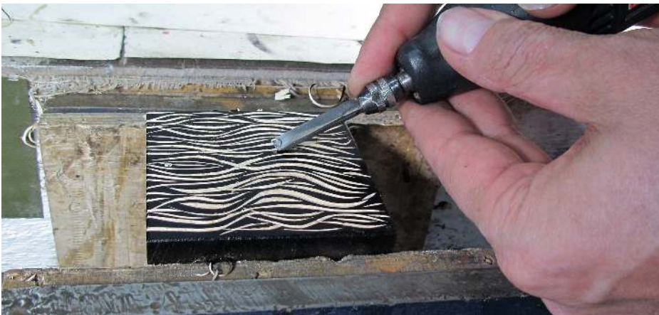
The power carving unit fitted with a V-gouge being used to create a wavy, s-like pattern on timber sprayed black
