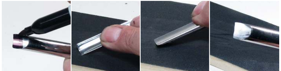
Mark the bevel with a colour marker, then lay the bevel of the gouge flat on the abrasive and work the flat face or, in this instance, with a curved gouge rotate the blade to one side and then, as you draw the gouge back along the abrasive, rotate it until you reach the other side of the curved bevel
