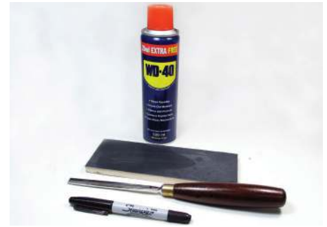
Diamond stone with lubricant helps with shaping and maintaining the bevel
