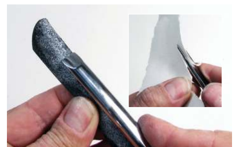
A shaped hone, working down using ever-finer abrasive grades, is used to refine the inside curve. Once sharpened it should cut paper
