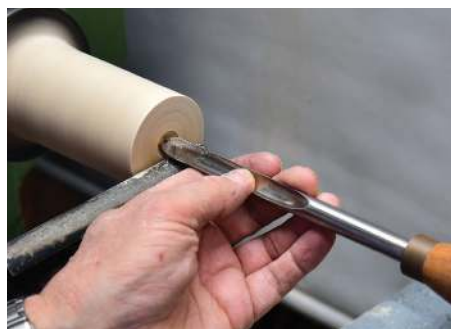
Start on centre and wiggle the gouge for clearance
