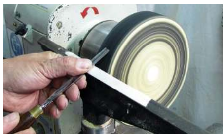
SAFETY WARNING: If sharpening, honing or stropping on a lathe, reverse the rotation of the lathe spindle so the wheels run away from the cutting edge
