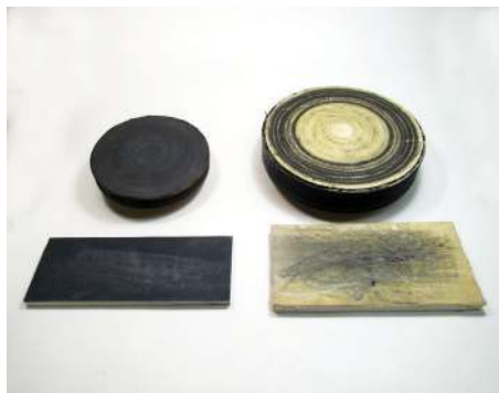
Honing discs for mounting on a lathe and leather strops for stropping an ultra-sharp edge
