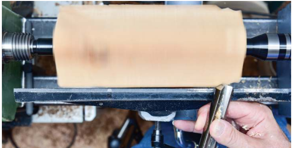
Gouge presentation angle with flute in direction of travel
