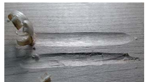
A freshly sharpened tool will cut wood cleanly when cutting with the grain. One needing stropping will not
