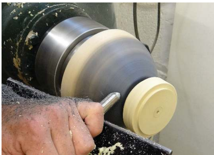
The glue chuck is turned and the Milliput turns well
