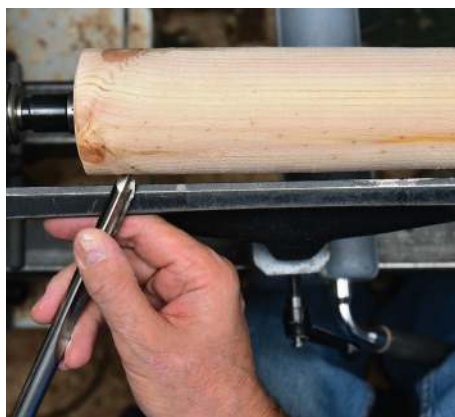
Turning left and right handed is a useful skill, start on a cylinder
