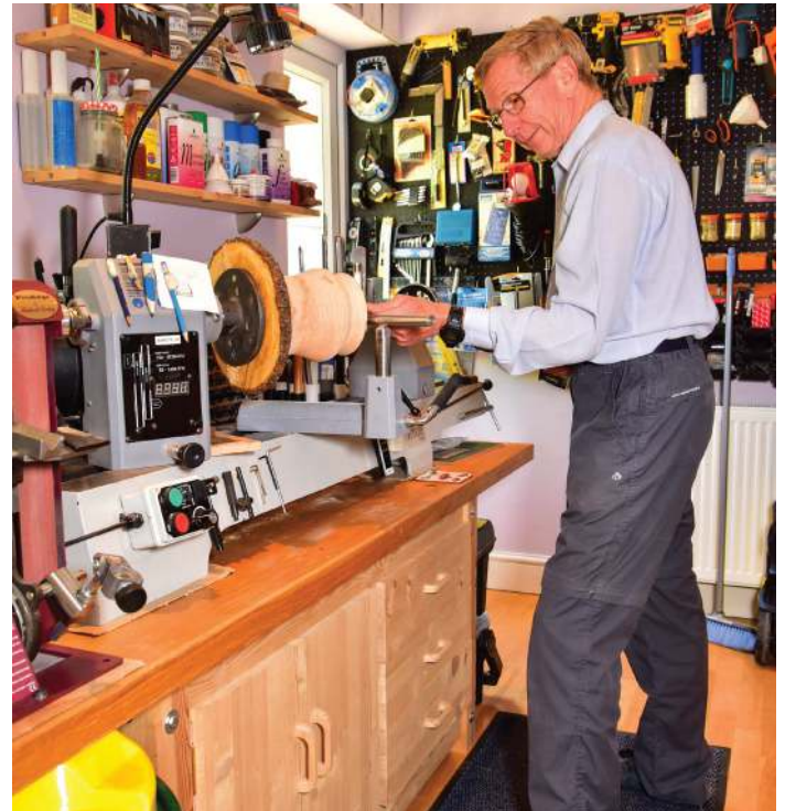
Ensure a stable, comfortable stance. Note: No one is turning in this picture, the work is stationary and shows a typical working stance, therefore the person is not wearing safety equipment
