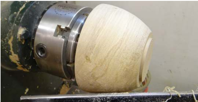
Using my standard-size tenon leads to a bowl with a fat bottom
