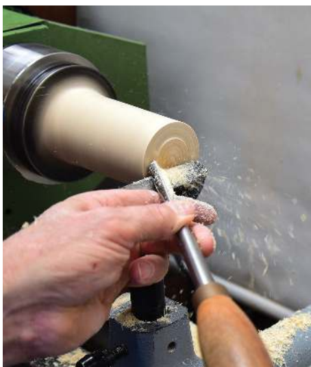
Cleaning the end with a spindle gouge leaves a good finish
