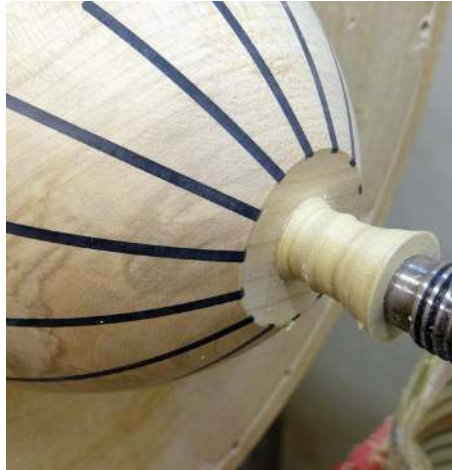
The base section ready for final adjustment off-lathe
