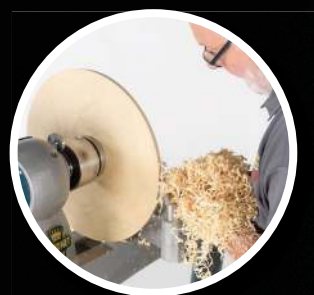
Features the latest motor technology to deliver huge amounts of torque from the 750 W output motor
