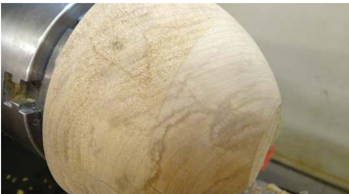
Marked improvement in the quality of the surface with the push cut
