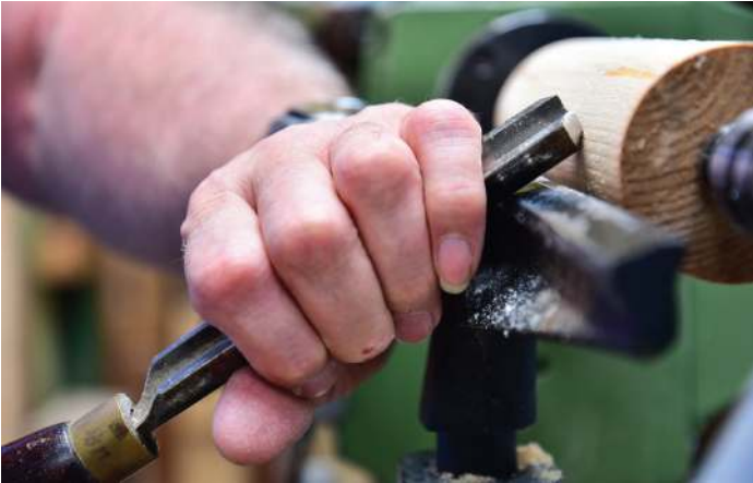
Toolrest lower than centre facilitates comfortable bevel rub
