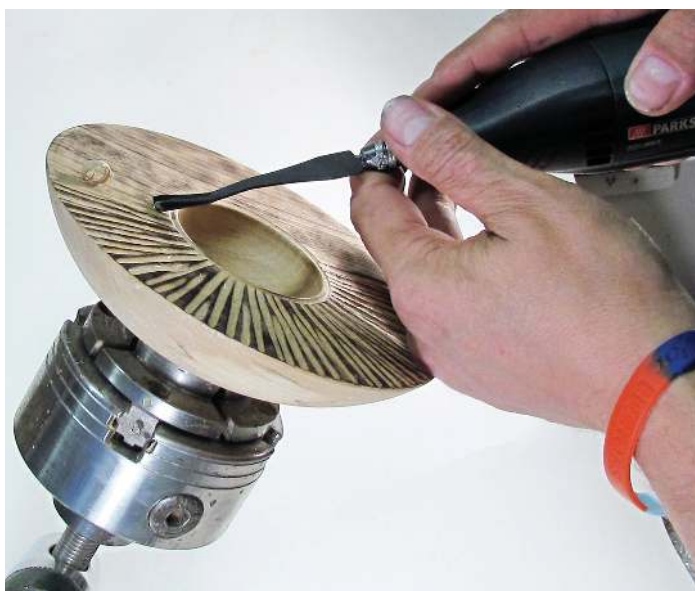
Work held in a chuck on a carver's vice, which has a threaded spindle to suit the chuck
