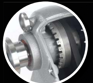
Heavy-duty spindle lock and 24 point indexing
