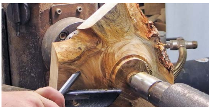
Shear cutting to reduce tear-out
