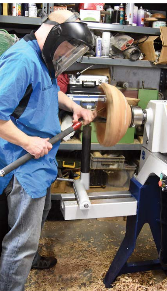
Turning a burr with bed extension with riser post
