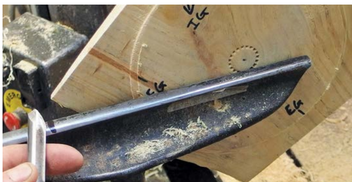
Cutting the upper face flat
