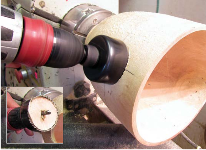
Using a hole saw INSET: The disc of timber removed
