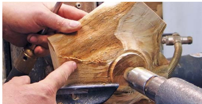
Tear-out on the trailing edges
