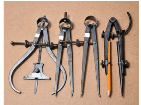
Callipers and other measuring devices used when making turnings to size or duplicating items
