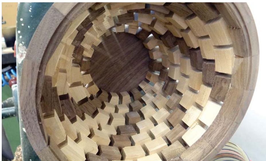
Briefly holding the bowl in place while the glue grabs before adding weights
