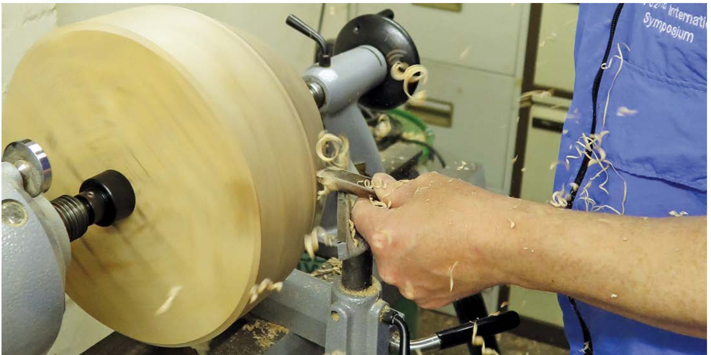
Turning a bowl between a ring centre and a tailstock centre with belt tension adjusted too
