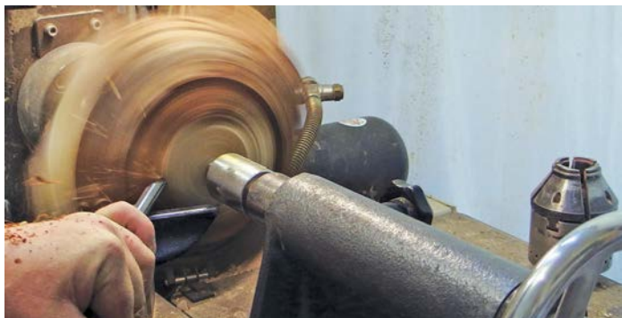
Roughing down with a pull cut
