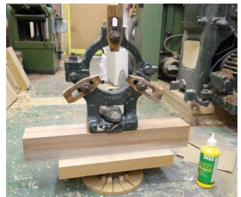
Heavy weights used to clamp the glue-up together
