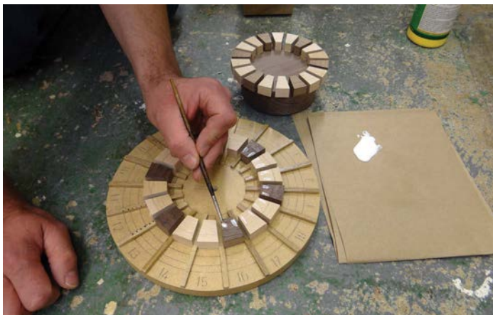
Careful glue placement for the next open ring
