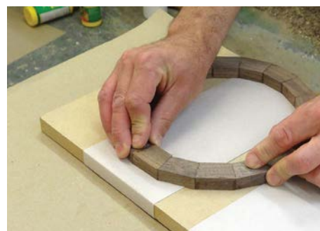
Flattening before final glue-up
