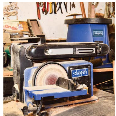
Sanders are useful for ancillary operations – disc, belt and bobbin illustrated
