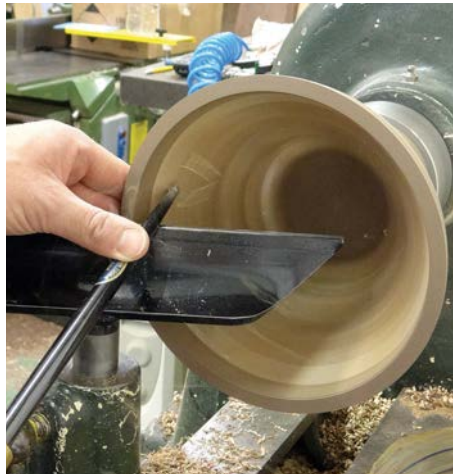
Contour-ground carbide-tip tool in use
