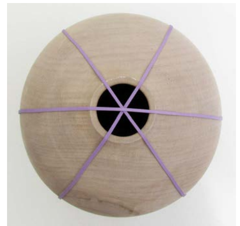
Elastic band help when marking curved surfaces
