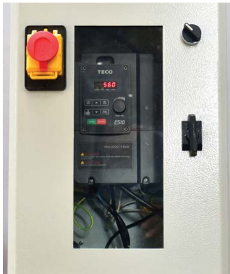
Inverters control speed & reversing – remote pendants can be positioned for safe operation
