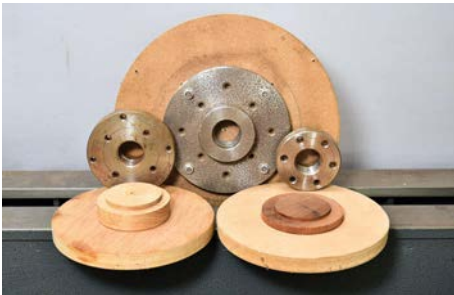
Faceplates are a very secure holding device and can be made to size in wood
