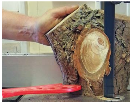
Trimming to create a flat base
