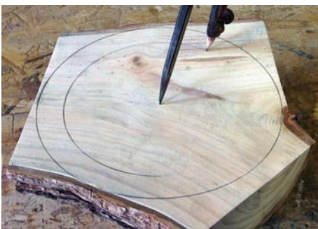
Marking dead centre for balance
