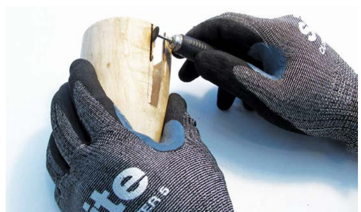
Using a saw-type burr to cut work
