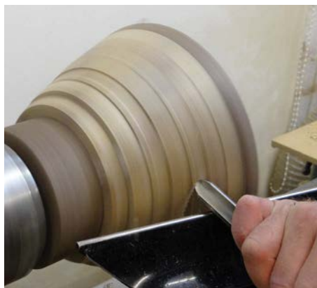
Initial cutting with bowl gouge
