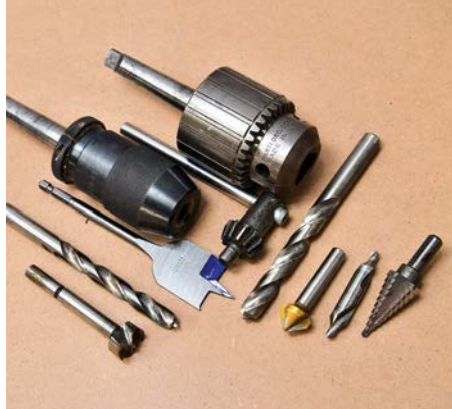
Drill chucks are available keyed or keyless and many bit types are available
