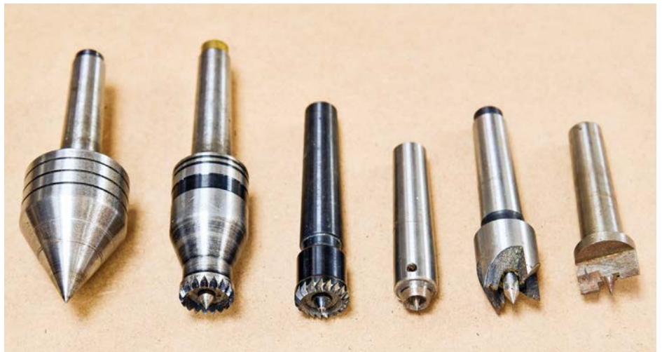
Centres from left to right: live, revolving, crown, ring, four-prong & two-prong drives/drive spurs
