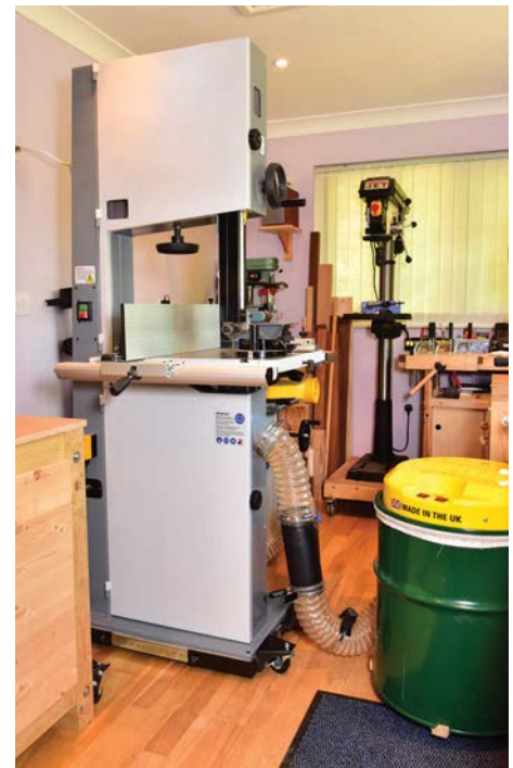
A bandsaw is the most versatile saw for woodturners. A drill press is very useful, as seen in the background, but a hand drill in a stand will perform most tasks required
