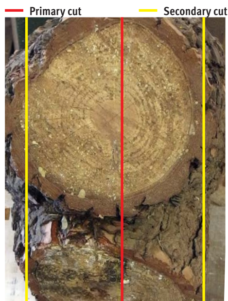
Cut lines to reveal figure
