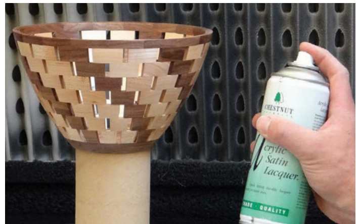
Spraying acrylic lacquer finish
