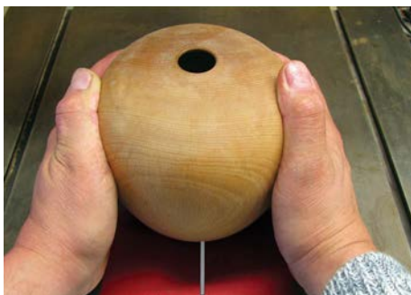
What not to do when cutting an unstable form. This picture was staged as what not to do, with the bandsaw switched off
