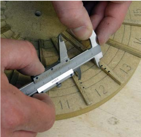
Measuring the size of each segment
