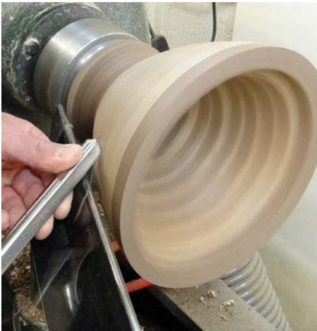
Shear cutting the outside of the bowl
