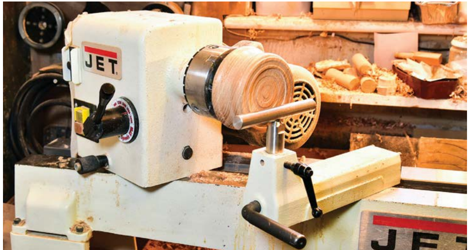
Swivel headstocks allow more comfortable working and larger diameter workpieces
