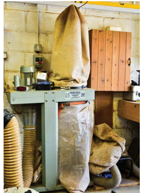
Good extraction helps remove chips, but dust protection is also necessary
