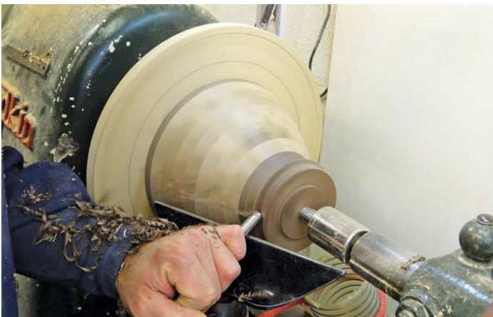
Reverse turning the base
