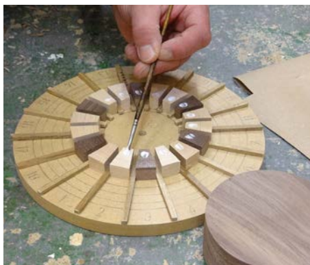
Gluing the walnut base to the first ring of segments
