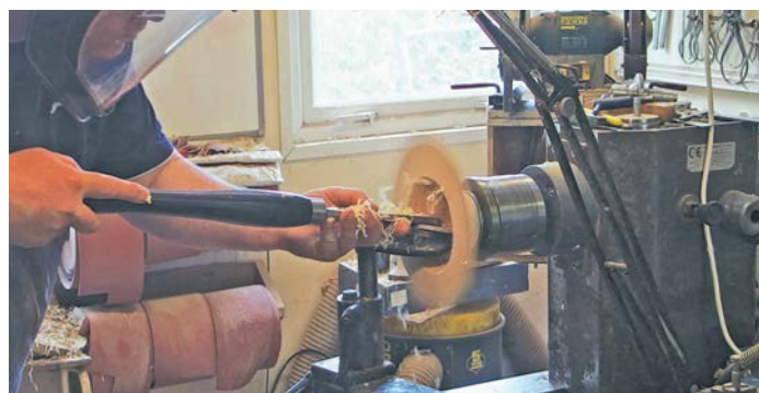
Turning the inside of the bowl
