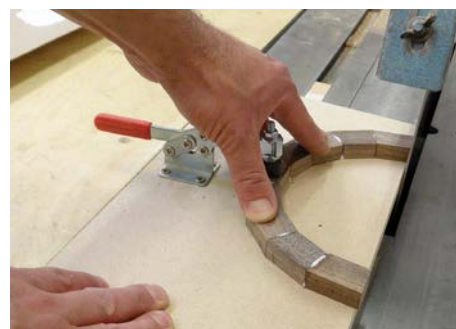
Truing up the joining faces of the two semi-circles
