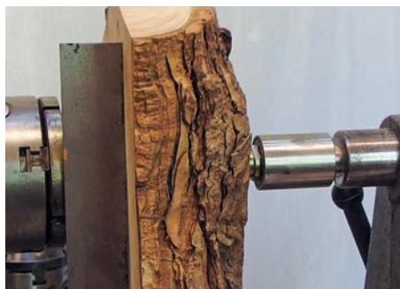
Mounting the work centrally between centres
