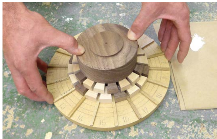
Briefly holding the bowl in place while the glue grabs before adding weights
