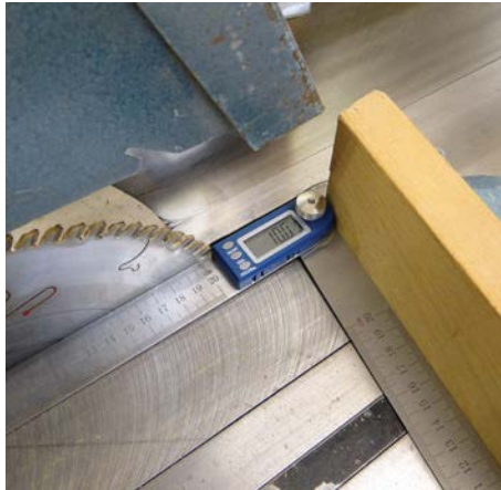
Setting the mitre fence to 10°
