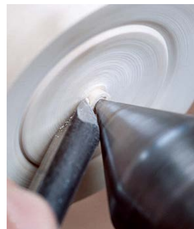
A 10mm shallow gouge is the best tool for working across the base and around the tail-centre cone
