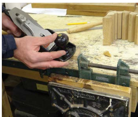
Using a hand plane to adjust the angles
