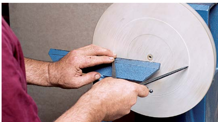
2 Mark the diameter on the jam chuck
