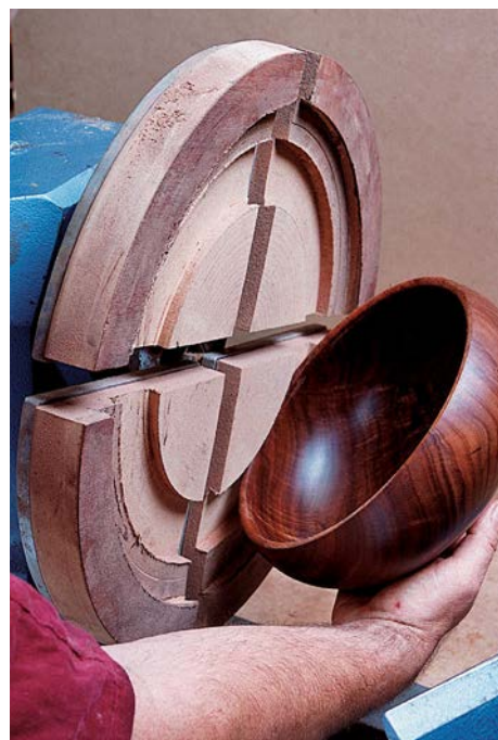
On these smaller bowl jaws, I've replaced the buttons with MDF cut to match the jaws. By opening the jaws wide before turning the recess, I extend the range over which the chuck can grip around a rim
