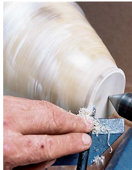
This thin box elder bowl being mounted over a bowl profile with tail-centre support is wrapped in cling wrap to keep it from flying apart
