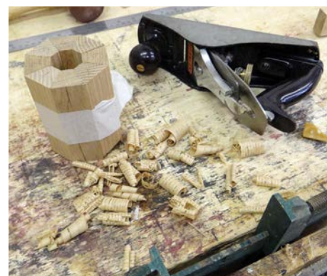
Now dry fitted together perfectly, with the sum total of the shavings I had to remove to achieve the fit
