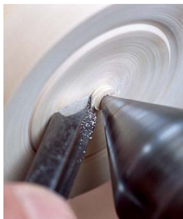
A 10mm shallow gouge is the best tool for working across the base and around the tail-centre cone
