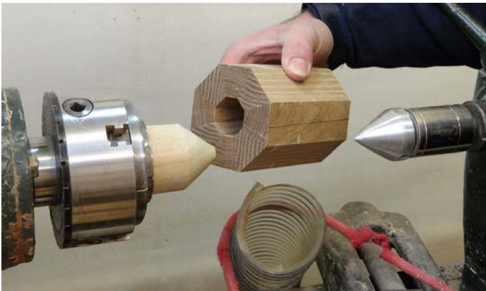
Mounting the blank between tapered centres
