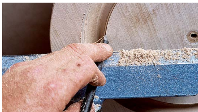
3 Cut a light taper into the chuck. Think in terms of 1°. Make the bottom of the shoulder slightly fatter than the top so the bowl fits on to the tenon with a slight grating sound
