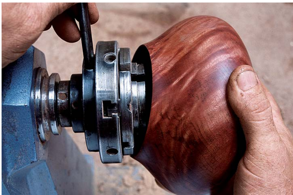
Small bowls are easily mounted over expanding jaws. If the rim of the bowl is against the chuck, the bowl should run true
