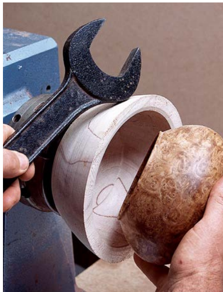
If a bowl is difficult to remove from a jam chuck, firmly tap the chuck with something heavy, and the bowl should drop free
