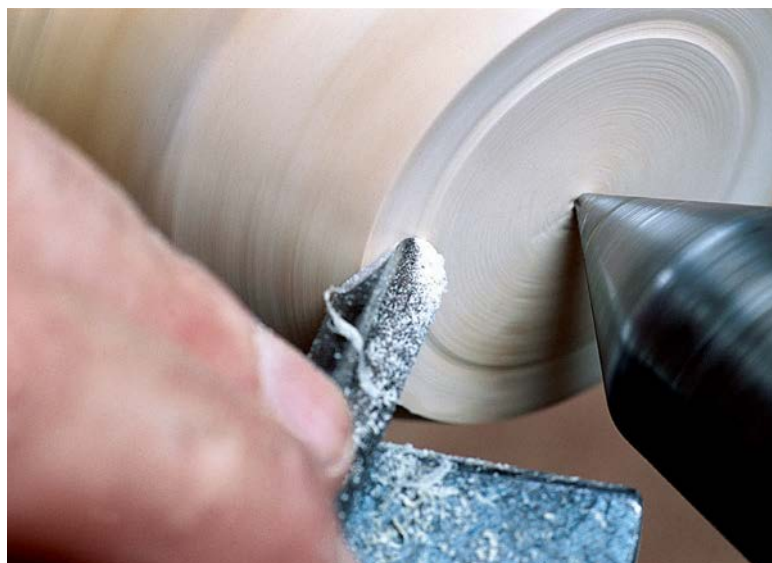
This thin box elder bowl being mounted over a bowl profile with tail-centre support is wrapped in cling wrap to keep it from flying apart
