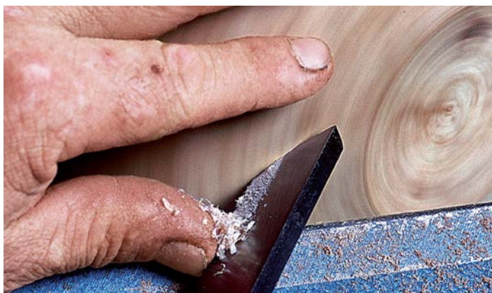
6 Complete the profile with a shear-scrape, and blend the new surface with the old
