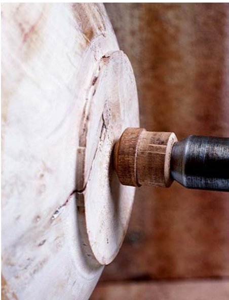
A flat tail centre is useful when the base is thin or finished. Flat centres are commercially available, but it's easy to turn your own to fit over your conical or cup centres
