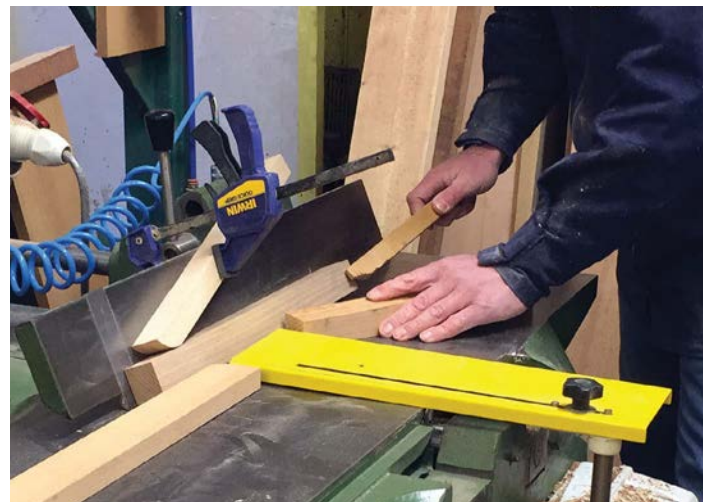
Machining the angle on the timber
