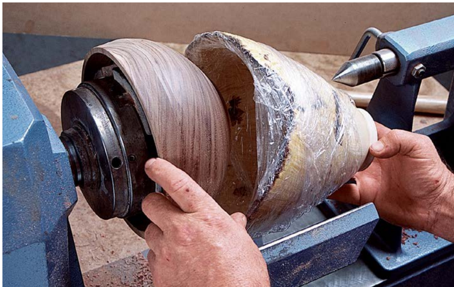
This thin box elder bowl being mounted over a bowl profile with tail-centre support is wrapped in cling wrap to keep it from flying apart
