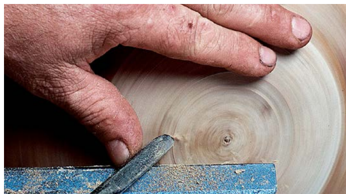
5 Then turn the base slightly concave, cutting toward centre from the rim
