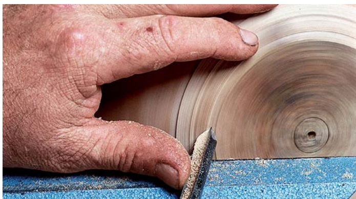
4 Mount the bowl, then use a \frac{3}{8} in (9mm) shallow gouge and small arcing cuts to remove the waste around the rim of the foot, working from smaller to larger diameter
