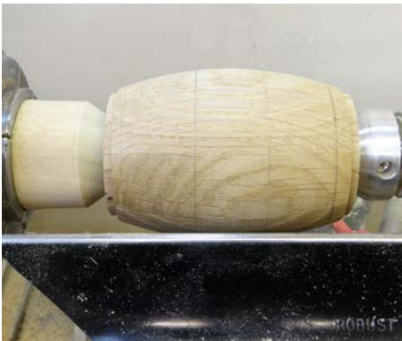
Barrel marked out and ready to part
