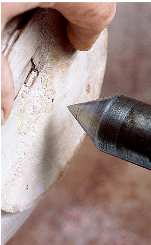
Putting a dot at the centre when you are completing your profile makes centring a bowl over a vacuum chuck or between centres easy – just align the dot with the tail centre
