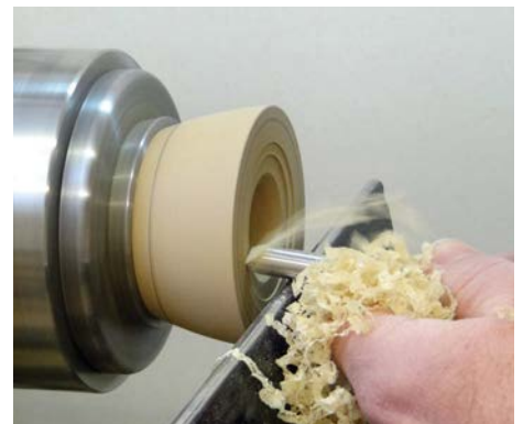
Cutting the recess in the base with a negative rake scraper
