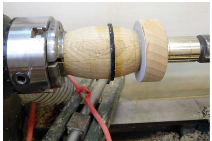
Using the lathe to apply pressure while the glue dries
