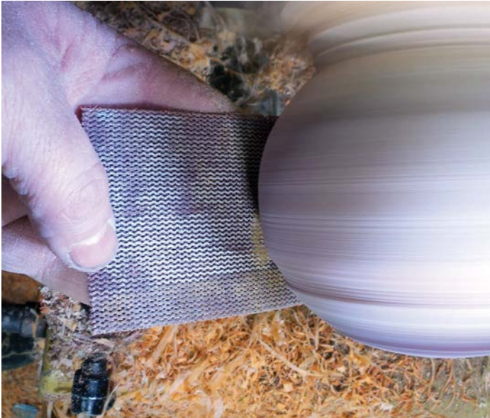
Coarse abrasive removes the damage quickly
