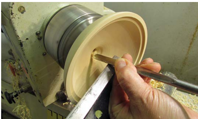
A gouge or scraper can be used to refine the inner form
