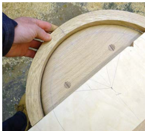
Setting out the positions of the back spindles
