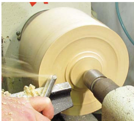
A pull cut to rough shape the base area
