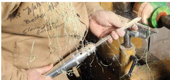
Bowl gouge shaping the outside of a hollow form
