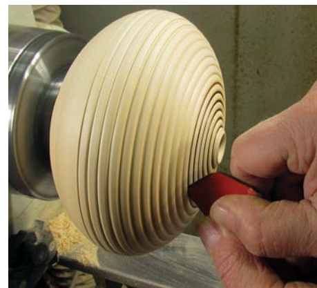
More groove cuts and burning in detail lines
