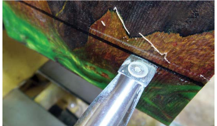
The radiused square cutter I use for roughing and shaping
