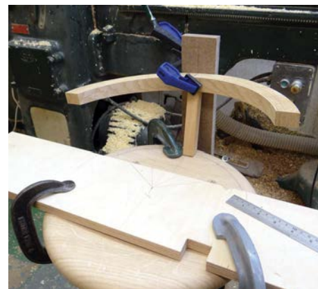
Mock-up including a spindle to check the angles
