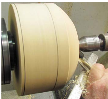
A push cut refines the surface
