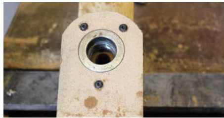
Counter-balance jig attached to chuck
