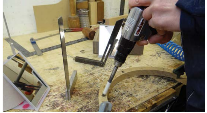
Drilling the backrest using 'the mirror trick'
