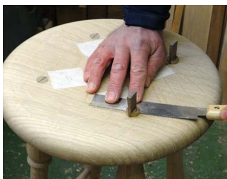
Trimming the tenons with a flush cutting saw
