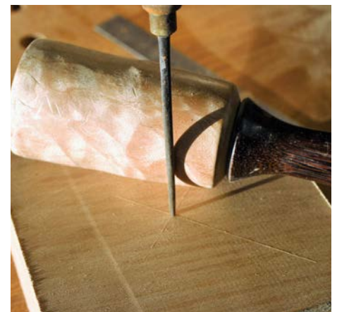
Using a marking knife to ensure accuracy when centring
