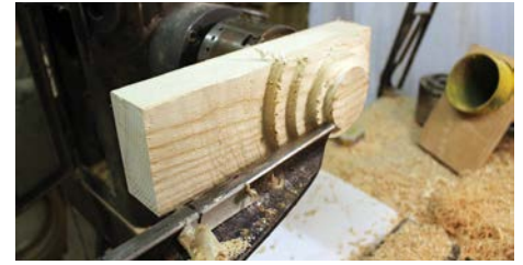
Off-set blank mounted on Forstner bit recess using expanding jaws
