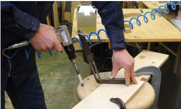
Drilling the seat using a mirror and sightline with a sliding bevel
