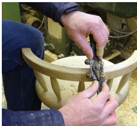
Adding curves to the backrest with a spokeshave
