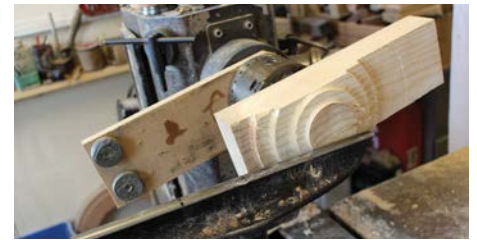
Lead weights screwed to jig to balance off-set blank
