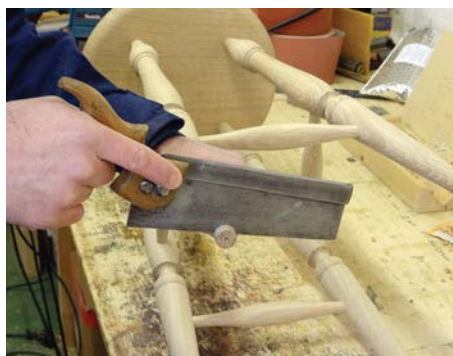
Sawing the legs to length
