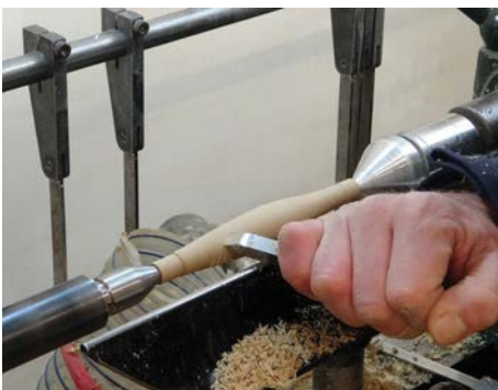
Planing cuts on the back spindles
