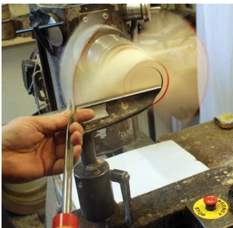
The ghost image of a piece of square-edged work
