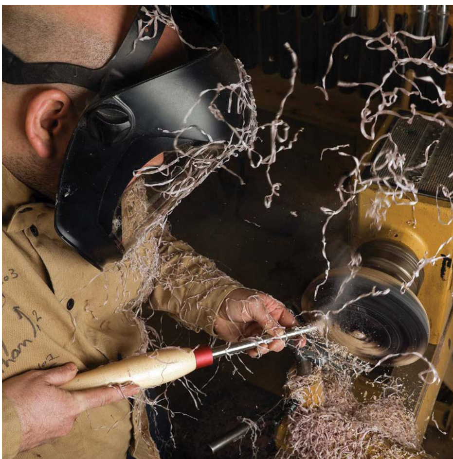
Working on a faceplate-oriented blank with a tipped tool wearing face protection and using a round cutter to refine the shape of the inside
