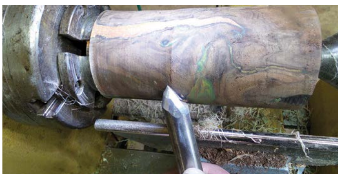
Bowl gouge used to make a shear cut using the wings of a gouge much like a skew chisel
