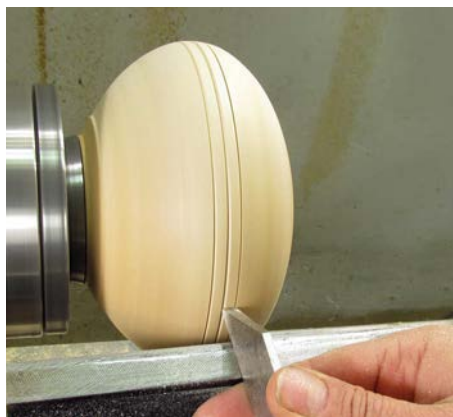
A forming tool cutting a groove on the join
