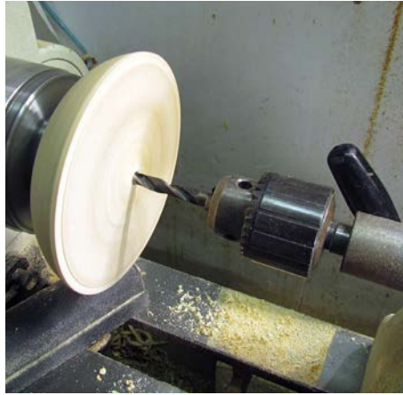
Drilling a hole all through the top section
