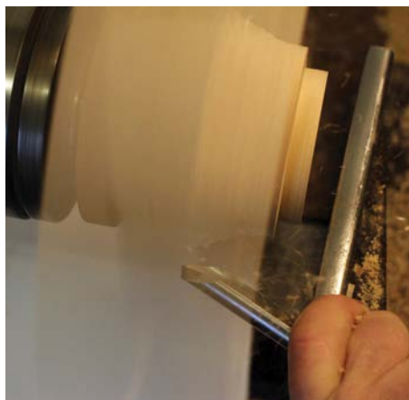
The bevel directing the cut
