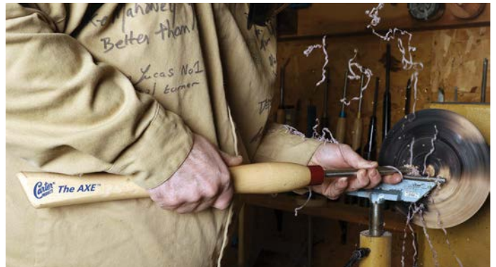
The radiused square cutter I use for roughing and shaping
