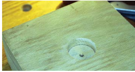
Bored hole ready for pin jaws, but the hole can be a large diameter hole to suit larger diameter jaws
