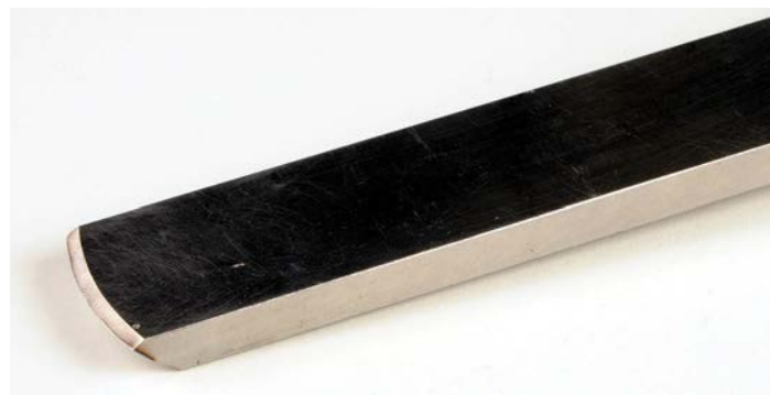
Conventional scrapers work well when used in trailing mode, but you might find that negative rake scrapers can be even more effective
