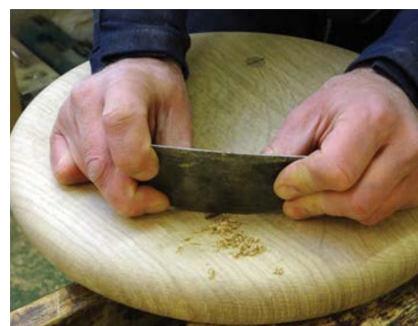
Using a cabinet scraper to finish the tops of the tenons
