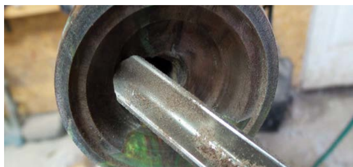
A spindle gouge being used to hollow out the end of a box, working from the lowest out and up to the top edge
