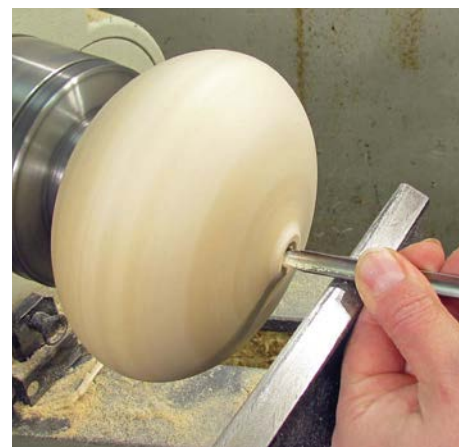
Spigot removed and the rim and opening shaped
