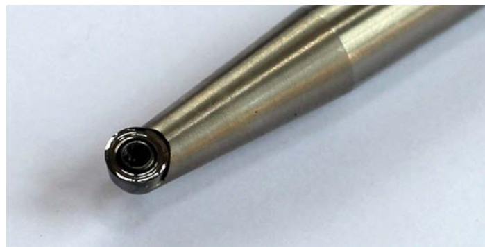
Round cutter, which has a groove behind the cutting edge on a round bar
