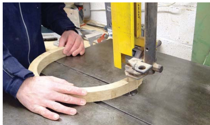
Cutting off the ends of the bent lamination
