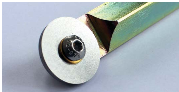
HSS scraper tips come on various sizes and shapes. Pick a shape of cutter that suits the area being refined. Some are mounted on round bars, square or set at an angle to cut in shear cut mode only
