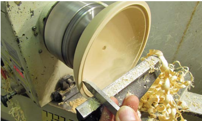
Creating the recess with a parting tool
