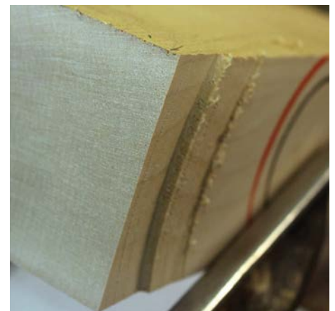
Work down in steps
