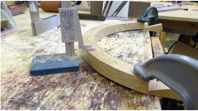
Using the height gauge to check the backrest is sitting flat and level on the bench
