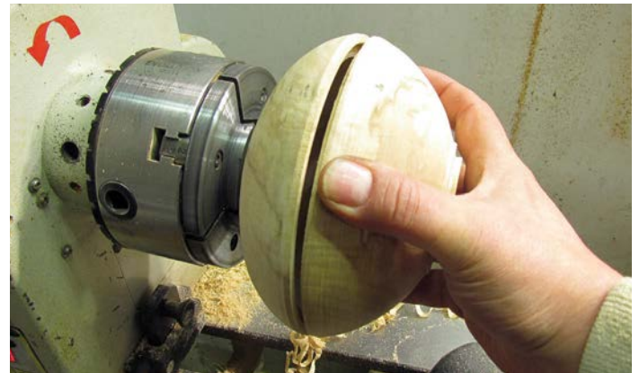
Checking the fit of the base to top section
