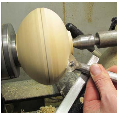
The vessel reversed and the top being refined
