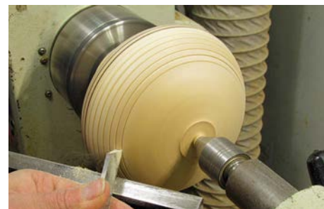
The piece secured and extra grooves added
