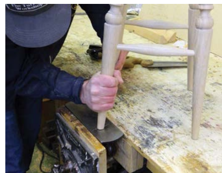
Trimming the legs with an upturned plane held in the vice
