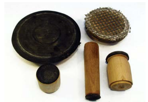
Various friction drives to support the work when the work is reversed and mounted between centres to deal with the base
