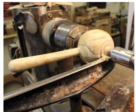
Turning a tenon to remount
