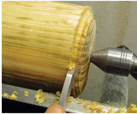
Cutting a spigot with a parting tool and cutting a spigot with a gouge
