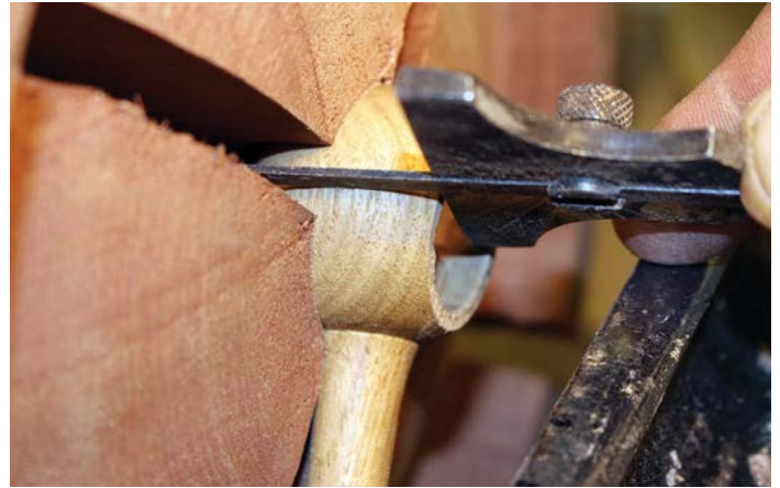
Checking for depth/wall thickness
