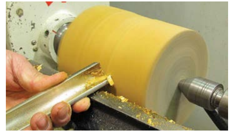
Spindle roughing gouge roughing down a cylinder. Note the fingers are not blocking the exit route of the shavings/wood chips along the flute
