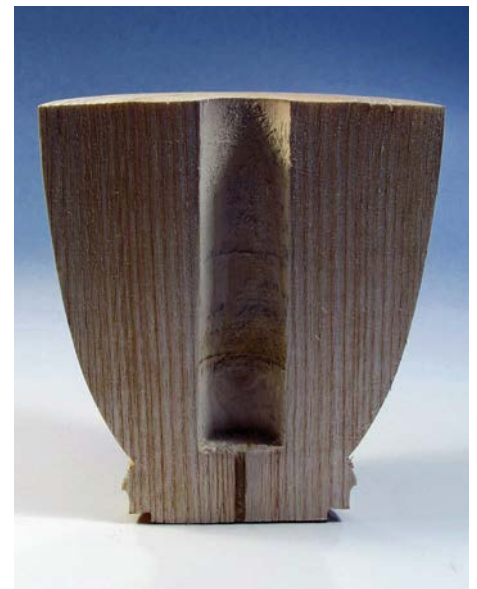
A piece cut in half after drilling. Note how the pith was centrally aligned
