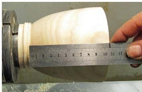
The piece mounted in the chuck and the top of the vessel cleaned up with a gouge
