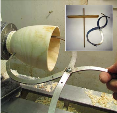
A depth and wall gauge are helpful to assess what is happening with the wall thickness and depth of the inside
