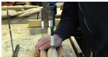
Drilling the mortises for the stretchers using 'the mirror trick'
