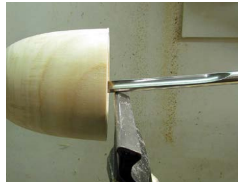
The gouge tip aligned with the centre and flute pointing at the 10 o'clock position ready for cutting
