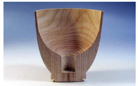
A form cut in half with the first two cut areas having been finished to thickness ready to move on to the next area
