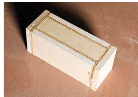
When making a mould, make sure all of the relevant joints are bonded together with no leaks
