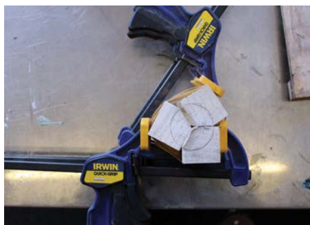
Clamping required for curing
