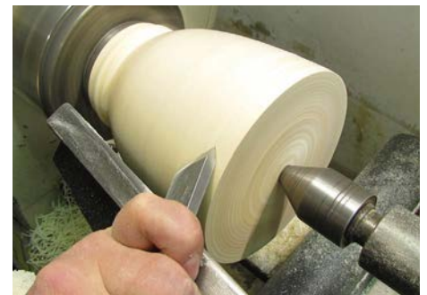
Refine the external shape with a gouge or skew
