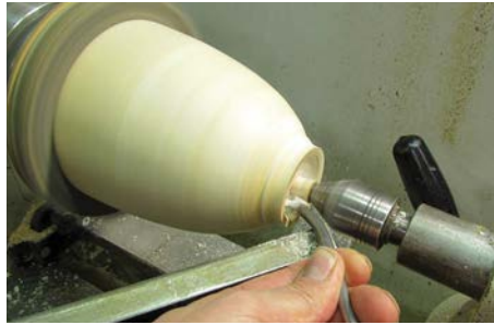
Refine the foot areas to leave an even wall thickness as much as practicable
