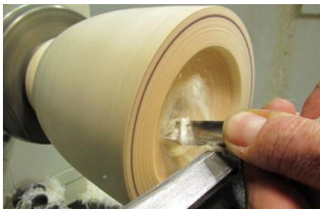
The gouge is arced from centre out towards the inner edge of the vessel, stopping just shy of the final thickness required
