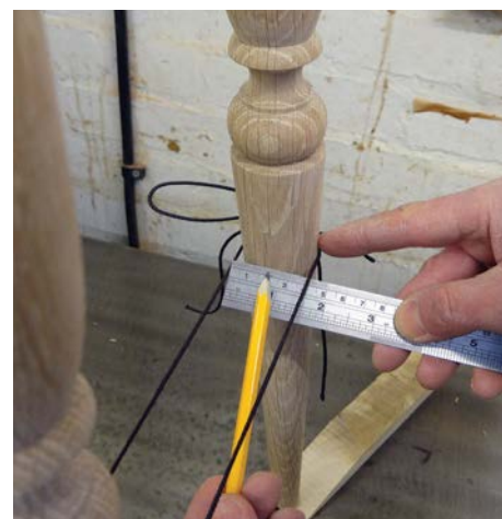
Using the loop of the cord to find the centre of the legs
