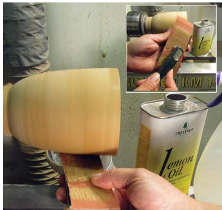
Wet sanding with water and a thin oil and cleaning up the abrasive
