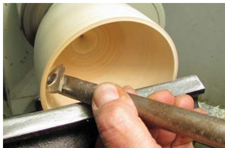
Using a scraper to blend in cut areas prior to moving on to the next area to be cut with a gouge
