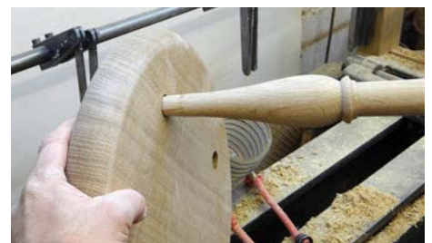
Test fitting the leg shows a witness mark
