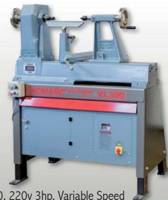
VL300, 220v 3hp, Variable Speed 24" swing. Adjustable height
