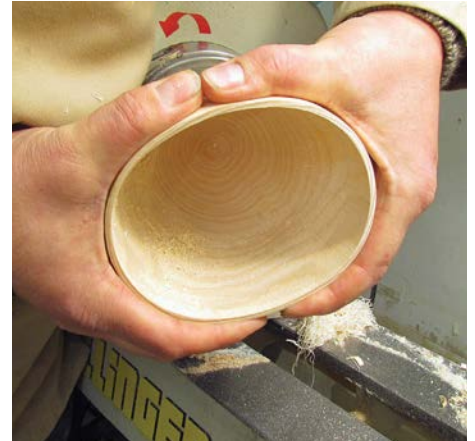
The wet wood fibres are flexible, as can be seen here with me crushing the wall of the form. It shows just how much the wood can move without fracture
