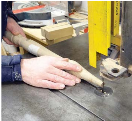
A bandsaw cut will give enough room for the wedge to be driven into the top of the leg
