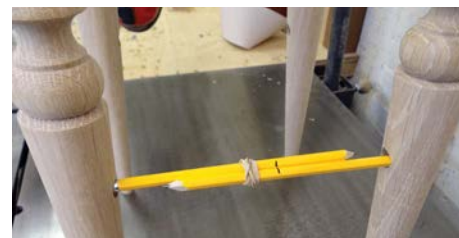
Using my pencil jig to measure the length of the stretchers
