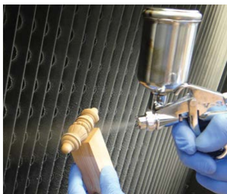
Spraying a layer of stain
