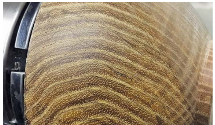
The result of the thin wired brass brush worked across the surface of the wood for 10 seconds with the lathe speed at 600rpm
