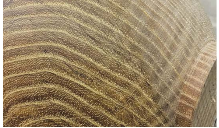
The result of the brush moved across the surface of the wood for 10 seconds with the lathe speed at 600rpm
