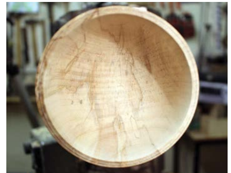
Finishing shear cut taken 24 hours later, leaving a clean surface
