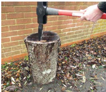
Using these cracks, a wedge is used in the log to split down through its length
