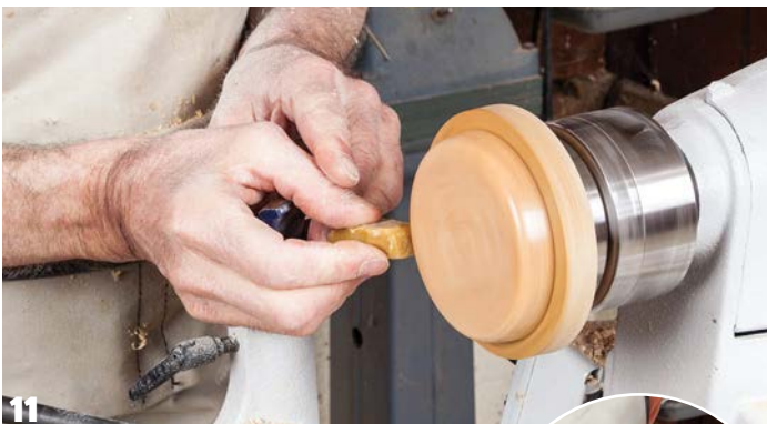
11 Buff with shavings or a small piece of paper towel. You can do all of this immediately. Now crayon on pure carnauba wax and buff with shavings again. Of course you can use a finish of your choice too. Pry the piece off the chuck with the bench chisel. Now fit the jar lid in the wooden lid's recess and, if required, apply a small amount of adhesive – silicone, cyanoacrylate or similar – to secure it in place
