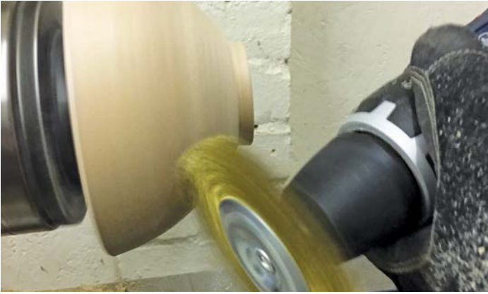
The coarse brass-coated wire brush being used in a drill against ash with the rotation of the brush running anti-clockwise
