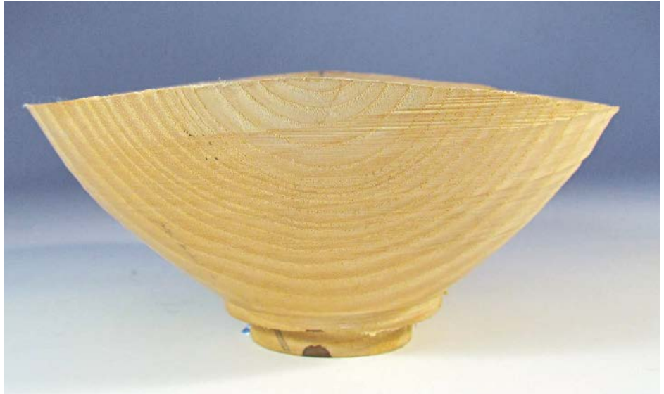
Roughed-out ash ( Fraxinus spp.) bowl showing how it has been cut – the centre area of the tree is uppermost – and how the wood has moved as it dries
