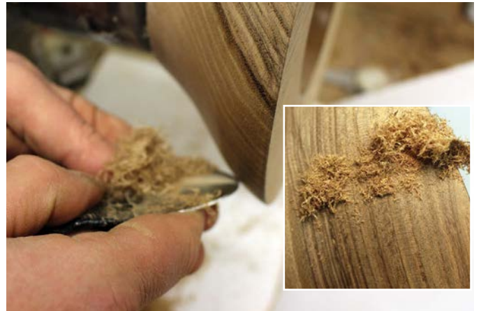
The scraper in use and the resulting shavings
