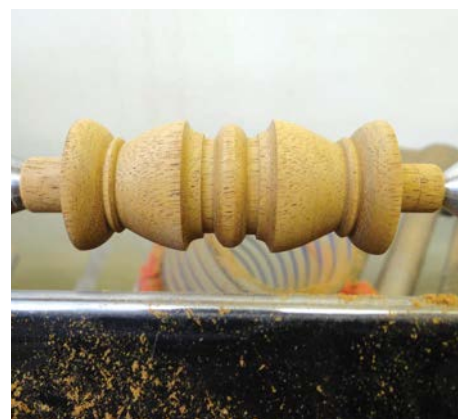
The turned spindle ready for carving
