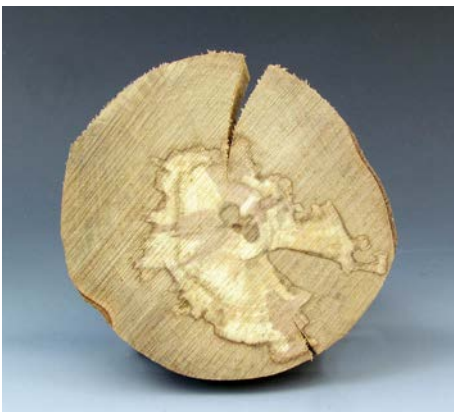
Cracking due to internal stresses created by uneven drying
