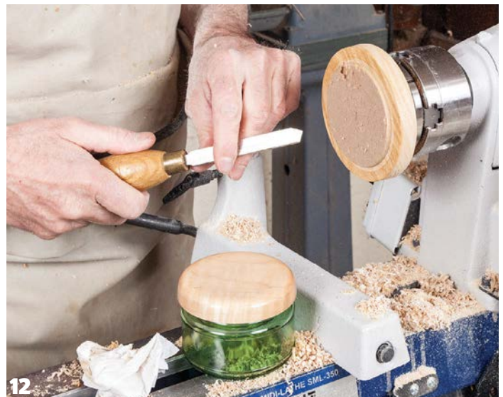
10 Sand the lid then apply some mineral oil to bring out the grain. Now brush on pure shellac
