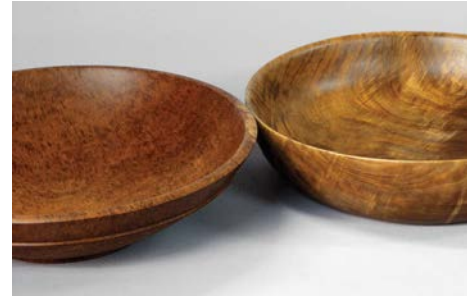
The way a simple highlight false on the inside of a bowl reveals the smoothness of the curve and thickness of the base, also gauged in relation to the surface the bowl sits on. On the walnut ( Juglans spp.) bowl (right), the highlight on the steep wall stops abruptly where the flat base meets the wall. On the gently curved inside of the lace sheoak ( Allocasuarina spp.), the highlight fades gradually towards the centre
