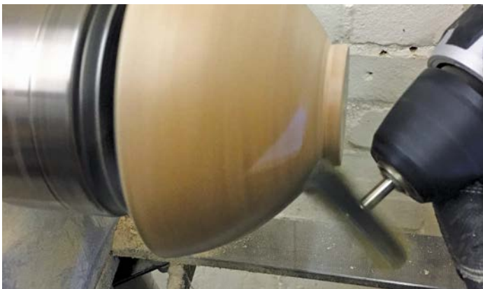
The thin brass-wired brush being used against the same piece of ash
