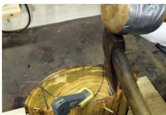
If you don't have a bandsaw a simple option is to clamp the blank as shown and, with a mallet and hatchet, cut down the line
