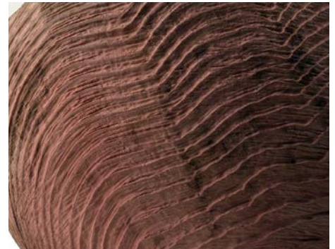
Here is a close-up of the texture on the exterior of the wellingtonia bowl. The timber is so soft that the softest areas were quickly removed with the coarser rotary wire brush, but note how that left some striations on the harder areas and some deep scoring on the softer areas. What you see here is much more refined than when the first steel wire brush was used. It is a similar effect to sandblasting
