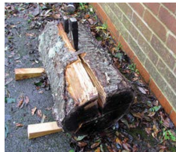
Turning it on to its side and supporting with wood wedges to stop it rolling, I then work along the splits
