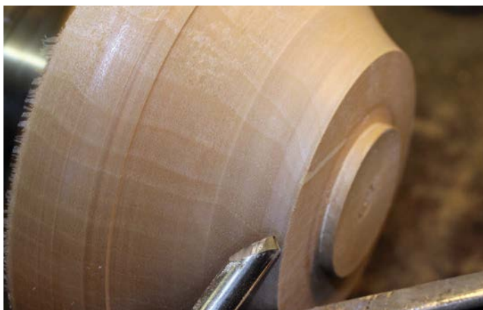
Pull shear cutting on a bowl's surface
