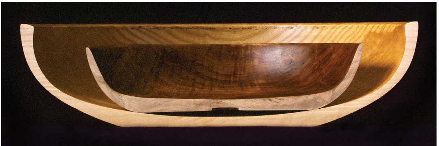
All is revealed in the cross-sections of these good – lower bowl made in ash ( Fraxinus spp., – and bad – upper bowl made in walnut ( Juglans spp.) archetypal bowls
