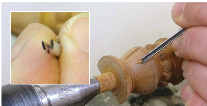
Cutting the flutes with the veiner
