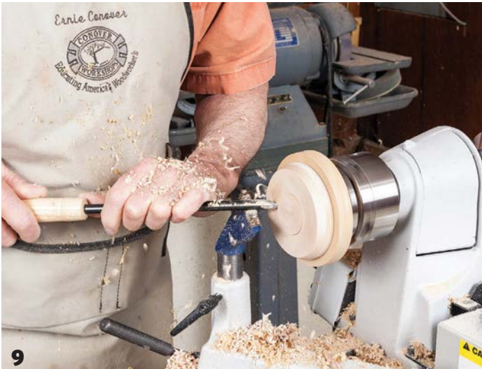
9 Turn the outside of your lid to a pleasing shape
