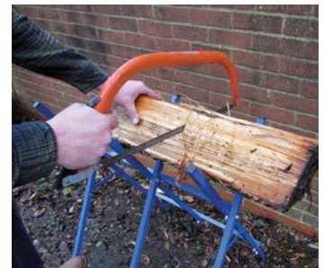
Next the sections are cut to a more manageable length on a sawhorse with bowsaw. You can use these sections for spindle grain or bowl-grain oriented blanks
