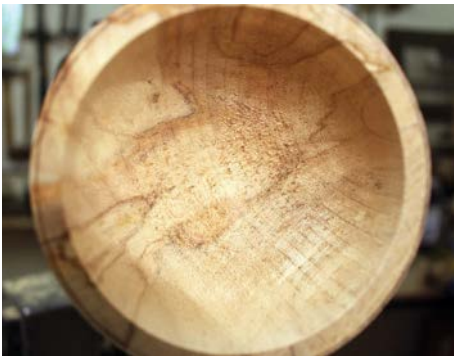
Badly torn grain in spalted wood
