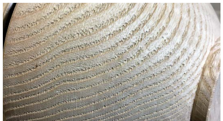
The result of the steel-wired cup brush used edge-on and moved across the surface of the wood for 10 seconds with the lathe speed at 600rpm.
