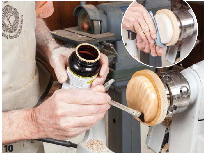
10 Sand the lid then apply some mineral oil to bring out the grain. Now brush on pure shellac
