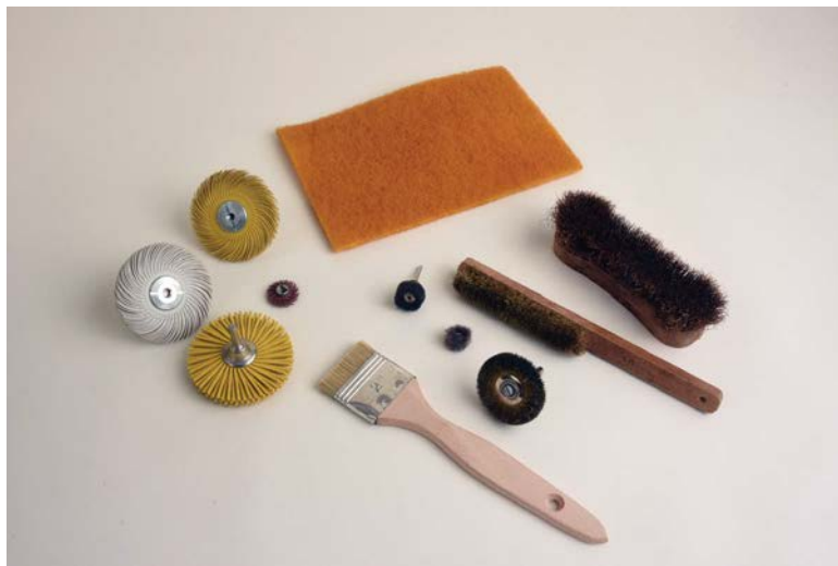
An assortment of items that can be used to refine a wire-brushed surface
