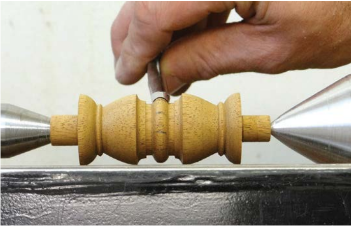
The curve of the gouge closely matches the shape of the bead
