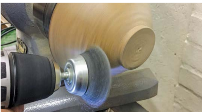
The steel wire cup brush being used against the same piece of ash
