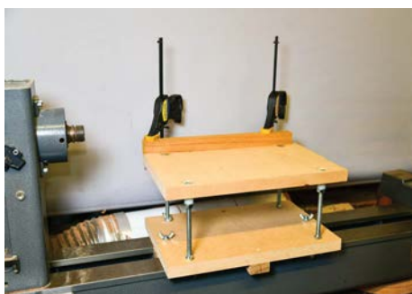
You can drill both spindle and faceplate projects using this jig, but do clamp things in place for safety
