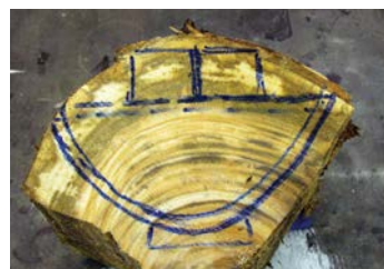
Flat-rim bowl. Note: you will also get a couple of spindle blanks from this section
