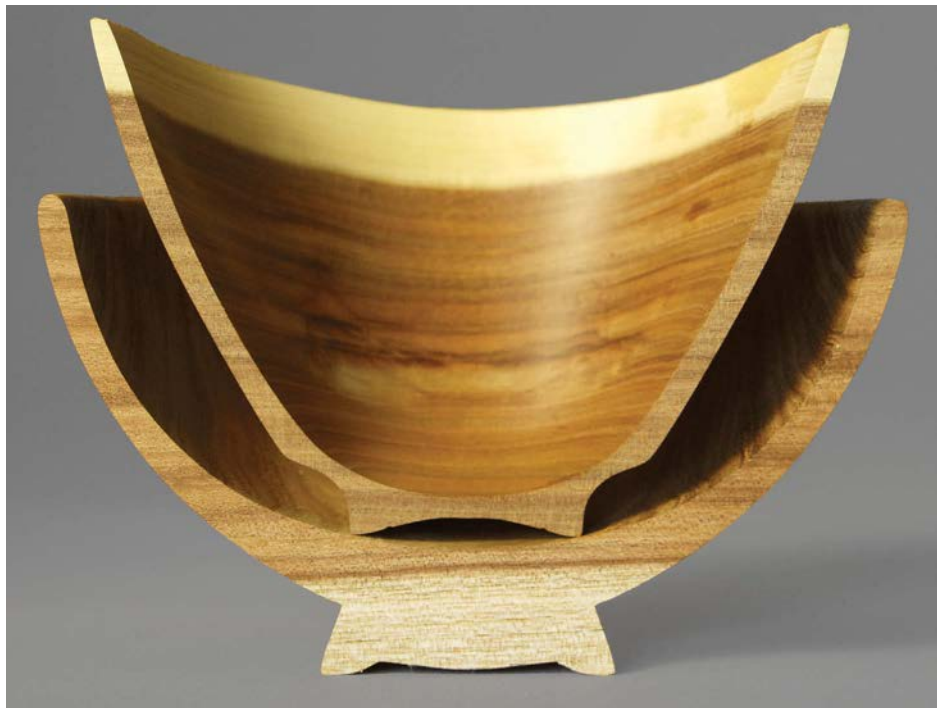
Although moderately chunky, the lower bowl feels better and is better balanced than the one above, where the wall is more even and the whole lighter in weight
