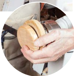
11 Buff with shavings or a small piece of paper towel. You can do all of this immediately. Now crayon on pure carnauba wax and buff with shavings again. Of course you can use a finish of your choice too. Pry the piece off the chuck with the bench chisel. Now fit the jar lid in the wooden lid's recess and, if required, apply a small amount of adhesive – silicone, cyanoacrylate or similar – to secure it in place
