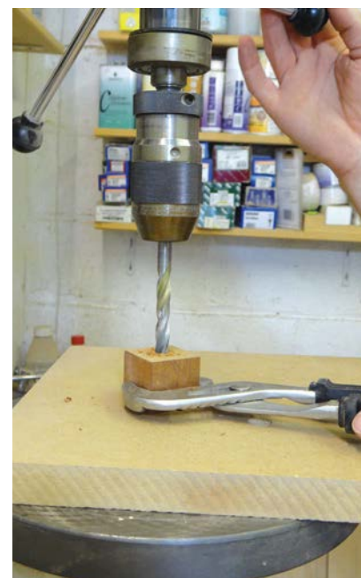
Drilling the mortises, holding the work with grips
