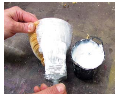
Paint the end grain of blanks with PVA glue, so they dry more evenly without cracking
