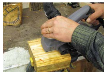
Once complete, the blank is clamped into a vice and an electric hand plane used to flatten the face. Note use of the quick-release clamp to hold larger sections
