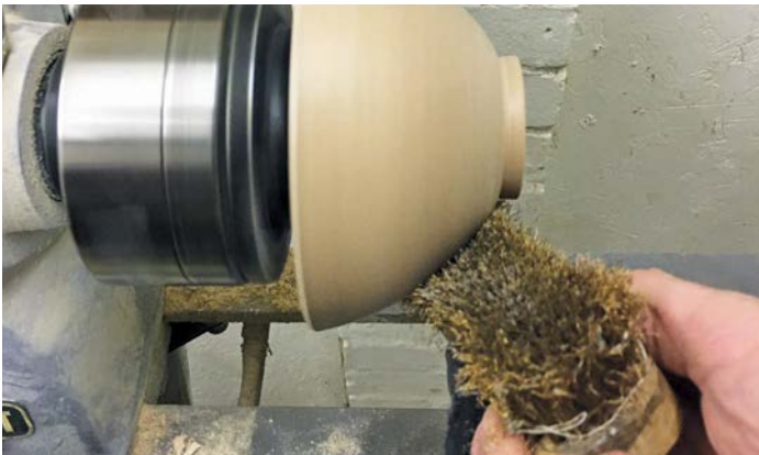
The bronze hand brush being used against the same piece of ash
