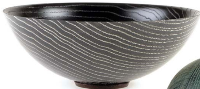
This bowl made from ash was turned, sanded, wire-brushed with a long-wired bronze brush to open up the grain and then sealed with sanding sealer, prior to spraying with black lacquer. It was denibbed and then had gilt cream applied and buffed to leave only the opened grain filled. Note the absence of any scratch marks from the wire brush. If any are left from the brush or the sanding, the gilt cream will highlight them
