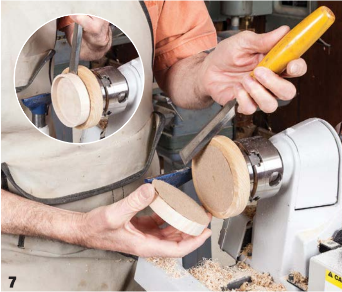
7 Remove the piece from the glue block with a bench chisel in the paper joint
