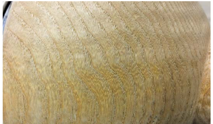
The result of the bronze brush moved across the surface of the wood for 10 seconds with the lathe speed at 600rpm
