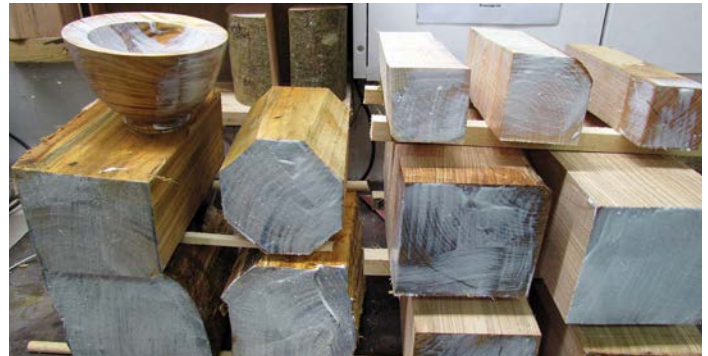
Sealed blanks with sticks to allow airflow during the drying process
