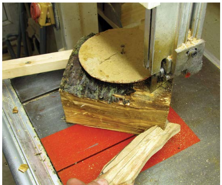
You can now continue by cutting off the corners with a handsaw, but here the bandsaw comes into its own for further processing to cut the corners off to produce an octagon. Cutting tight circles on a bandsaw can wear one side of the blade set, making it difficult to cut accurate straight sections
