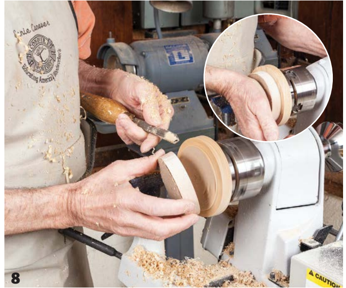
8 Scrape a tapered tenon on the glue block that matches the mortise/recess opening in the lid. Force it over the tenon with a smart smack. You need a secure hold but not so tight that it splits the sidewall as you do so
