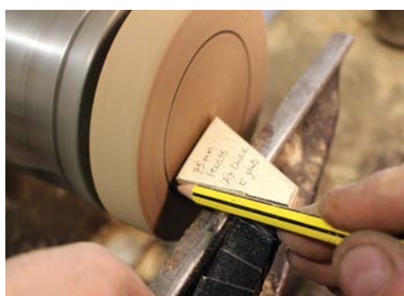
Marking a 75mm recess
